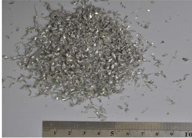
Figure 44. Chip forms of AZ91/2.5 wt.% rCF composite at conditions:  $V_c$ :560 m/min,
