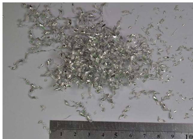
Figure 40. Chip forms of AZ91 alloy at conditions:  $V_c$ :480 m/min,  $V_f$ :0.65 mm/min
