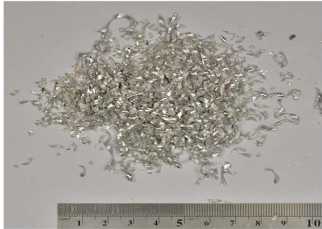
Figure 45. Chip forms of AZ91/2.5 wt.% rCF composite at conditions:  $V_c$ :640 m/min,
