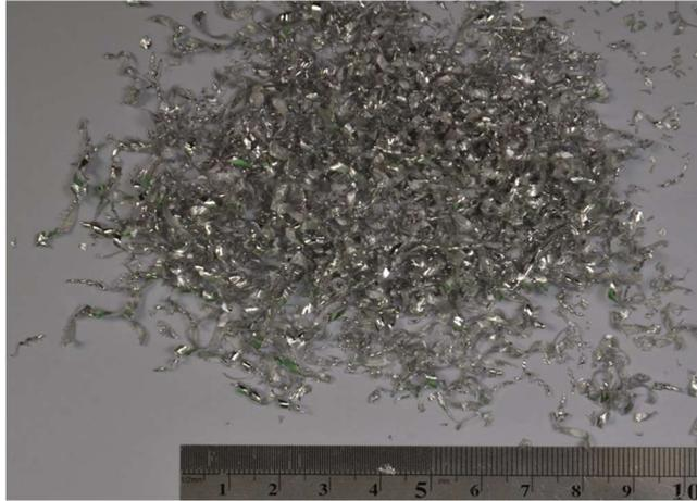
Figure 41. Chip forms of AZ91 alloy at conditions:  $V_c$ :560 m/min,  $V_f$ :0.80 mm/min
