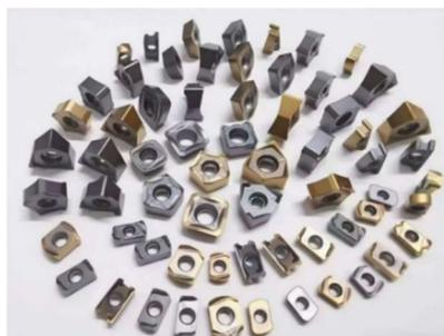
Figure 12. Types of face milling inserts<sup>47</sup>
