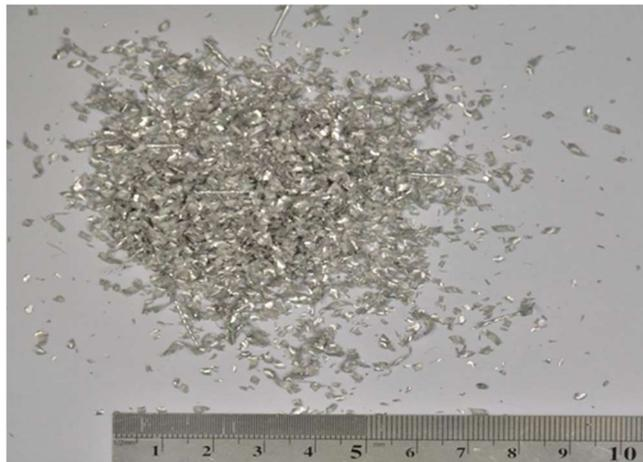
Figure 48. Chip forms of AZ91/5 wt.% rCF composite at conditions:  $V_c$ :640 m/min,
