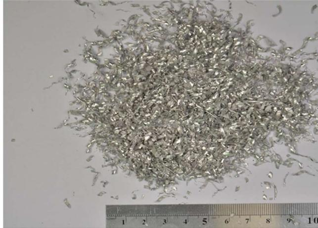
Figure 47. Chip forms of AZ91/5 wt.% rCF composite at conditions:  $V_c$ :560 m/min,
