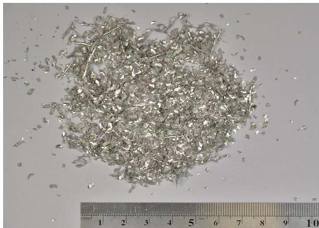
Figure 46. Chip forms of AZ91/5 wt.% rCF composite at conditions:  $V_c$ :480 m/min,
