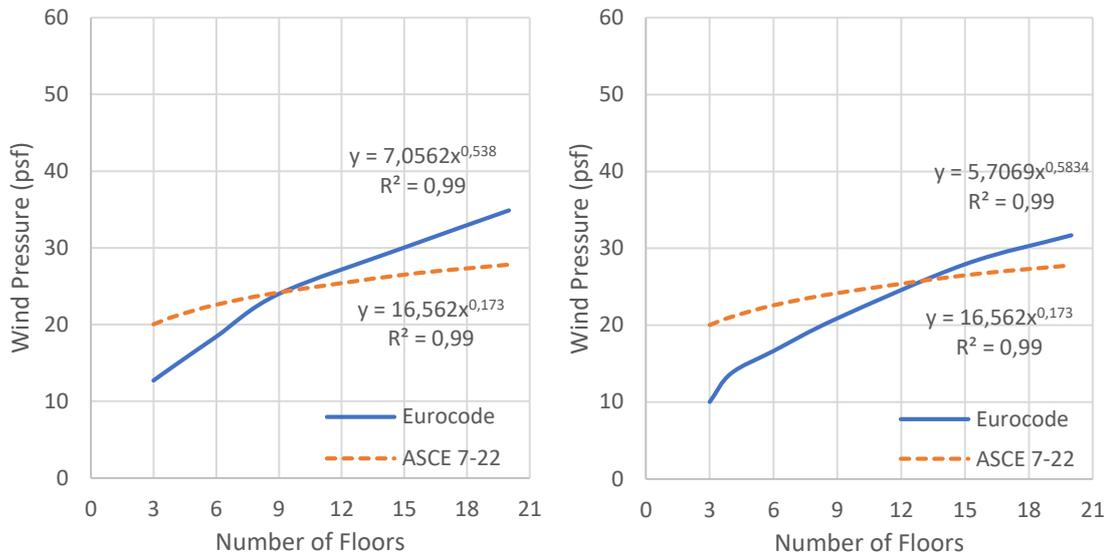
Figure 4.6. ASCE 7-22 -EN1991-1 Comparison for a) 2y b) 3y
