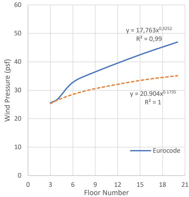
A.6. Wind Pressure- Number of Floors for Racetrack on Winward Wall (Directionality y)
