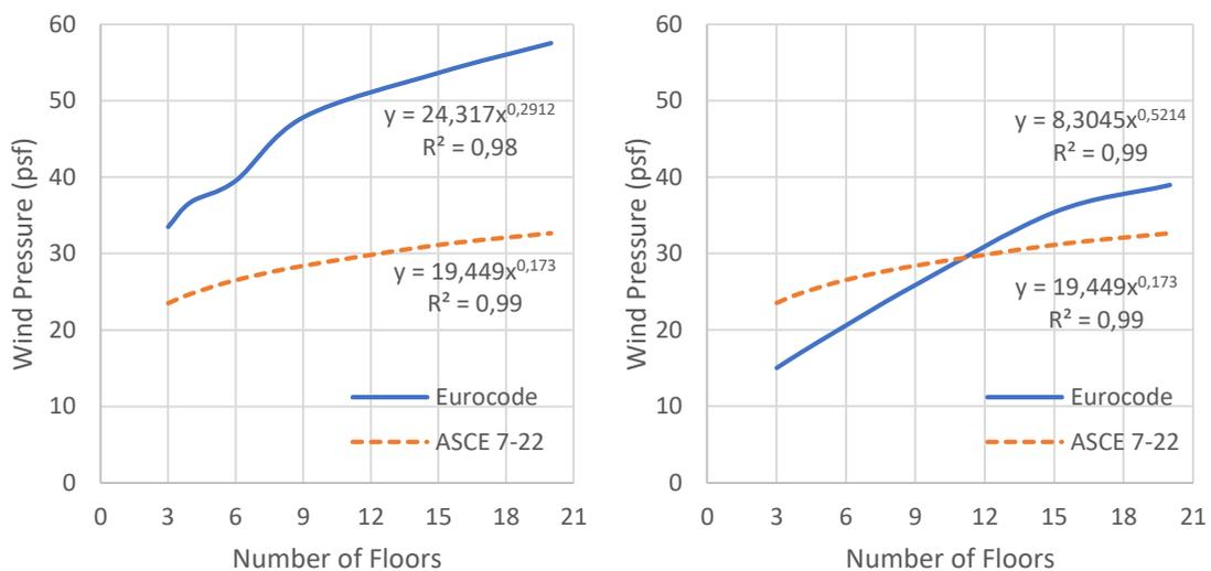
Figure 4.7. ASCE 7-22 -EN1991-1 Comparison for a) 1x b) 1y
