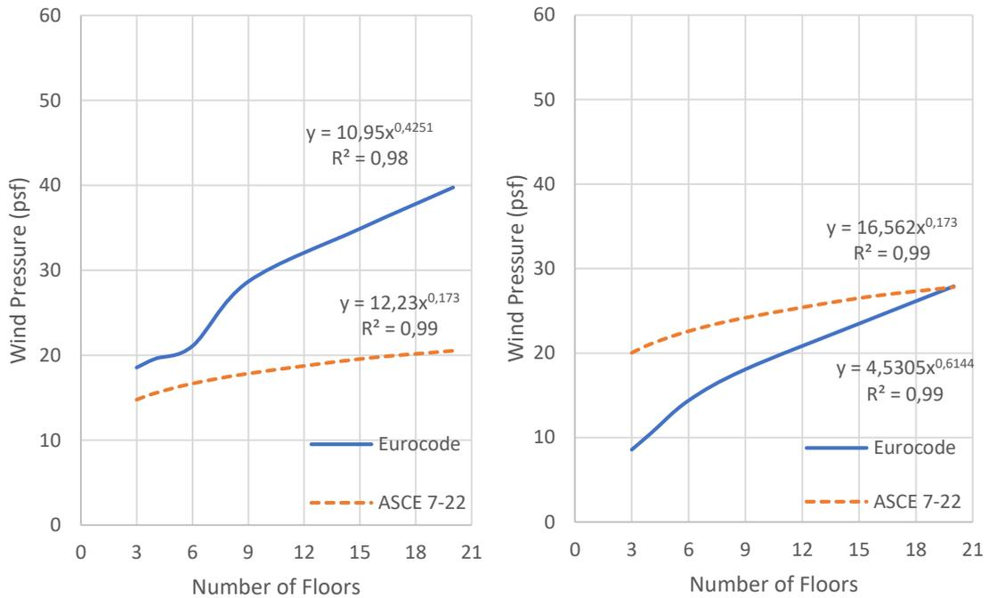
Figure 4.5. ASCE 7-22 -EN1991-1 Comparison for a) 1x b) 1y
