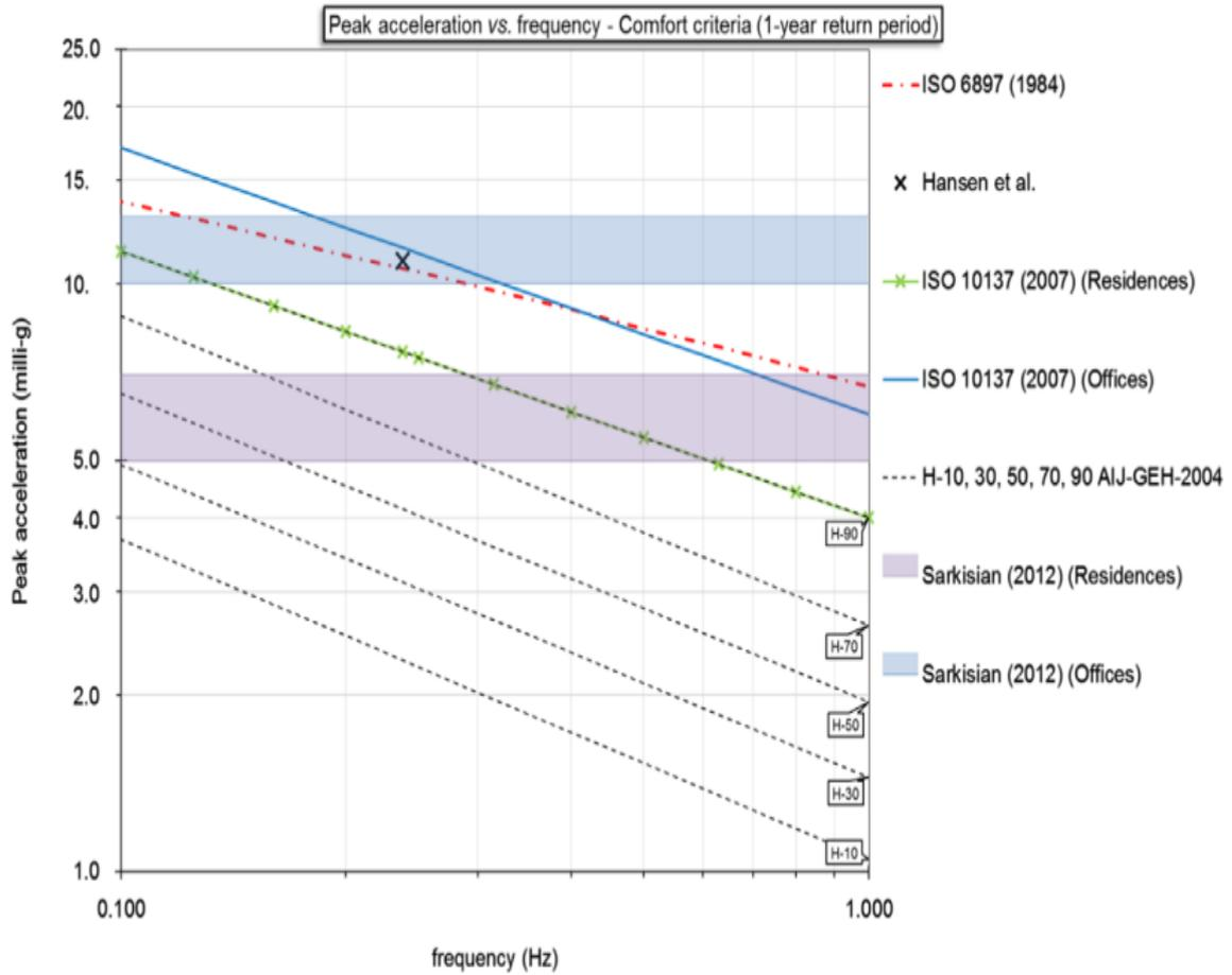
Figure 2.2. Peak Acceleration-Based Occupant Comfort Limits (Ferrareto et al. 2014)
