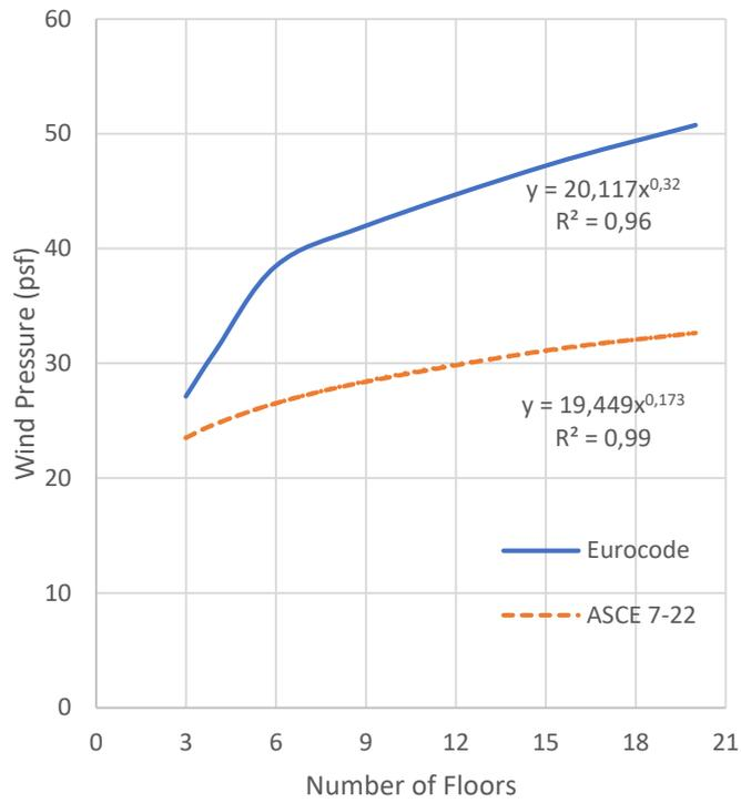
A.8. Side Wall Wind Pressures for Type 2 (Racetrack-Directionality y)
