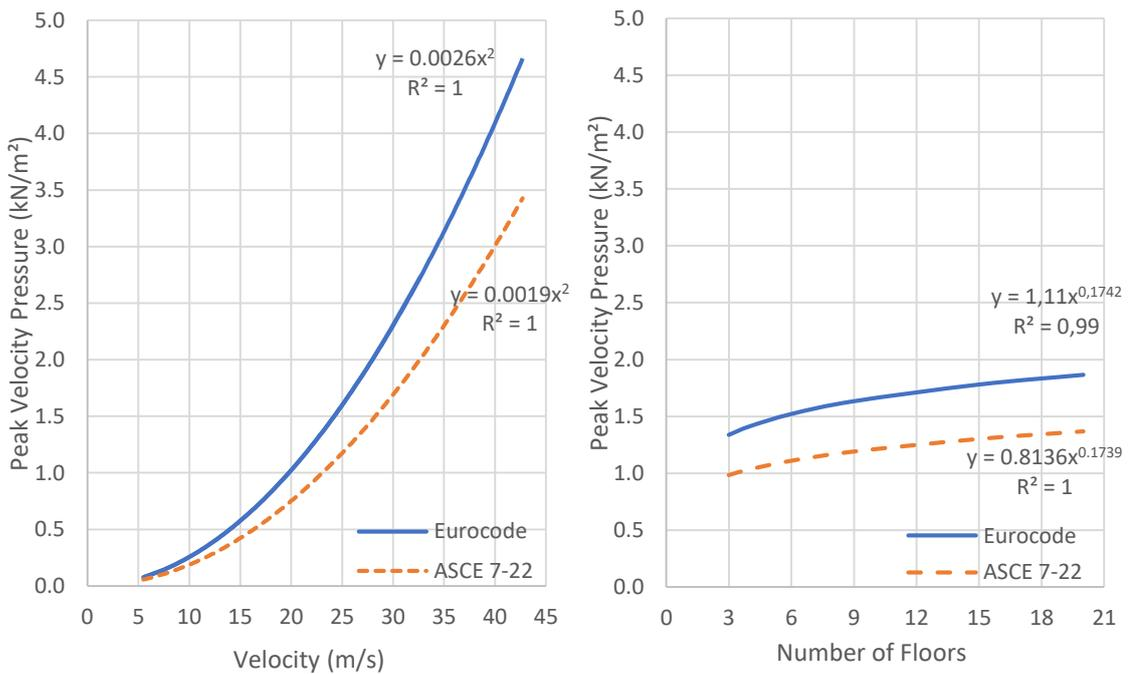
Figure 4.1. a) Peak Velocity Pressure-Velocity b) Peak Velocity Pressure-Number of Floors at  $V= 27$  m/s
