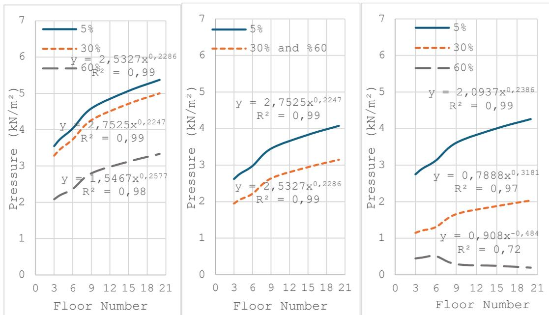
Figure 4.9. Number of Floor- Peak Velocity Pressure at Zone F for a) Mono Pitched Roof b) Duo Pitched Roof c) Hipped Roof
