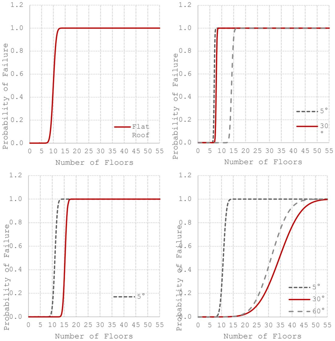
Figure 4.10. Roof fragility curves a) Flat Roof b) Monopitch roof b) Duopitch Roof c) Hipped Roof
