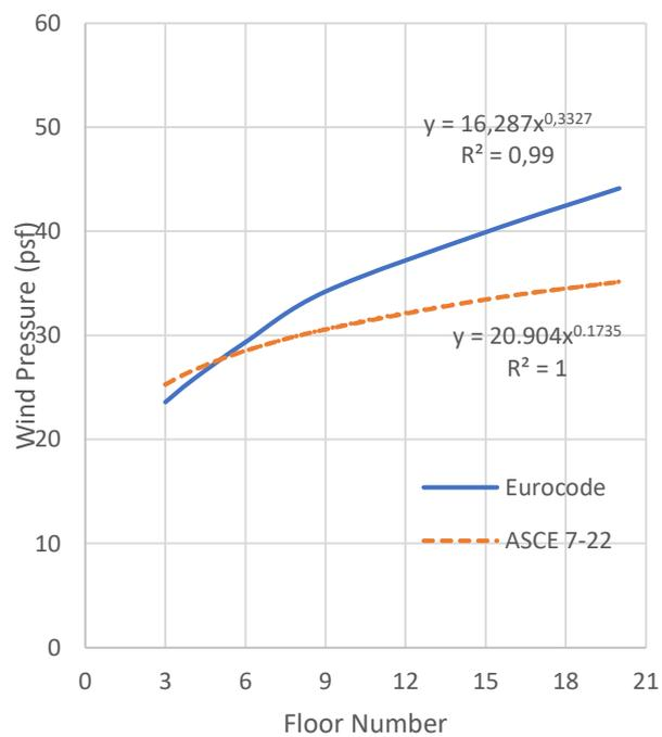
A.7. Side Wall Wind Pressures for Type 2 (Racetrack-Directionality x)
