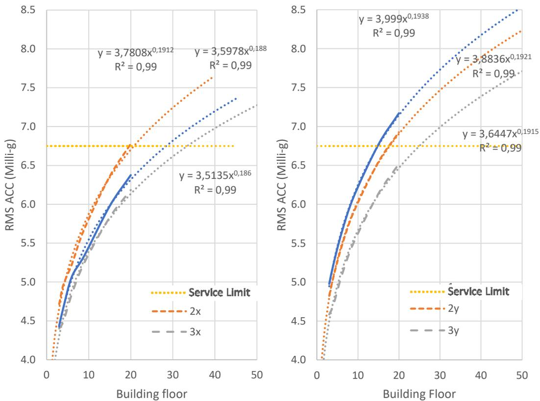
Figure 4.16. Floor Number- Geometry Comparison for EN1991-1 a) Directionality x
