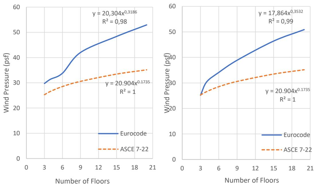
Figure 4. 3. Windward Wall Pressures for a) 1x b) 3x
