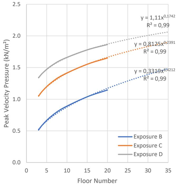
A.4. Peak Velocity Pressure-Number of Floors for ASCE 7-22 (V= 27 m/s)
