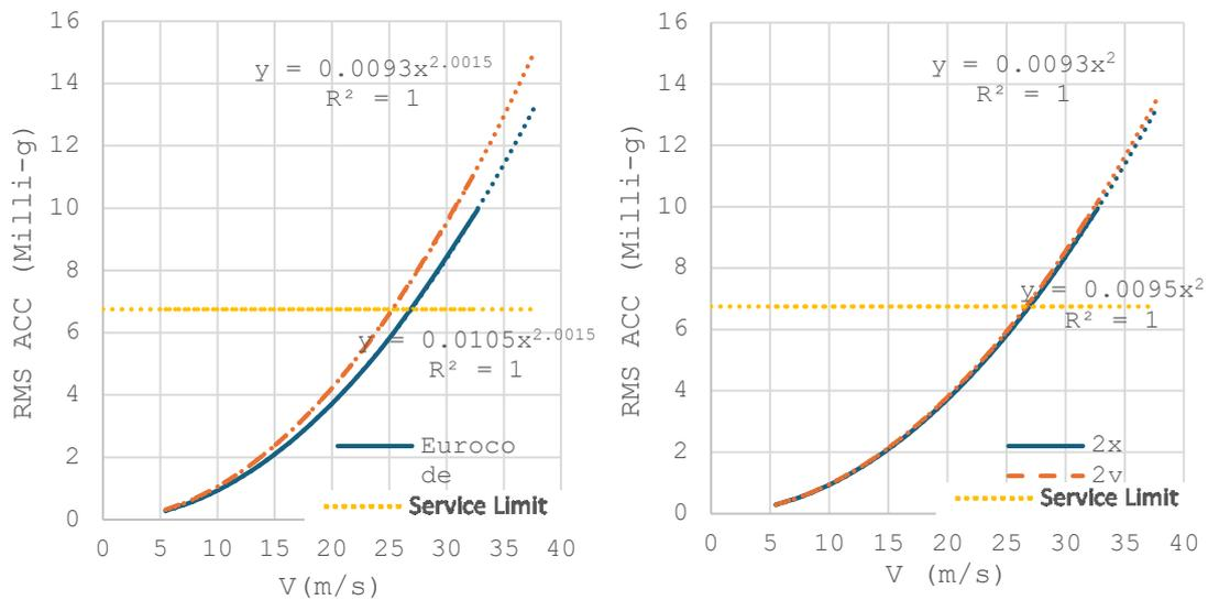
Figure 4.14. a) Velocity Based Code Comparison b) Velocity- Directionality Comparison for Type 2 (EN1991-1)
