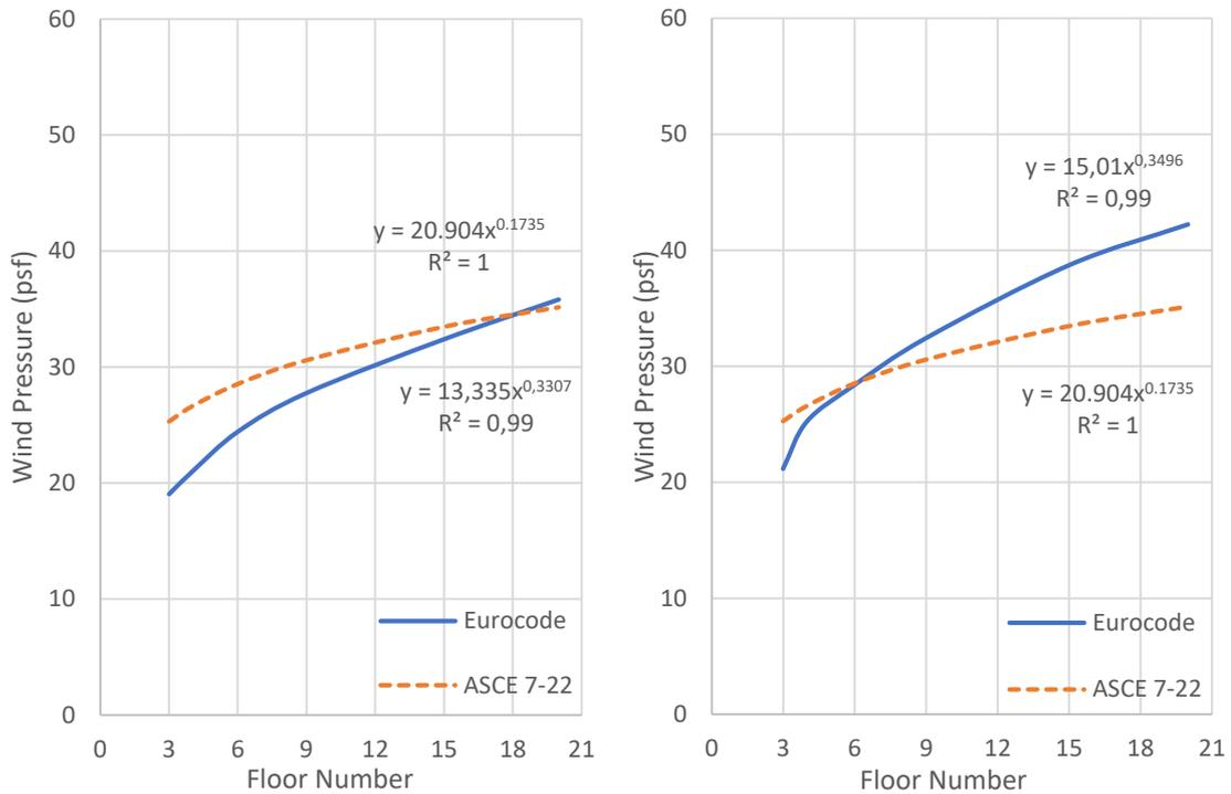
Figure 4.4. Windward Wall Pressures a) 1y b) 3y
