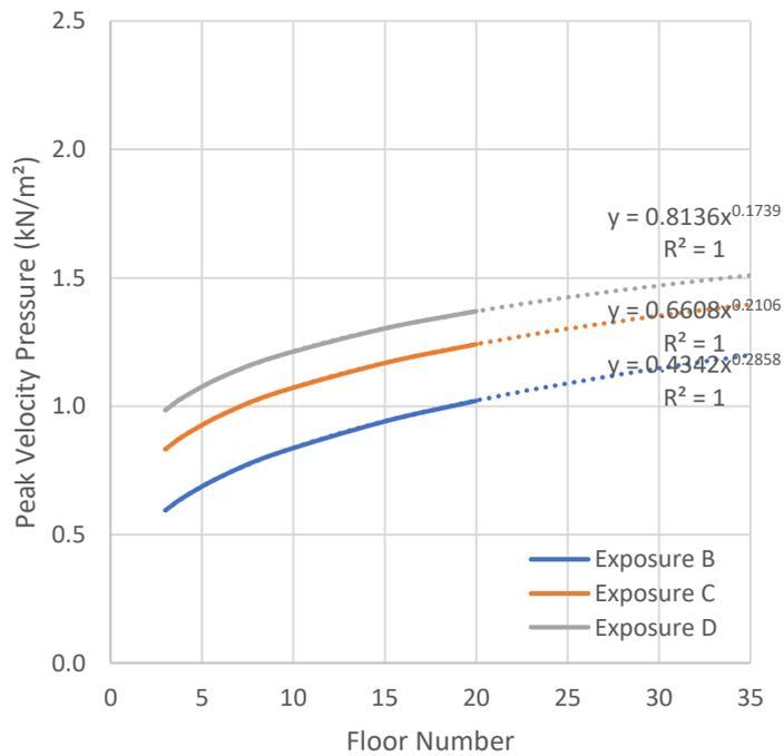
A.5. Wind Pressure- Number of Floors for Racetrack on Winward Wall (Directionality x)
