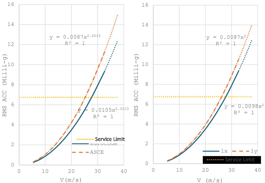
Figure 4.12. a) Velocity Based Code Comparison b) Velocity- Directionality Comparison for Type 1 (EN1991-1)
