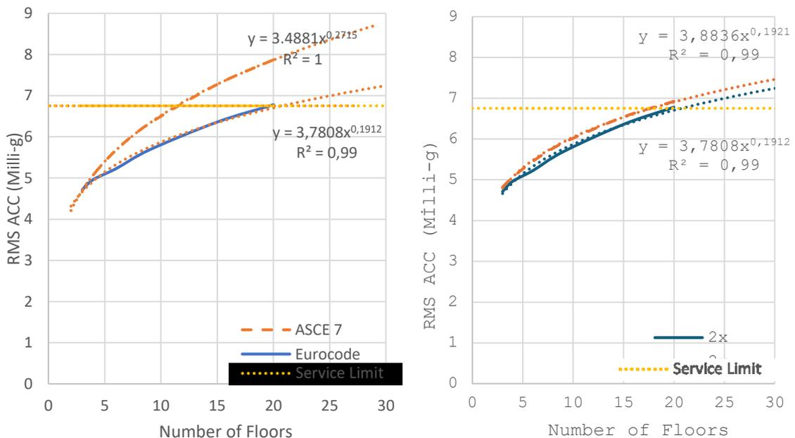
Figure 4.13. a) Floor Number-Based Code Comparison b) Velocity- Directionality Comparison for Type 2 (EN1991-1)
