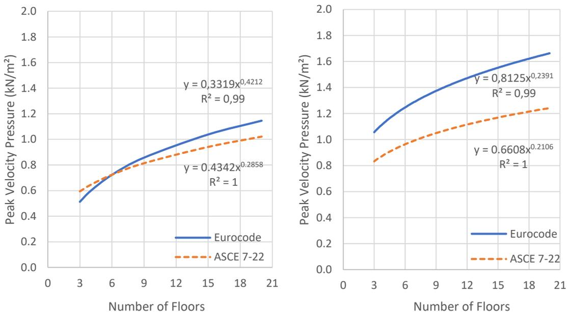
Figure 4.2. Peak Velocity Pressure Comparison for a) Exposure B, b) Exposure C
