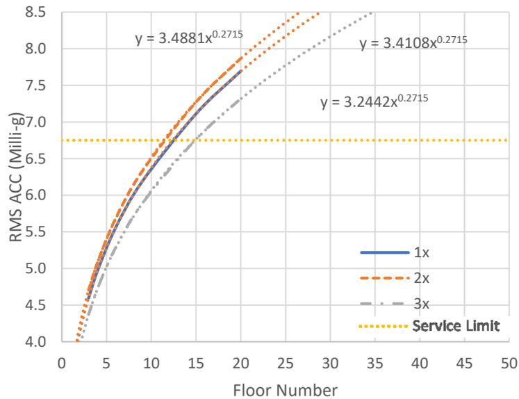
Figure 4.17. Floor Number Geometry Comparison for ASCE 7-22
