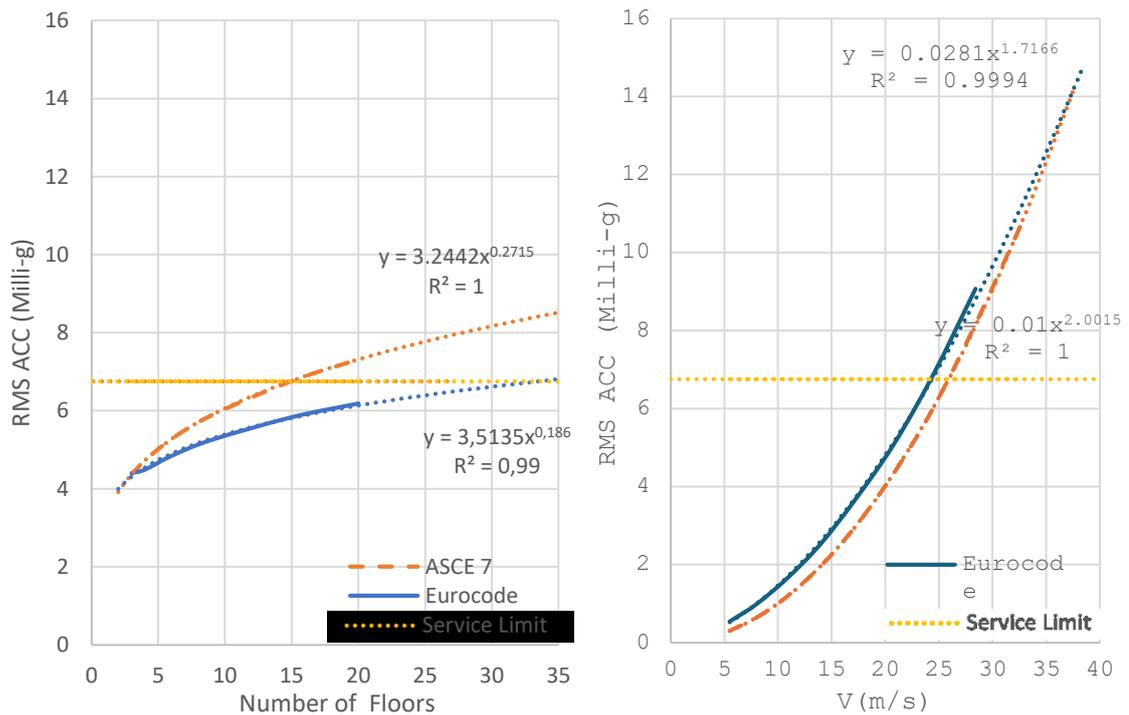
Figure 4.15. a) Floor Number-Based Code Comparison b) Velocity- Directionality Comparison for Type 3 (EN1991-1)
