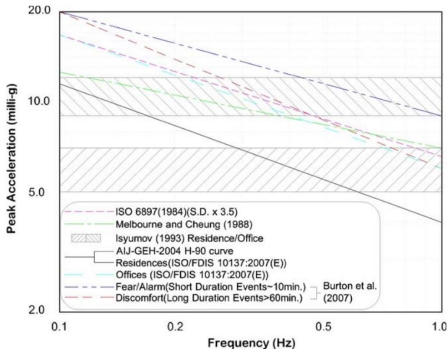
Figure 2.1. Criteria for Occupant Comfort and Serviceability Over a One-Year Return Period (Kwok, 2009)
