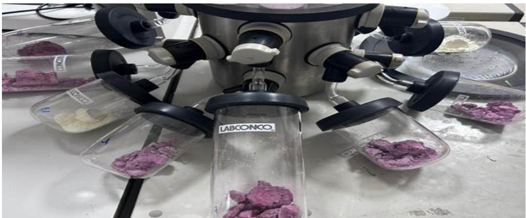
Figure 3. Samples lyophilized in a lyophilizer (Lablonco, USA)
