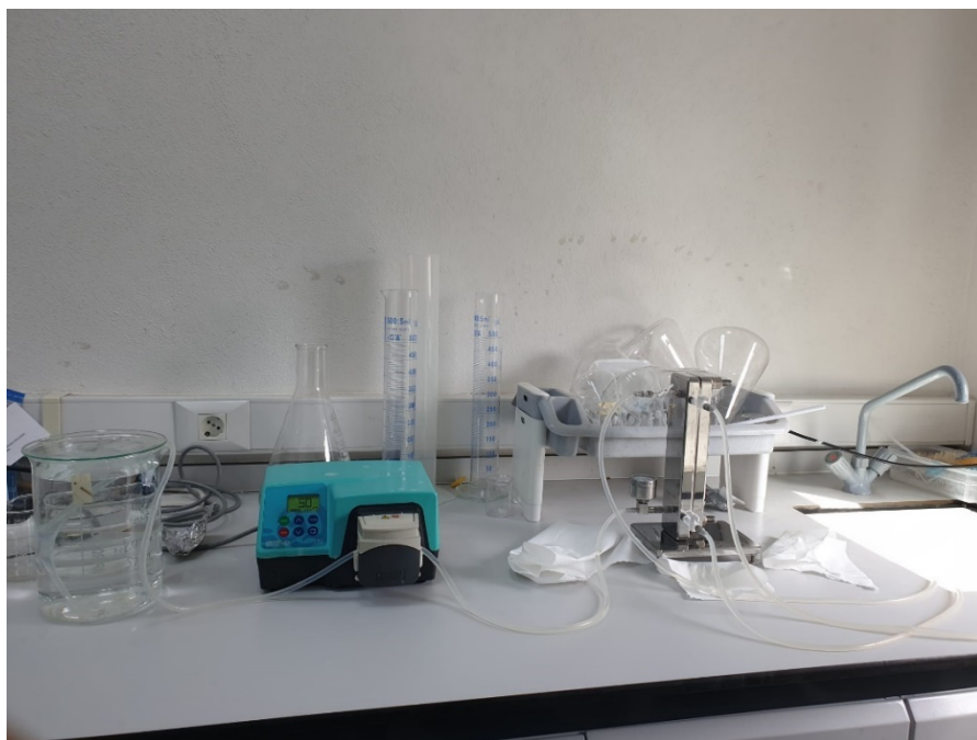
Figure B3. Ultrafiltration setup for Maillard reaction products
