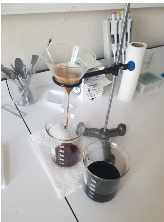
Figure B2. Maillard reaction products filtered with Whatman filter paper.
