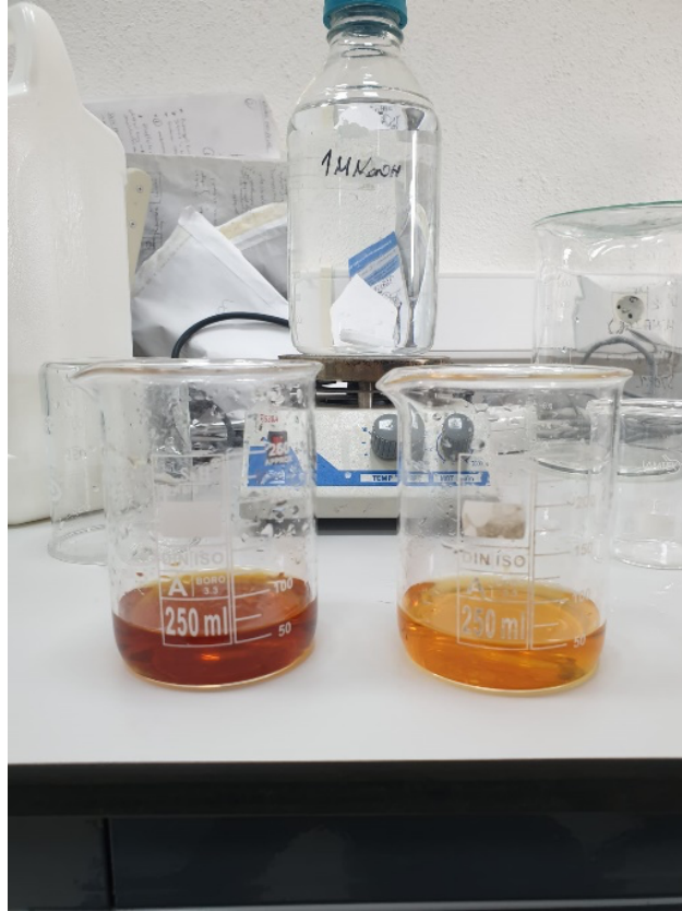
Figure C1. After ultrafiltration process of Maillard reaction products (Left: Retentate, Right: Permeate)
