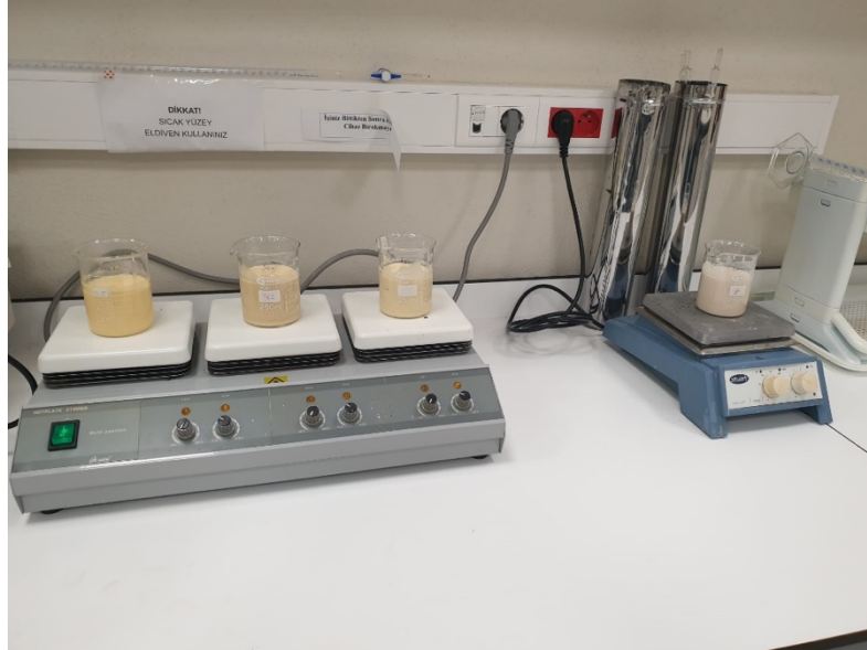
Figure A1. Lipid extraction from Legumes with n-Hexane
