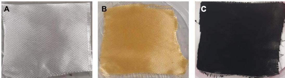
Figure 3.6 Preparation and CNT Growth on 10 cm x 10 cm GF Fabric: (A) Initial GF Fabric, (B) Dip-Coated with Fe Catalyst, (C) resulting CNT growth
