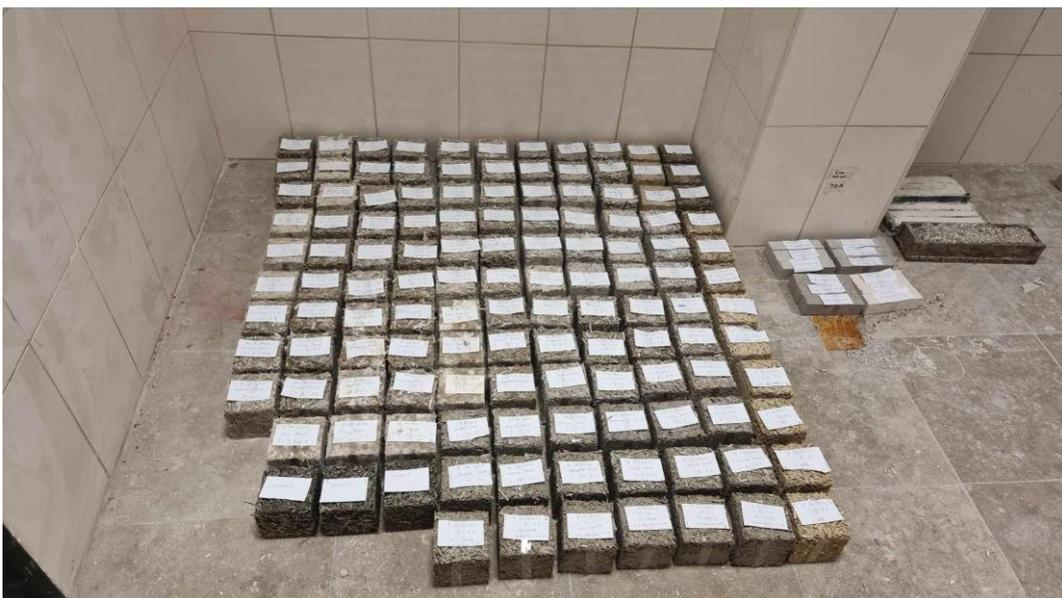
Figure 16. Hempcrete specimens in the curing room.
