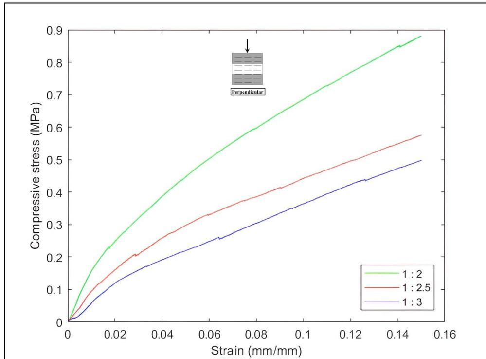
Figure 52. Effect of hemp : water on the compressive stress-strain relationship of hempcrete specimens loaded perpendicular to the hemp shives' orientation at 180 days.
