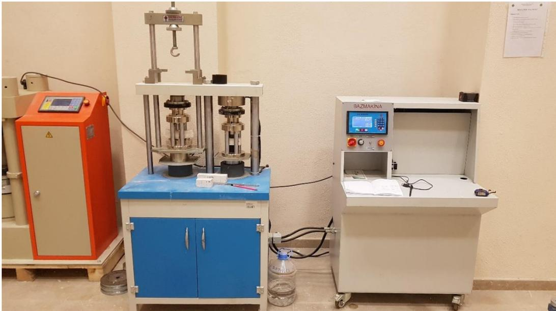
Figure 17. The testing machine used for evaluating the binder paste.
