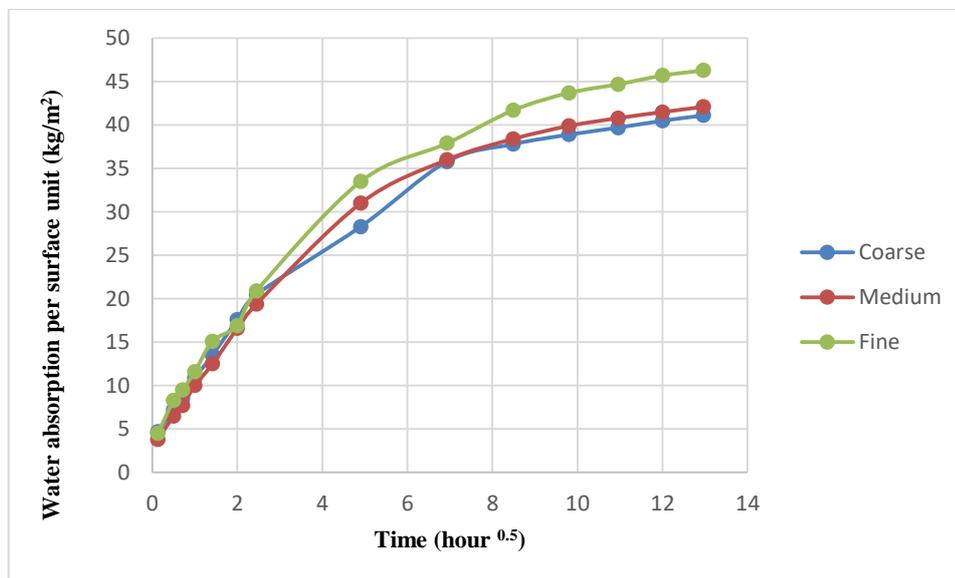
Figure 64. Effect of particle size on the capillary water absorption of hempcrete.
