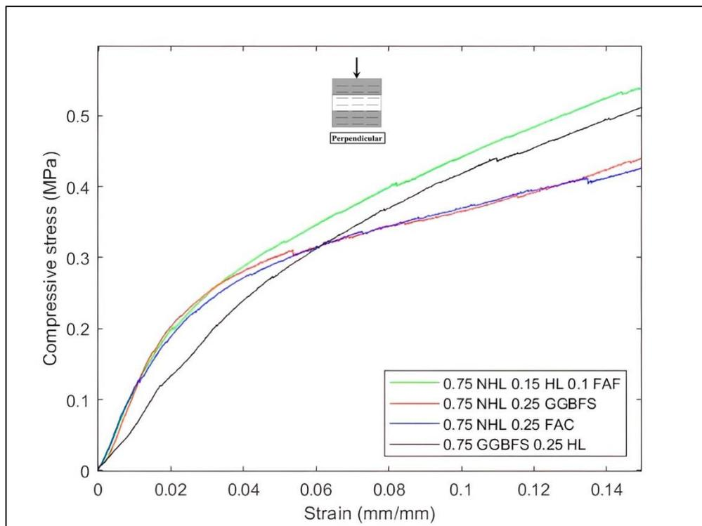
Figure 37. Effect of binder composition on the compressive stress-strain relationship of hempcrete specimens loaded perpendicular to the hemp shives' orientation at 28 days.
