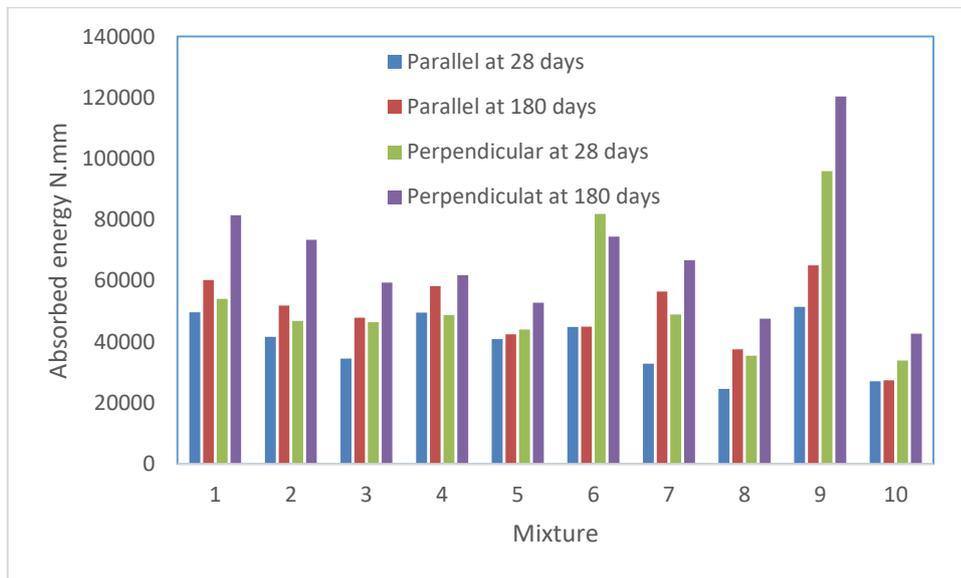
Figure 67. The absorbed energy of hempcrete specimens under compression at 28 and 180 days was evaluated in both parallel and perpendicular loading directions.
