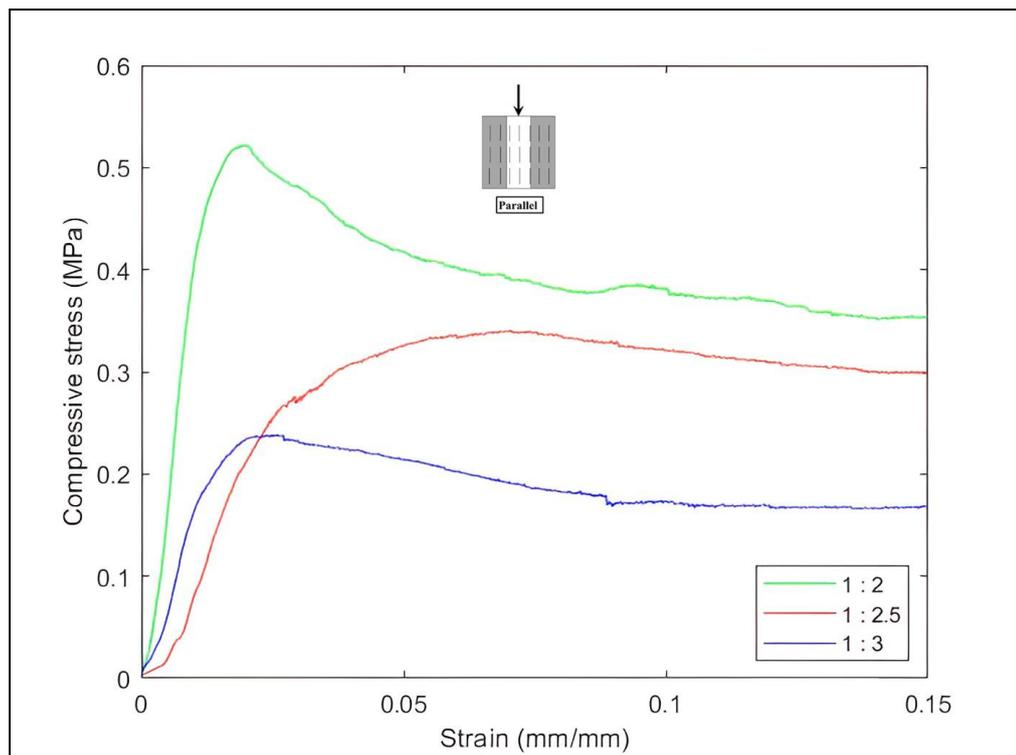
Figure 51. Effect of hemp : water ratio on the compressive stress-strain relationship of hempcrete specimens loaded parallel to the hemp shives' orientation at 180 days
