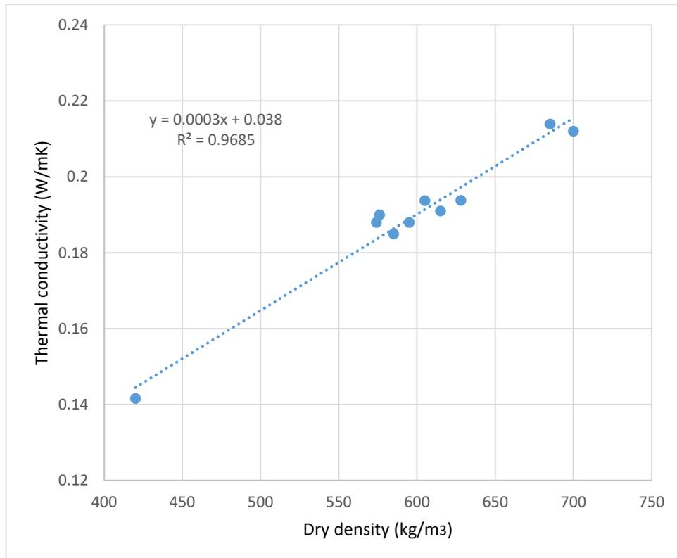
Figure 56. Thermal conductivity of hempcrete versus density.
