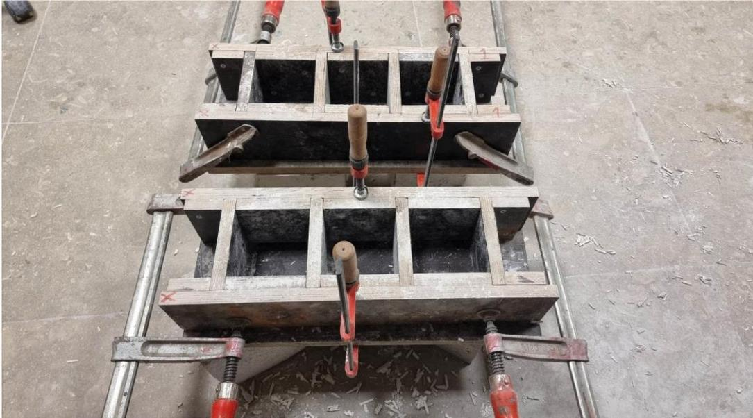
Figure 15. The molds used for casting hempcrete specimens.
