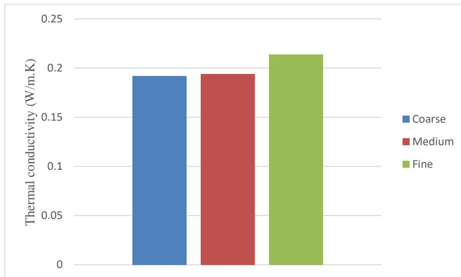
Figure 59. Effect of hemp shive particle size on the thermal conductivity of hempcrete.
