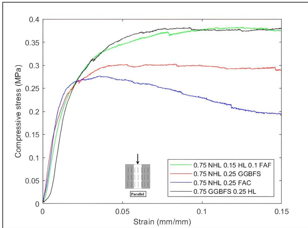
Figure 36. Effect of binder composition on the compressive stress-strain relationship of hempcrete specimens loaded parallel to the hemp shives' direction at 28 days.
