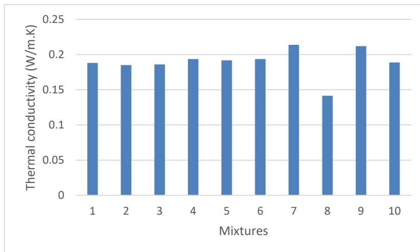
Figure 55. The thermal conductivity of hempcrete specimens.
