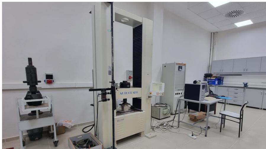
Figure 21. Compressive strength test of hempcrete specimens.
