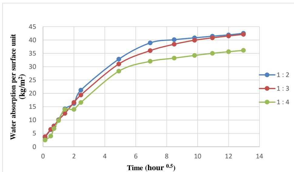
Figure 65. Effect of hemp : binder ratio on the capillary water absorption of hempcrete.
