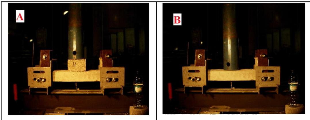
Figure 69. Impact test: A) with hempcrete and B) without hempcrete.
