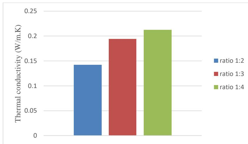
Figure 60. Effect of hemp : binder ratio on the thermal conductivity of hempcrete.
