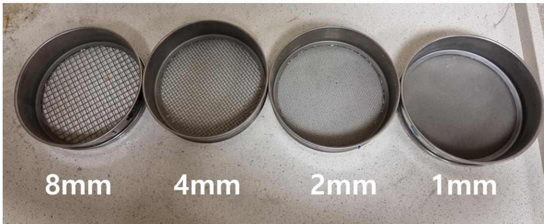
Figure 13. The sieves used in the research.
