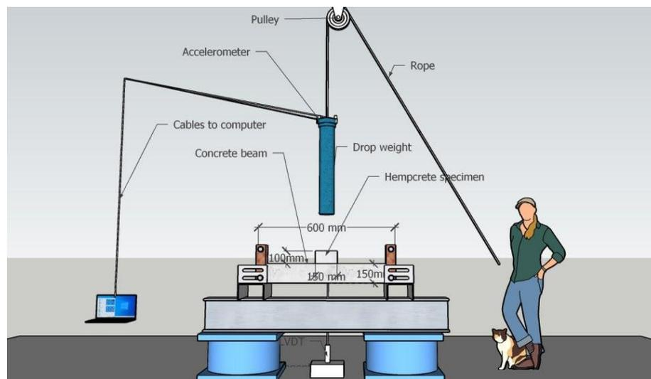
Figure 26. Illustration of the impact test.
