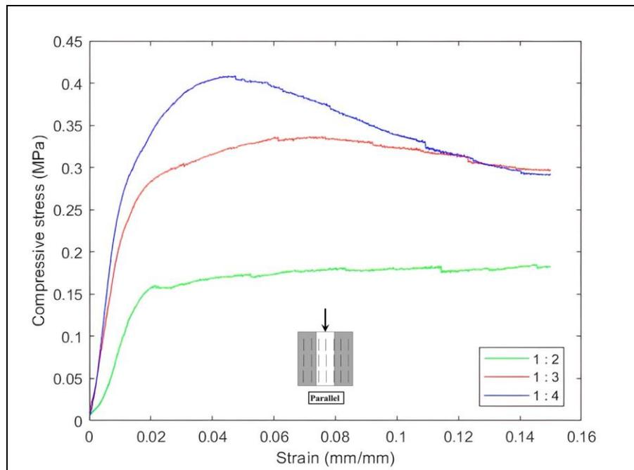
Figure 40. Effect of hemp : binder on the compressive stress-strain relationship of hempcrete specimens loaded parallel to the hemp shives' orientation at 28 days.
