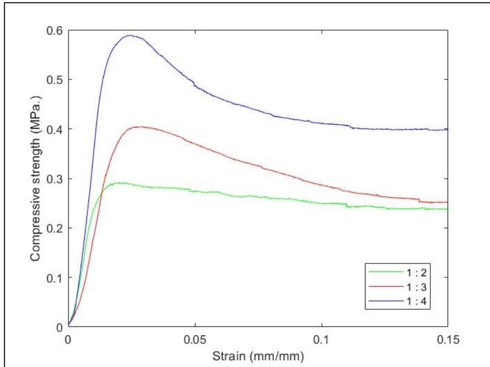
Figure 49. Effect of hemp : binder ratio on the compressive stress-strain relationship of hempcrete specimens loaded parallel to the hemp shives' orientation at 180 days.
