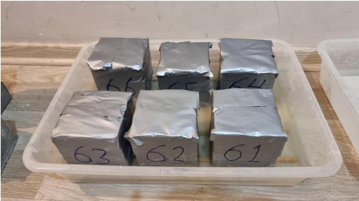
Figure 24. Capillary water absorption of hempcrete specimens.
