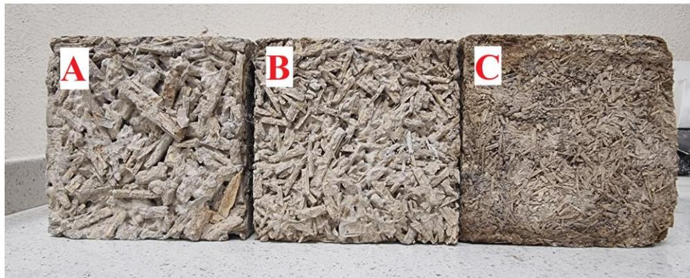
Figure 33. Hempcrete specimens with three distinct particle sizes: A) Coarse, B) Medium, C) Fine.
