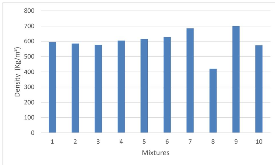
Figure 32. The density of the mixtures in the research.
