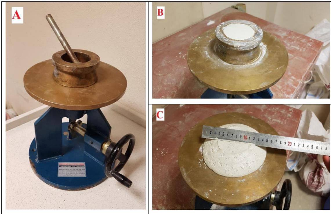
Figure 12. Flow table test: A) Flow table, B) Filling the mold with binder, C) Measuring the flow.
