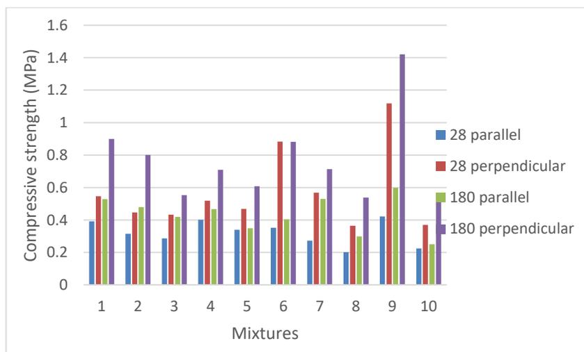
Figure 34. Compressive strength of hempcrete mixtures at 28 and 180 days in parallel and perpendicular directions to the hemp shiv orientation.
