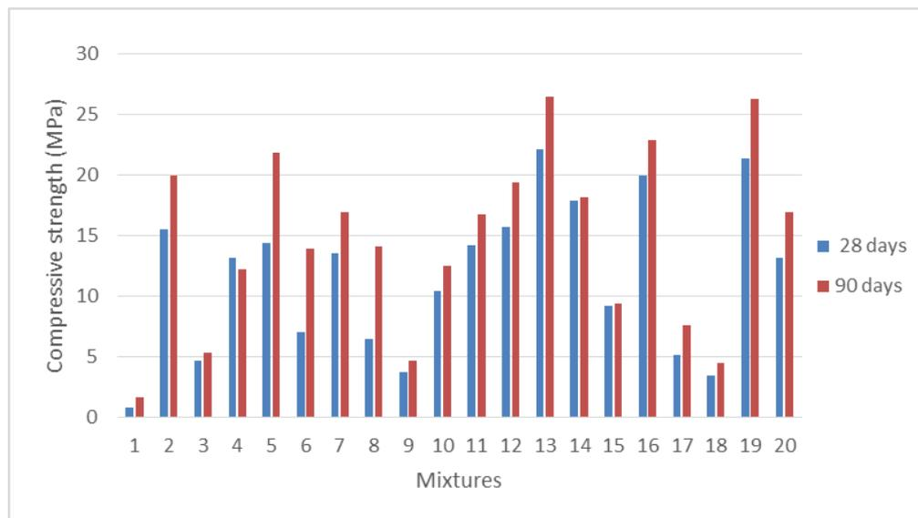
Figure 28. Compressive strength of binder pastes at 28 and 90 days.
