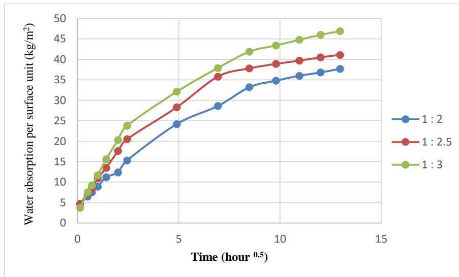
Figure 66. Effect of hemp : water ratio on the capillary water absorption of hempcrete.
