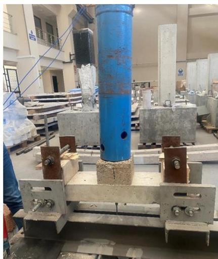
Figure 68. An experimental setup was used to investigate the impact behavior of hempcrete.
