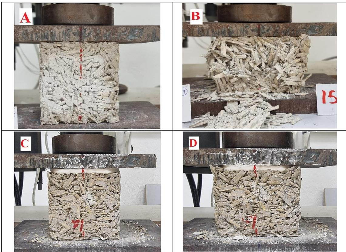
Figure 54. Comparison of the failure of Mix 1 at a strain of 15% : A) Before testing B) After testing parallel to the hemp shiv orientation C) Before testing D) After testing perpendicular to the hemp shiv orientation.
