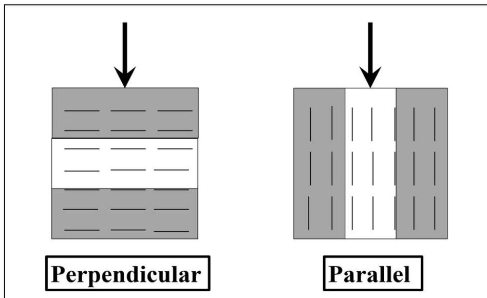
Figure 22. Application of load parallel and perpendicular to the hemp shives' orientation.
