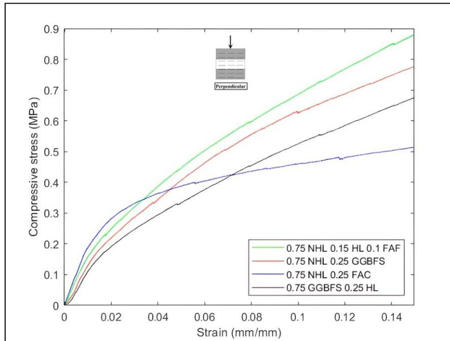
Figure 46. Effect of binder composition on the compressive stress-strain relationship of hempcrete specimens loaded perpendicular to the hemp shives' orientation at 180 days.
