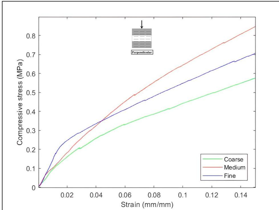
Figure 48. Effect of particle size on the compressive stress-strain relationship of hempcrete specimens loaded perpendicular to the hemp shives' orientation at 180 days.
