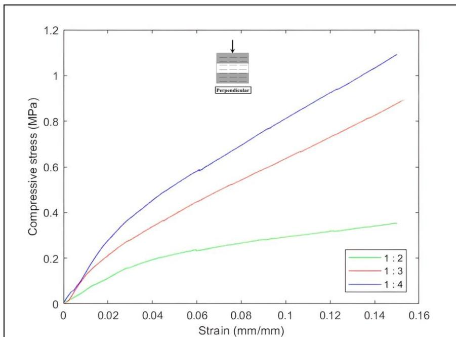
Figure 41. Effect of hemp : binder ratio on the compressive stress-strain relationship of hempcrete specimens loaded perpendicular to the hemp shives' orientation at 28 days.
