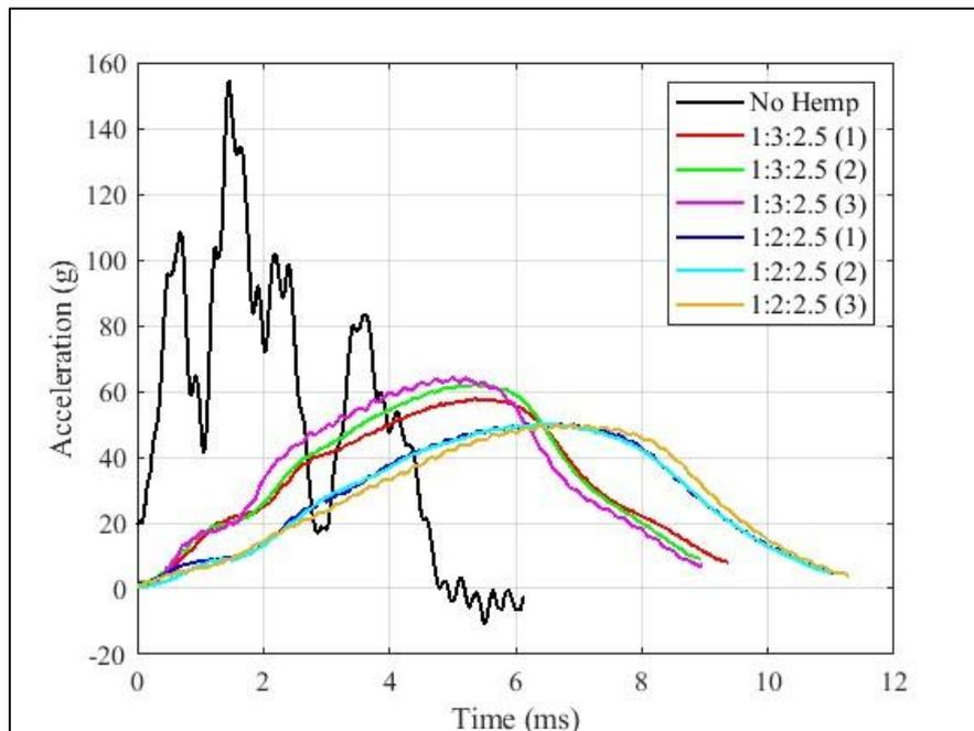
Figure 70. Effect of hemp : binder : water ratio on the drop weight acceleration-time response for 30 cm drop-height.
