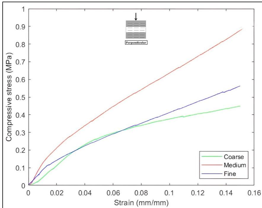
Figure 39. Effect of particle size on the compressive stress-strain relationship of hempcrete specimens loaded perpendicular to the hemp shives' orientation at 28 days.
