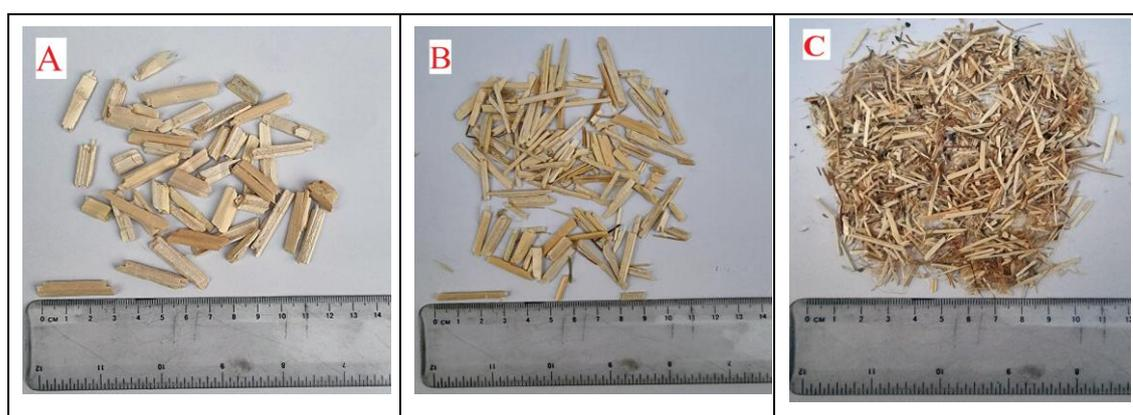
Figure 10. Hemp shives used in the study: A) Coarse, B) Medium, C) Fine.
