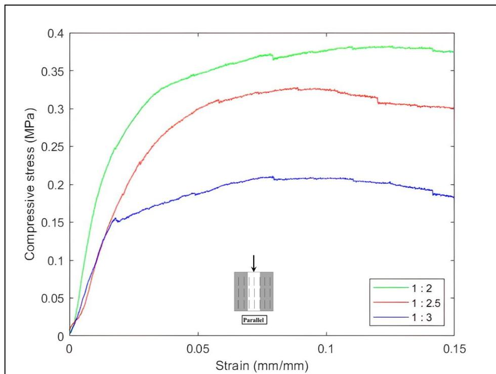
Figure 42. Effect of hemp : water on the compressive stress-strain relationship of hempcrete specimens loaded parallel to the hemp shives' orientation at 28 days.
