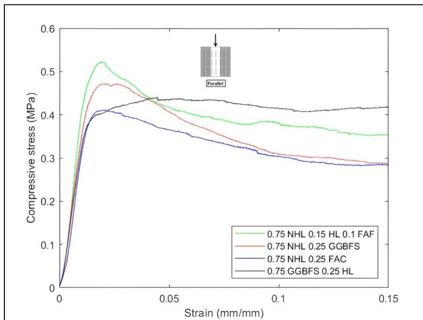
Figure 45. Effect of binder composition on the compressive stress-strain relationship of hempcrete specimens loaded parallel to the hemp shives' orientation at 180 days.
