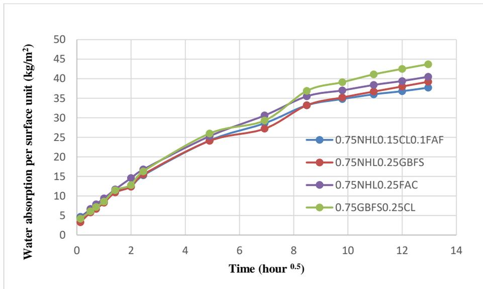
Figure 63. Effect of binder composition on the capillary water absorption of hempcrete.
