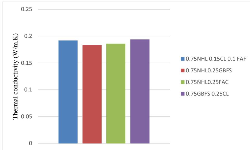
Figure 58. Effect of binder composition on the thermal conductivity of hempcrete.
