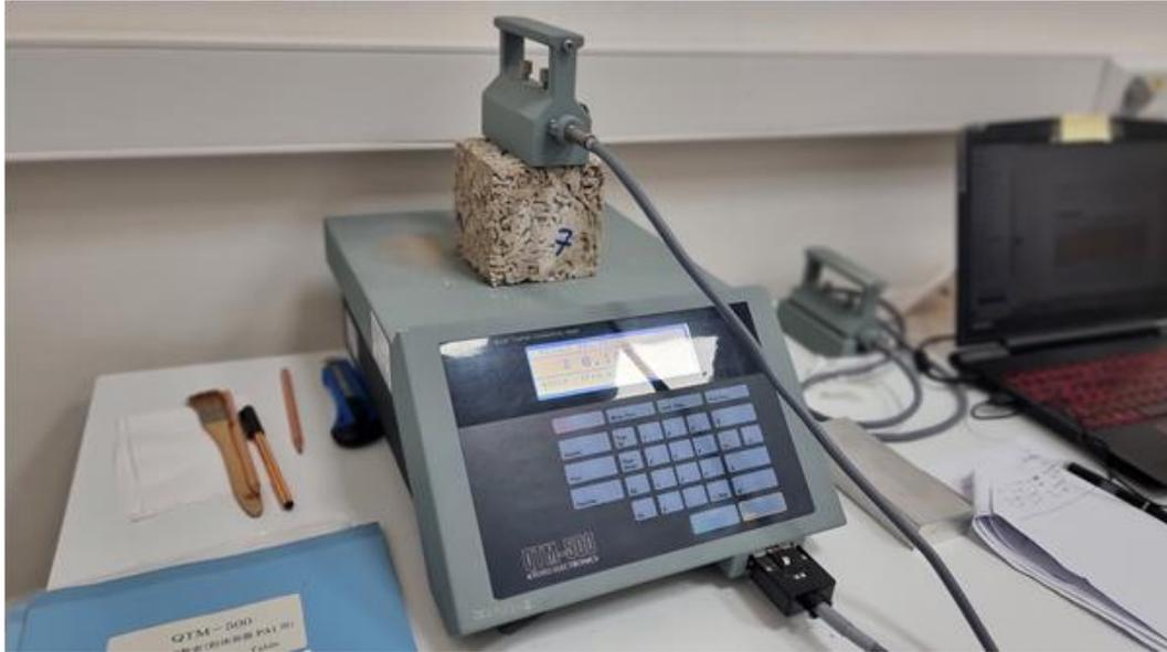
Figure 23. Thermal conductivity test of hempcrete specimens.
