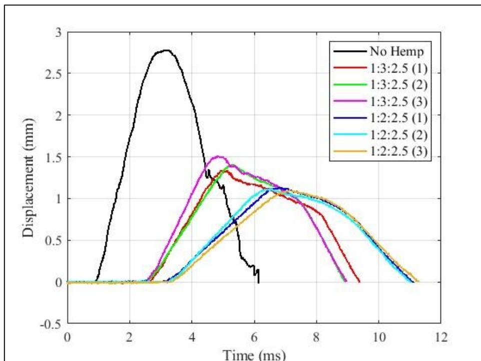
Figure 73. Effect of hemp : binder : water ratio on the mid-span displacement response of reinforced concrete beam for 30 cm drop-height.
