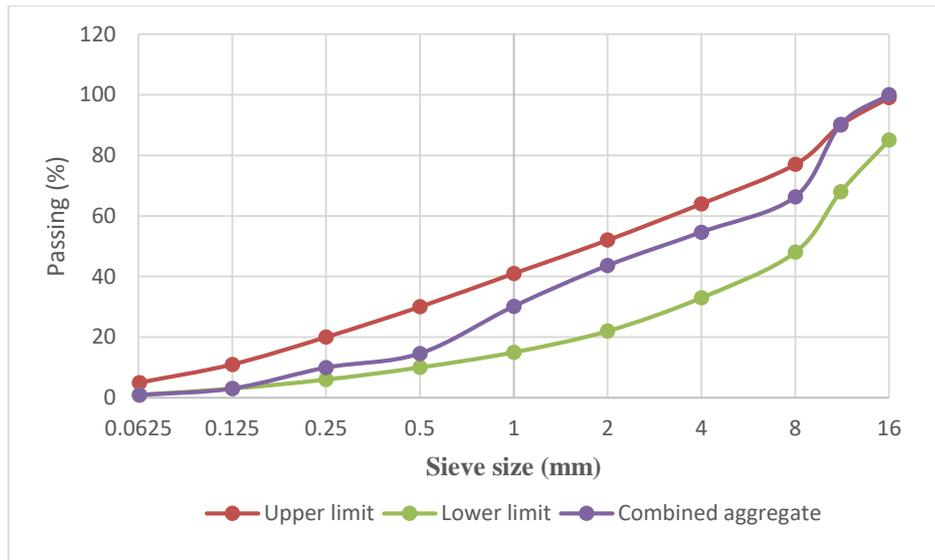
Figure 11. Gradation curve of combined aggregate.
