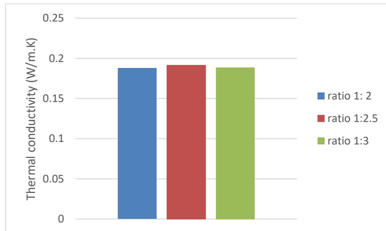
Figure 61. Effect of hemp : water ratio on the thermal conductivity of hempcrete.
