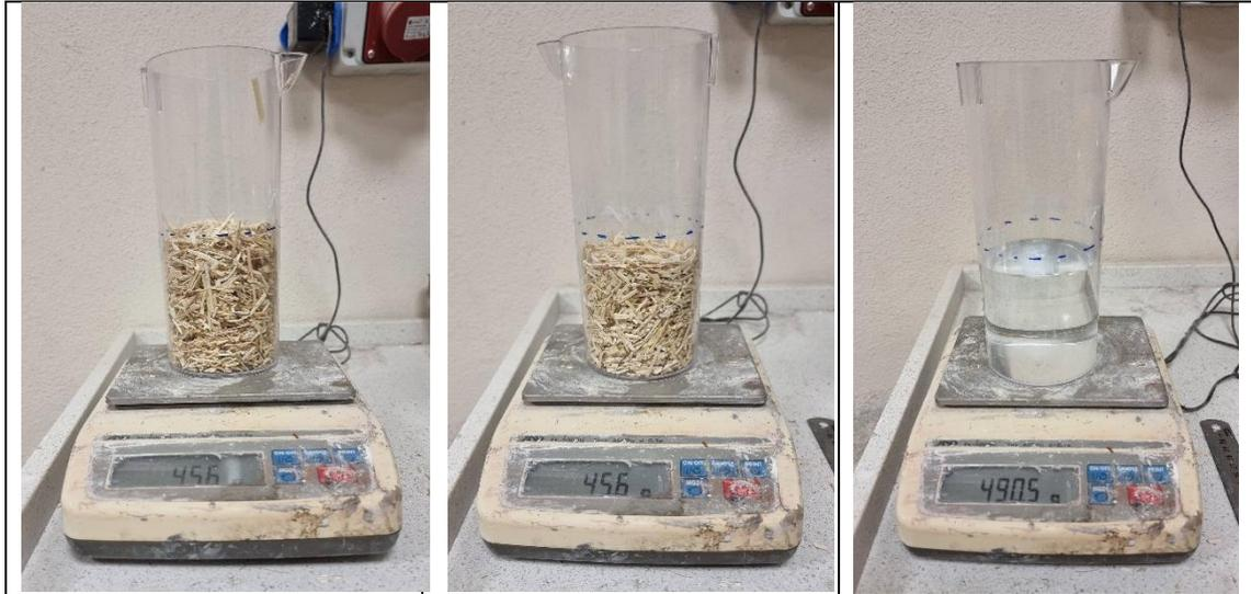
Figure 20. Dry bulk density test of hemp shives.
