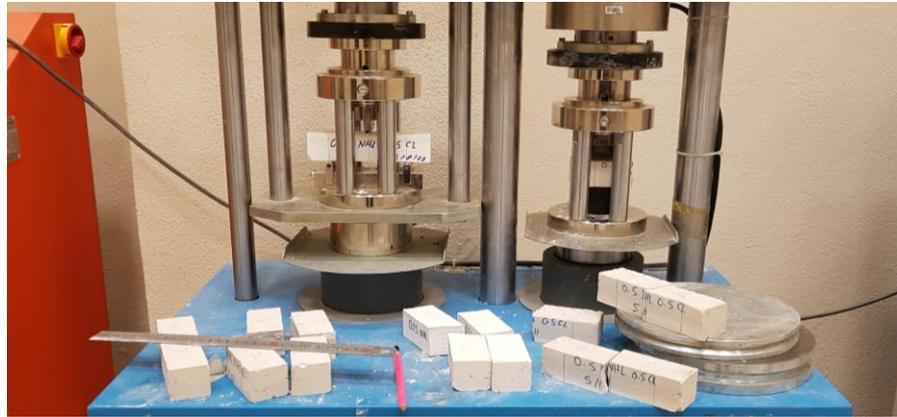
Figure 18. Testing the compressive strength of specimens remaining from the flexural strength test.
