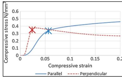
Figure 9. Stress-strain curve of the parallel and perpendicular direction. (Source: Williams, Lawrence, and Walker 2017)
