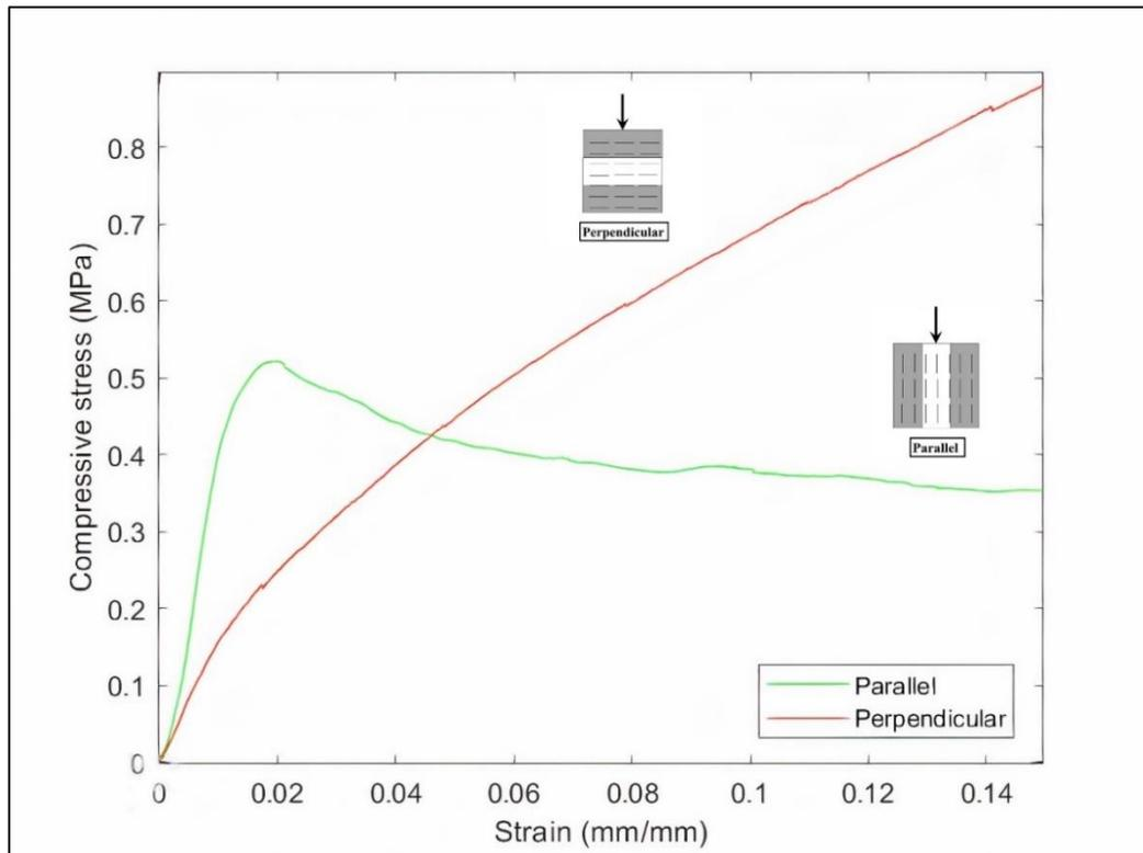
Figure 53. Comparison of the stress-strain curve behavior of Mix 1 when the load is applied parallel and perpendicular to the hemp shiv orientation at a strain of 0.15
