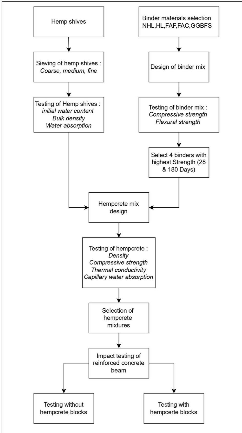
Figure 27. Flow chart of the experimental procedure for preparing and testing hempcrete specimens.
