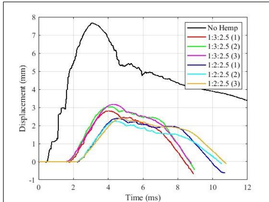
Figure 74. Effect of hemp : binder : water ratio on the mid span displacement response of reinforced concrete beam for 100 cm drop-height.
