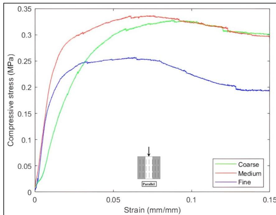
Figure 38. Effect of particle size on the compressive stress-strain relationship of hempcrete specimens loaded parallel to the hemp shives' orientation at 28 days.
