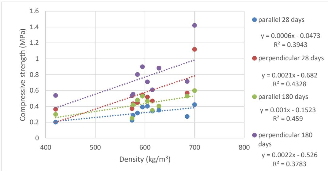
Figure 35. Compressive strength of hempcrete versus density.
