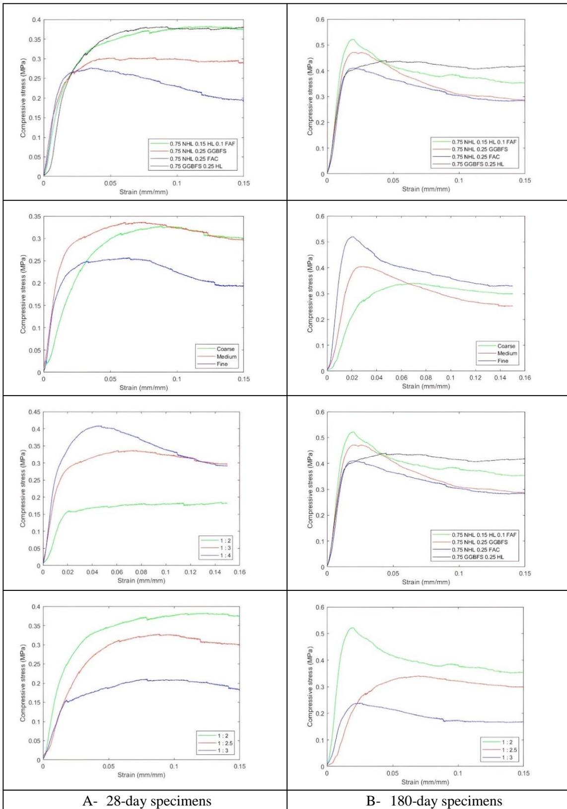
Figure 44. Compressive strength comparison of hemp concrete: A- 28-day specimens and B- 180-day specimens, with the load applied parallel to the hemp shives orientation.
