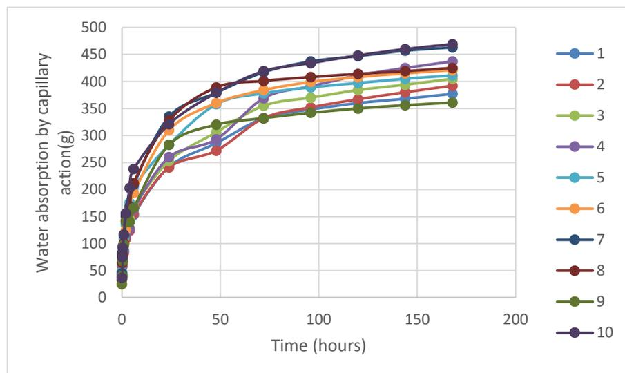
Figure 62. The capillary water absorption of hempcrete specimens for 7 days.
