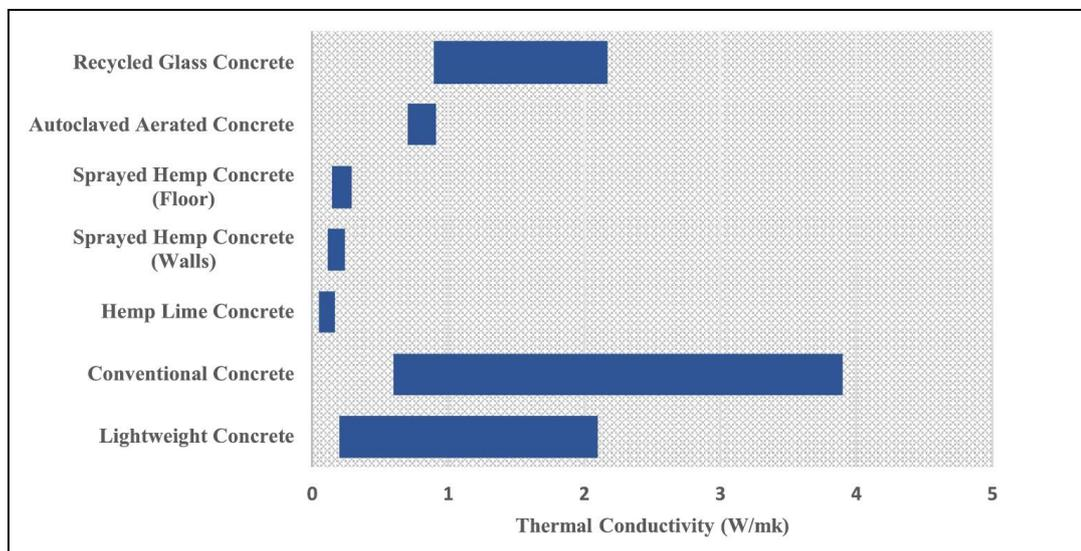
Figure 57. Comparison of hempcrete thermal conductivity with other types of concrete. (Source : Ansari, Tabish, and Zaheer 2025)
