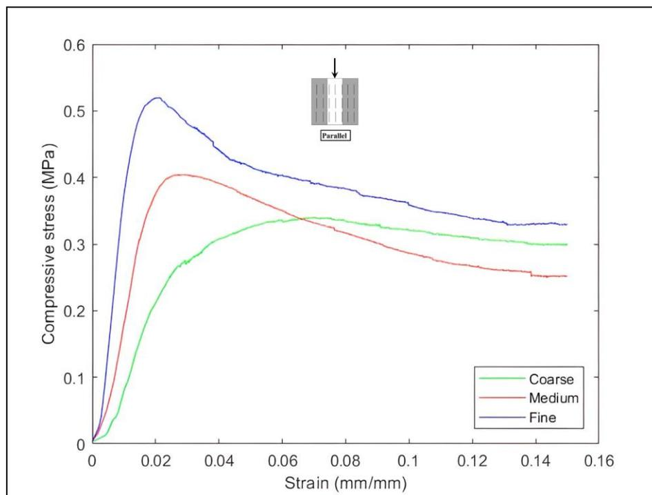
Figure 47. Effect of particle size on the compressive stress-strain relationship of hempcrete specimens loaded parallel to the hemp shives' orientation at 180 days
