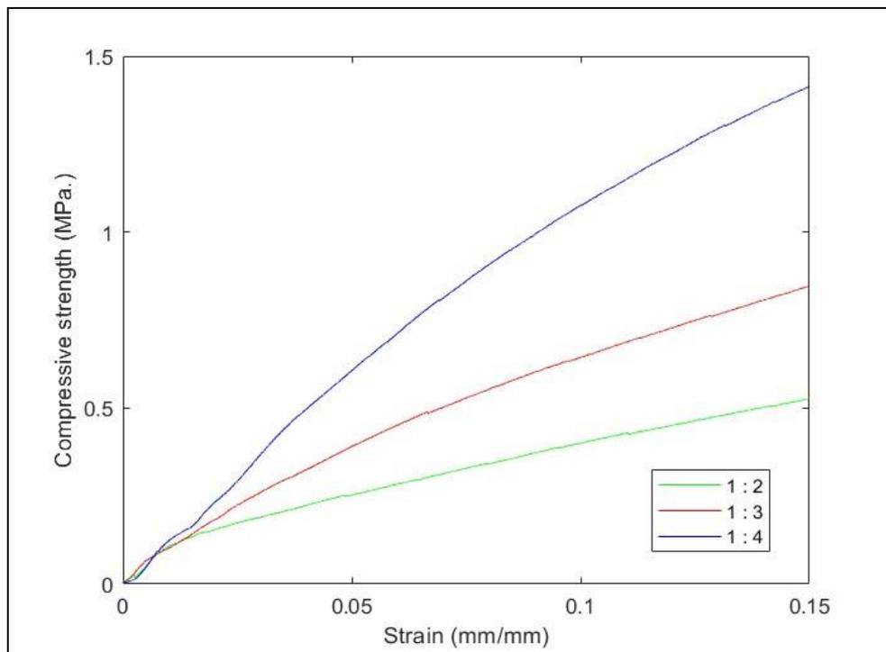
Figure 50. Effect of hemp : binder ratio on the compressive stress-strain relationship of hempcrete specimens loaded perpendicular to the hemp shives' orientation at 180 days.
