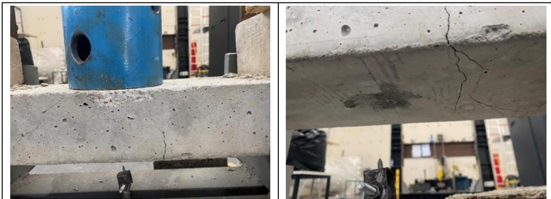
Figure 72. Damage suffered by the reinforced concrete beam after 100 cm drop test with no hempcrete.
