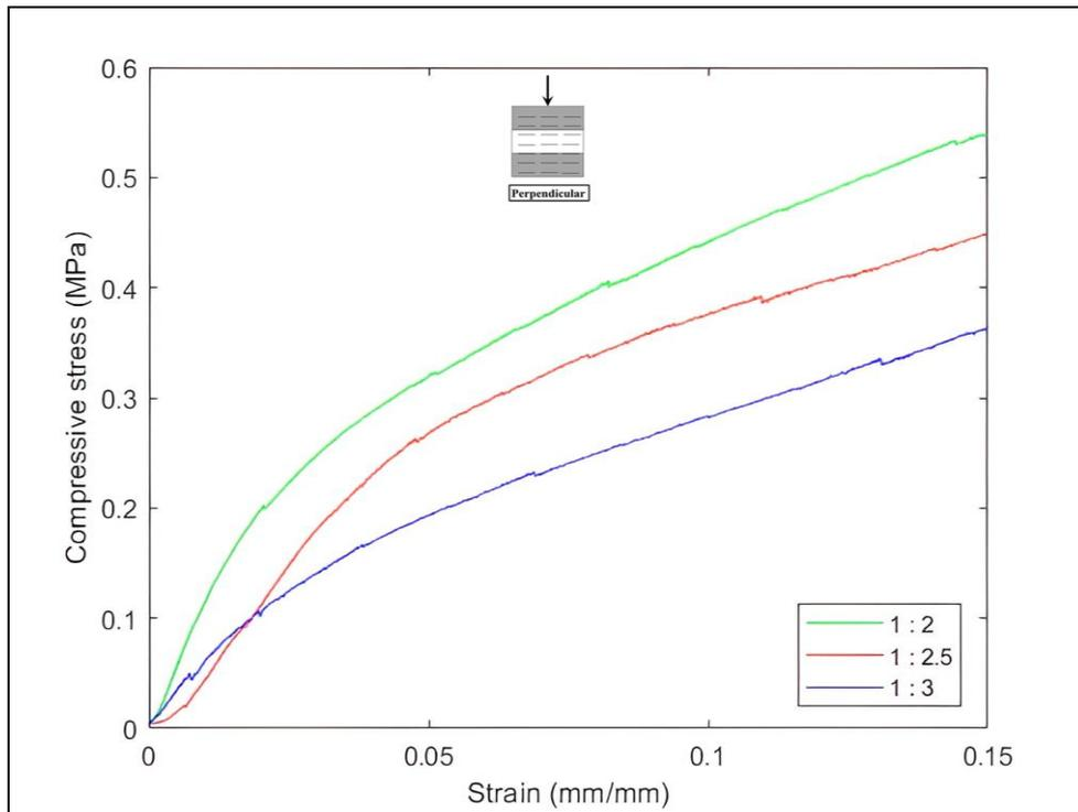
Figure 43. Effect of hemp : water on the compressive stress-strain relationship of hempcrete specimens loaded perpendicular to the hemp shives' orientation at 28 days.
