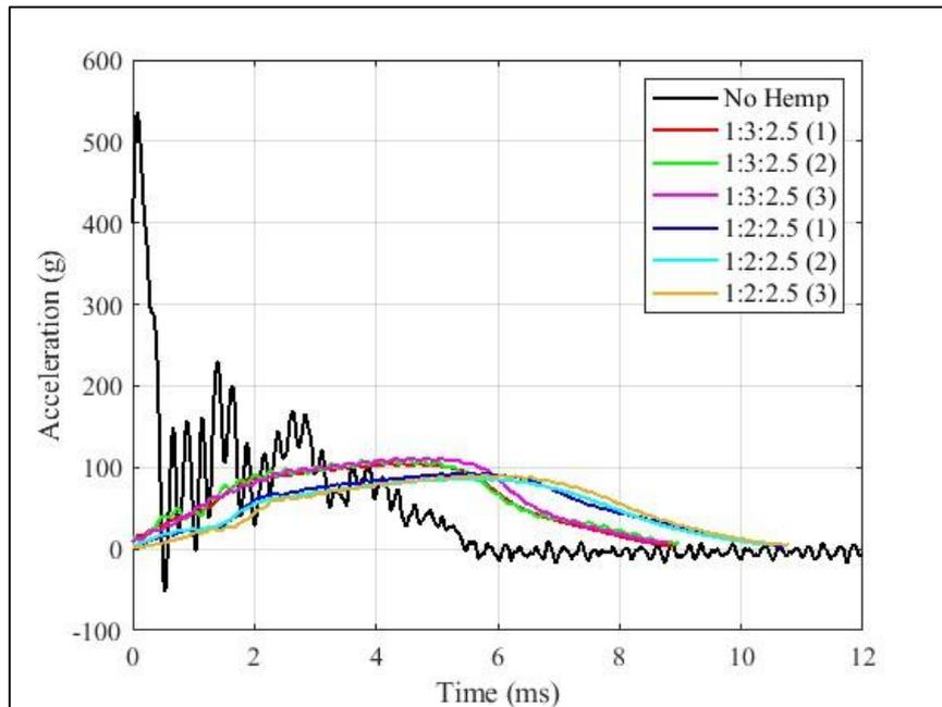
Figure 71. Effect of hemp : binder : water ratio on the drop weight acceleration-time response for 100 cm drop-height.
