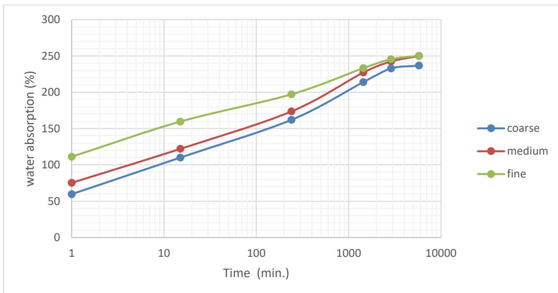
Figure 31. Water absorption of the three hemp shive sizes coarse, medium, and fine.
