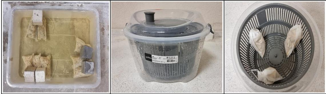
Figure 19. Water absorption test of hemp shives.
