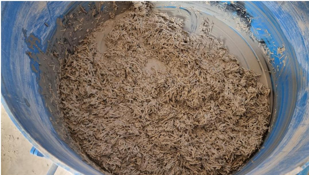
Figure 14. A pan-type concrete mixer used for mixing hempcrete.
