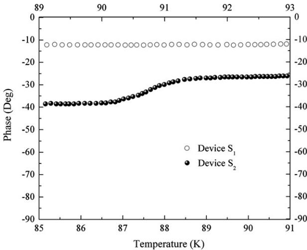
Fig. 7. The phase of the IR response of the small area bolometers  $S_1$  and  $S_2$  as a function of temperature at 100 Hz modulation frequency. Upper and bottom scales represent the temperature of the devices  $S_1$  and  $S_2$ , respectively.
