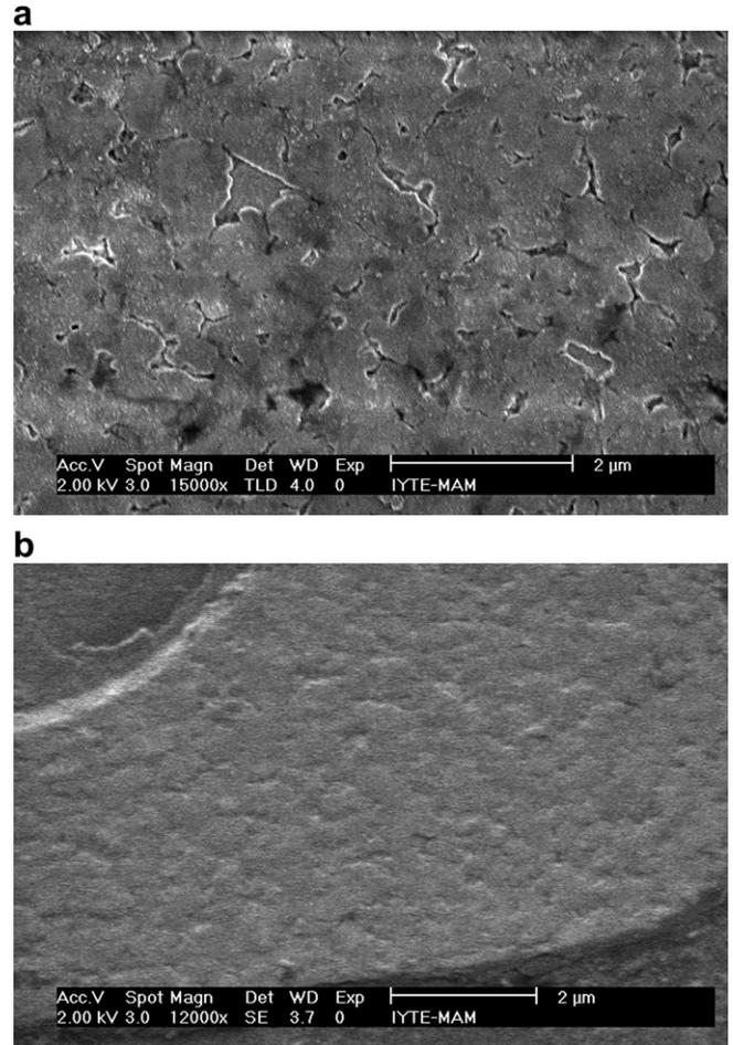
Fig. 3. SEM micrographs of the large area devices (a) with wide transition width ( $L_2$ ) and (b) with narrow transition width ( $L_1$ ).
