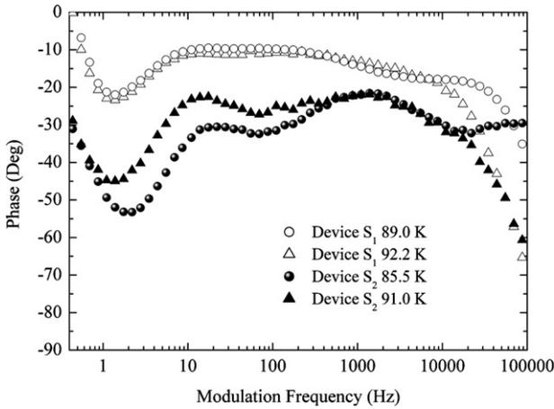
Fig. 6. The phase of the IR response of the small area bolometers  $S_1$  and  $S_2$  versus  $f_m$  measured at temperatures around  $T_{c-zero}$  and  $T_{c-onset}$ .
