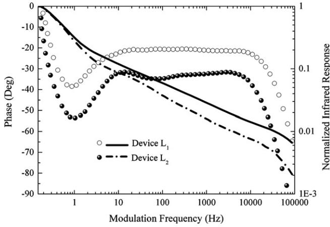
Fig. 5. The phase and magnitude of the IR response of the large area bolometers  $L_1$  and  $L_2$  as a function of  $f_m$  measured at temperatures around  $T_c$ .
