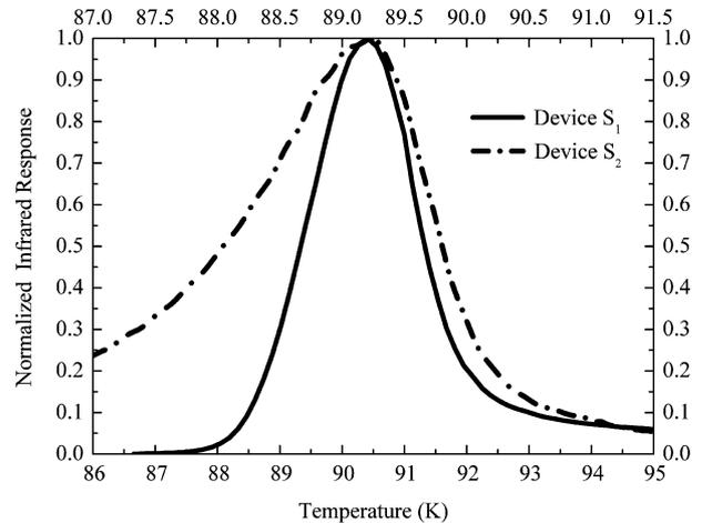
Fig. 1. The normalized magnitude of the IR response of the small area bolometers  $S_1$  and  $S_2$  versus temperature measured at 110 Hz,  $f_m$ . Upper and bottom scales represent the temperature of the devices  $S_2$  and  $S_1$  respectively. Note that the IR response is proportional to  $dR/dT$  of the bolometers and hence a wide IR response indicates wide superconducting transition width.
