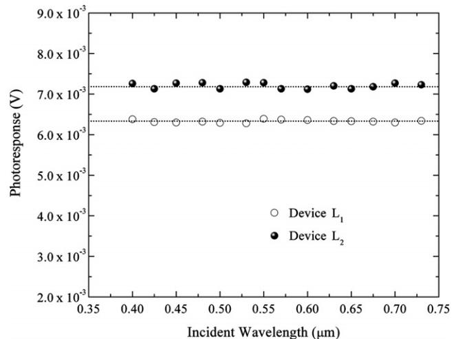
Fig. 9. Photoresponse of the bolometers  $L_1$  (at 88.5 K) and  $L_2$  (at 87.2 K) as a function of wavelength at  $I_b = 1$  mA and  $f_m = 11$  Hz.
