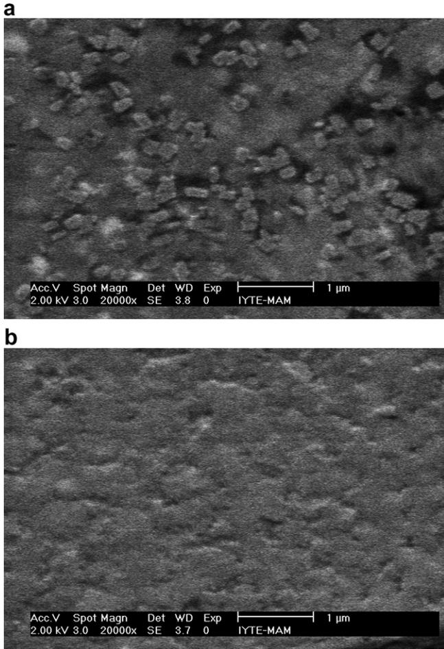
Fig. 2. SEM micrographs of the small area devices (a) with wide transition width ( $S_2$ ) and (b) with narrow transition width ( $S_1$ ).
