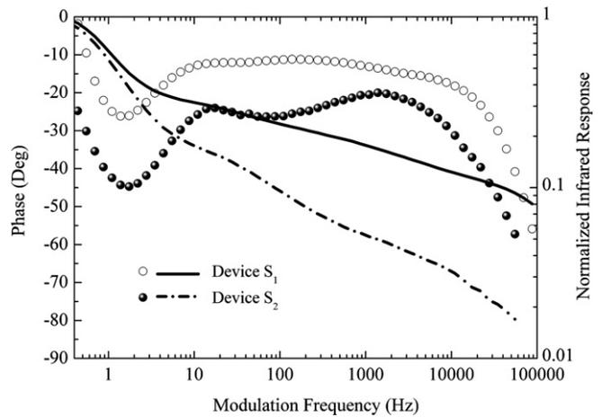
Fig. 4. The phase and magnitude of the IR response of the small area bolometers  $S_1$  and  $S_2$  versus  $f_m$  measured at temperatures around  $T_c$ .
