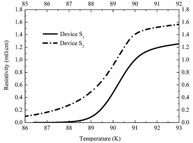
Fig. 8. Resistivity versus temperature curves of the bolometers  $S_1$  and  $S_2$ . Upper and bottom scales represent the temperature of the devices  $S_2$  and  $S_1$ , respectively.
