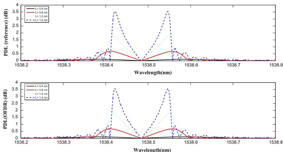
**Fig. 3.** Computed PDL evolution as a function the grating length (a) based on analytical formula applied on a single FBG [22,23], (b) simulated OFDR system proposed in the current work.
