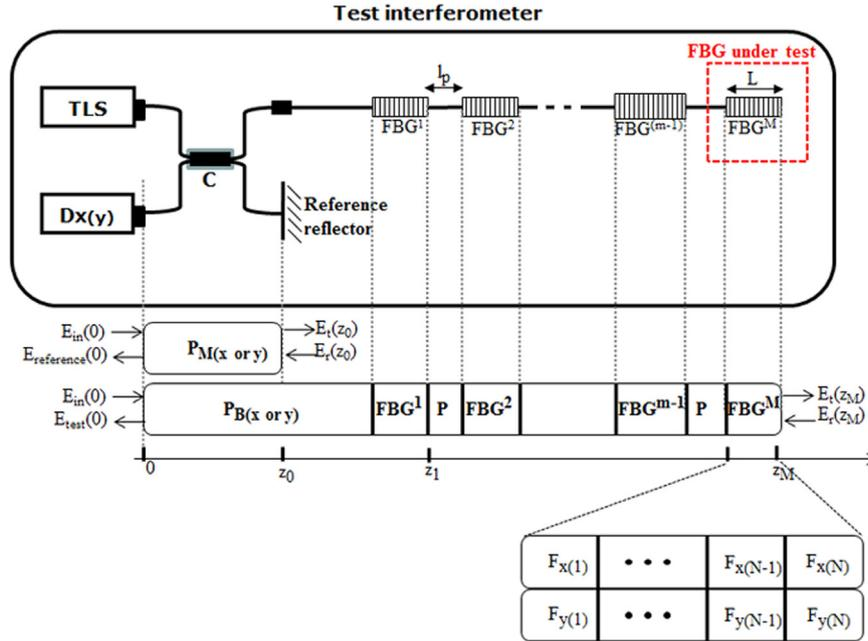
**Fig. 2.** Schematic of the test interferometer for the numerical simulation model.
