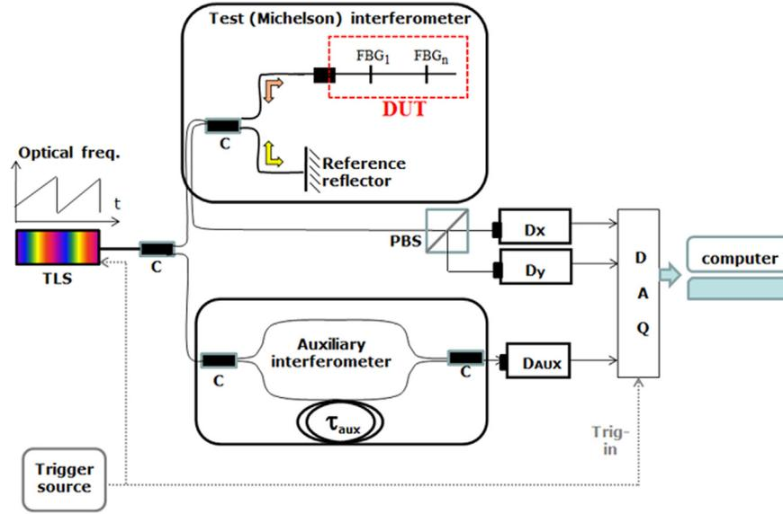
**Fig. 1.** Schematic of polarisation sensitive OFDR system (TLS: tunable laser source, Dx and Dy are detectors for both polarisation modes, C: coupler, PBS: polarisation beam splitter, DAQ: data acquisition card).
