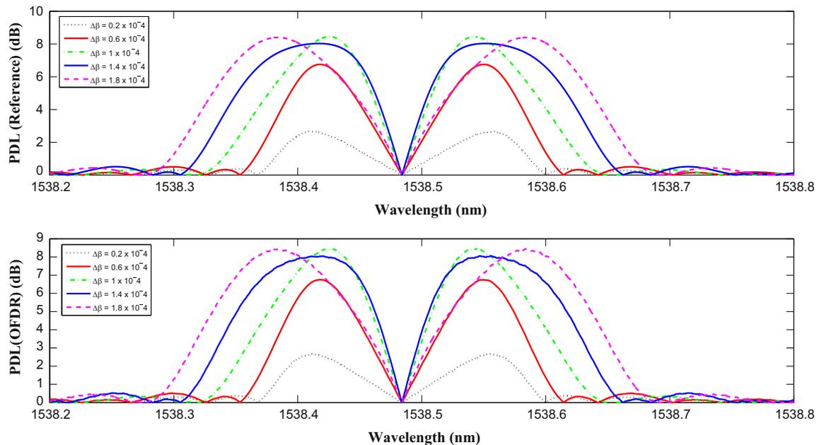
**Fig. 4.** Computed PDL evolution as a function the birefringence value (a) based on analytical formula applied on a single FBG [22,23], (b) simulated OFDR system proposed in the current work.
