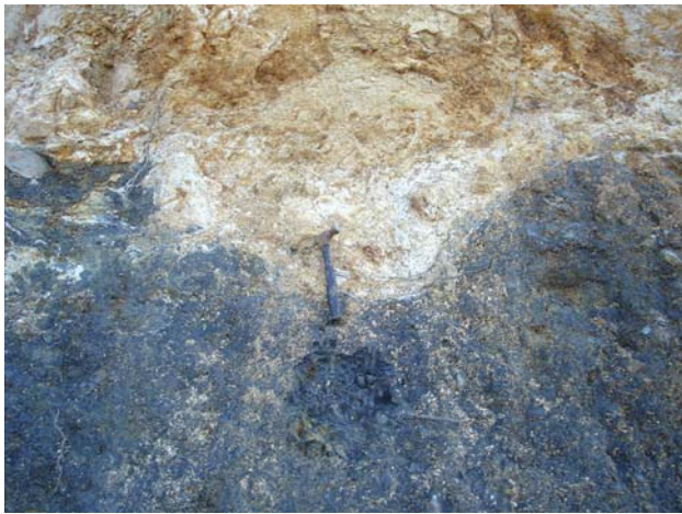
Fig. 8 Argillization (upper light-colored section) and propylitization (lower dark-colored section) in Kirazlı area
