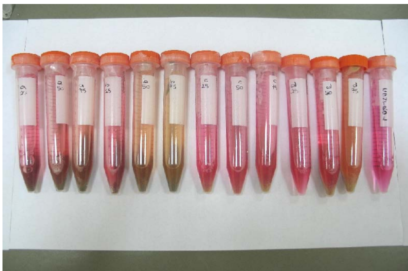
Figure 8.13. Color of cancer cell growth media treated with digested and non-digested zeolite samples with different doses. Left to right: each 3 tubes grouped as : a, b, c, d and they were Z1, Z1D, Z2, Z2D respectively and their concentrations in each group were (left to right) 25-50 and 75 mg/ml zeolite, last sample is untreated one as control sample.
