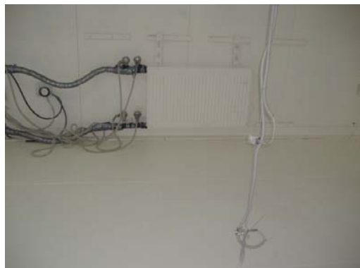
Figure 5.3. Measuring of air temperature inside the test room.
