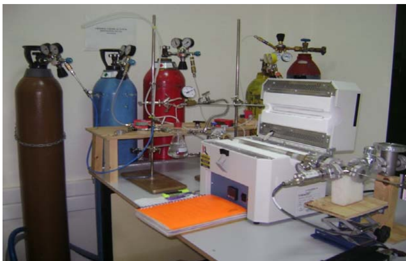
Figure 4.2. The TCVD system, CNL Lab in Physics Department IYTE
