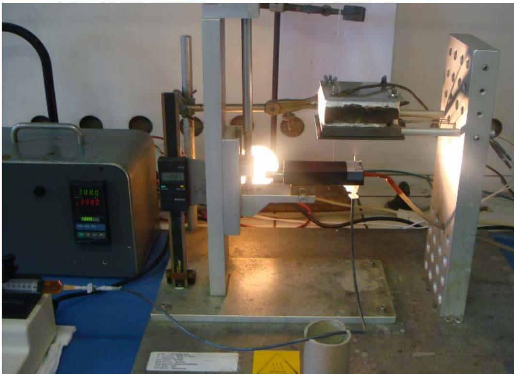
Figure 3.5. The photograph of ESD setup used in sample preparation (in LEPMI, Grenoble, France)
