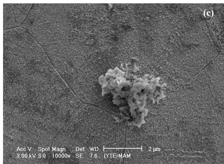
Figure 6.3. SEM photomicrographs (a) before and (b, c) after the immersion test taken from 60 keV at 200 °C N ion implanted specimen.
