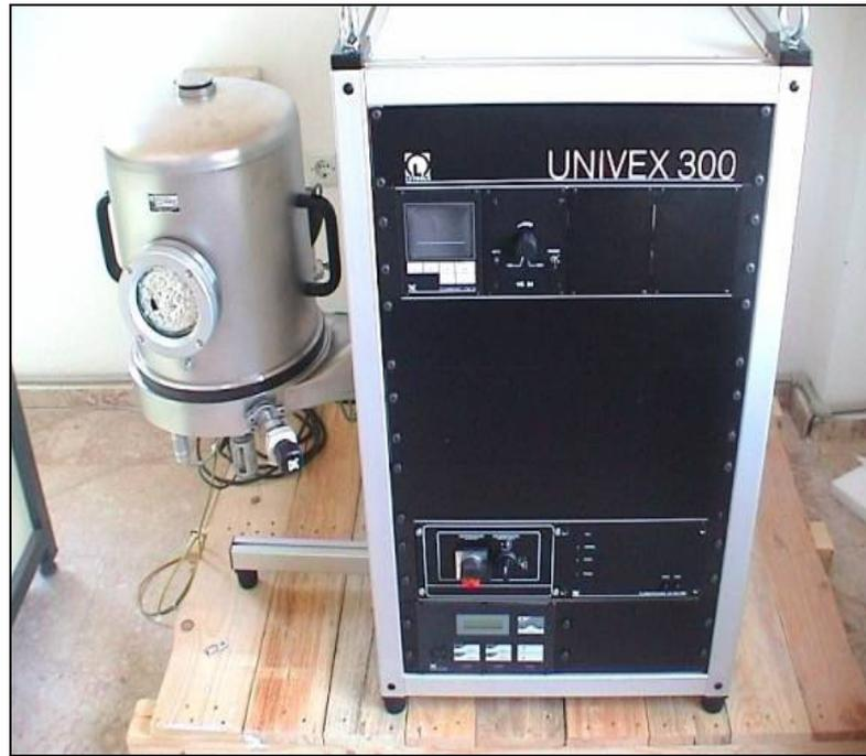
Figure 2.1. The photograph of thermal evaporation system used for deposition gold surface.
