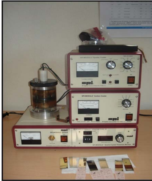
Figure 3.5. SPI Sputter coater for gold deposition.
