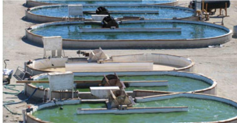
Figure 2.3. A raceway pond.
