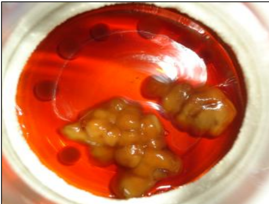
Figure 4.27. Pellet image from exo-PG production with mutant A. sojae in phosphoric acid hydrolysate at 1x10 5 spore mL -1 concentration
