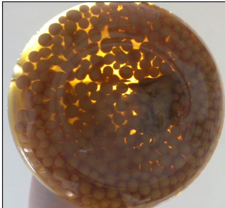
Figure 4.25. Pellet image from exo-PG production with mutant A. sojae in phosphoric acid hydrolysate with different pH adjustment
