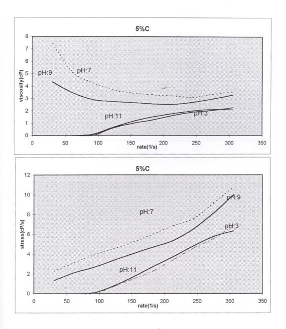
Figure 7.4 : Viscosity vs.rate and rate vs.stress graphs for powder C having 5% solid
