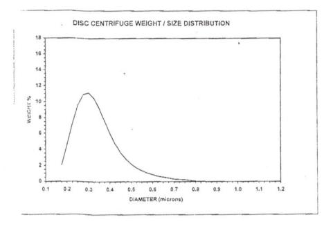
Figure 6.1 : Particle Size Distribution Diagram for Powder C
