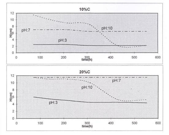
Figure 7.2 : H vs.t at 3 different pH for powder C without surfactant
