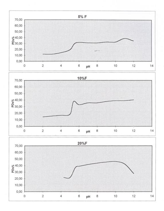
Figure 7.23 : PD% vs.pH at saturation time for powder F without surfactant
