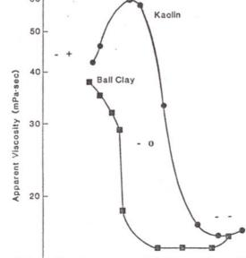
Figure 5.5 : Viscosity of clay slips decreases with increasing pH above IEP of edges of clay particles, but viscosity remains high at low pH because faces remain negative.[27]
