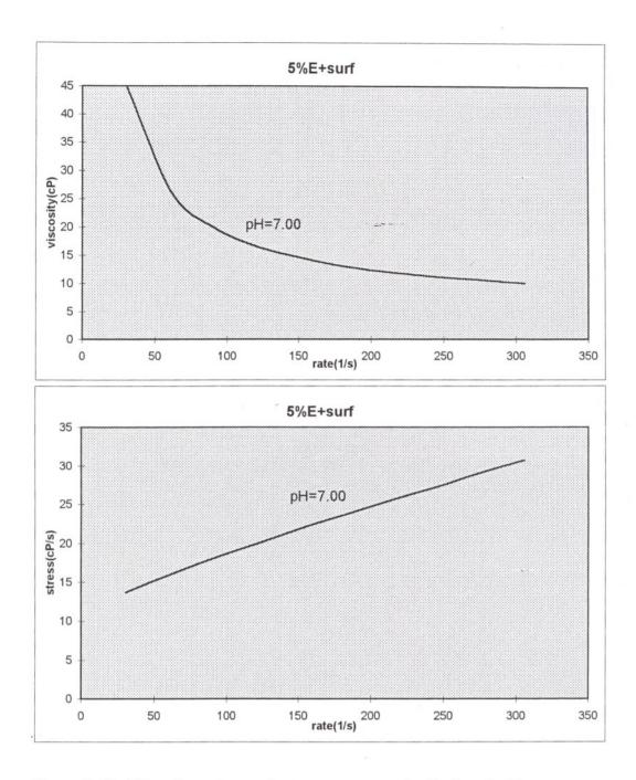
Figure 7.19 : Viscosity vs.rate and rate vs.stress graphs for Powder E having surfactant
