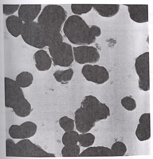
Figure 2.4 : SEM picture of silica coated rutile titania particles.[6]
