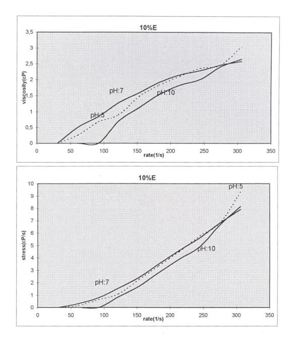
Figure 7.15 : Viscosity vs.rate and rate vs.stress graphs for powder E having 10% solid
