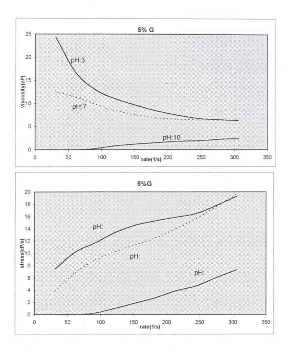
Figure 7.30 : Viscosity vs.rate and rate vs.stress graphs for powder G having 5% solid
