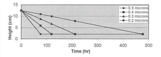
Figure 7.1 : Schematic representation of H vs. t for monosize particles for 10% solids.
