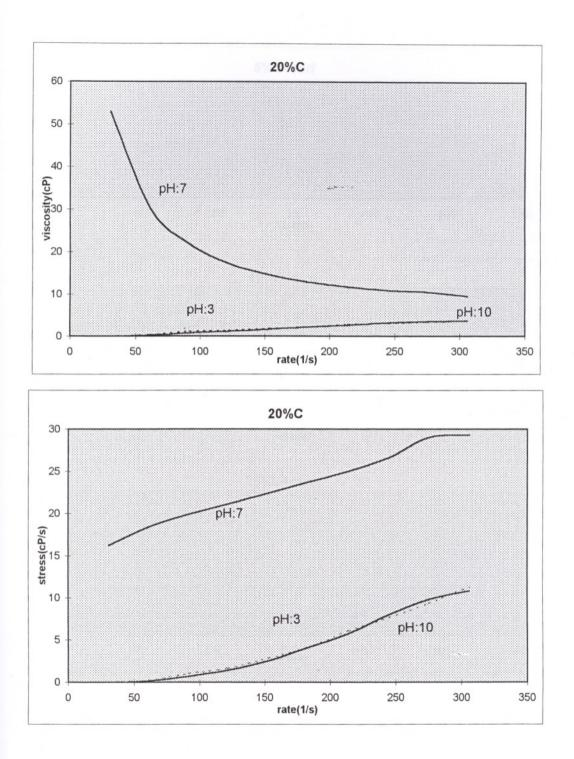
Figure 7.6 : Viscosity vs.rate and rate vs.stress graphs for powder C having 20% solid
