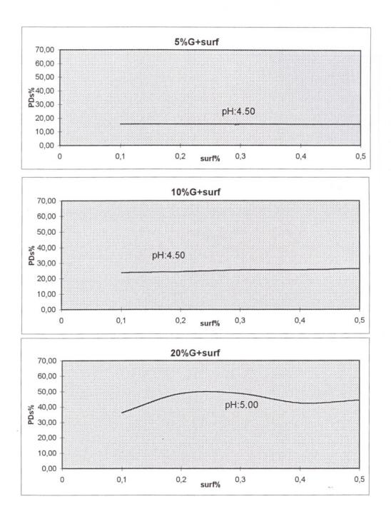
Figure 7.32 : PD% vs.surf% for powder G at saturation time
