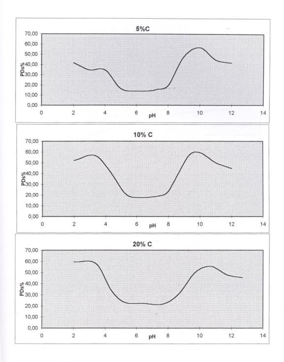
Figure 7.3 : PD% vs.pH at saturation time for powder C without surfactant
