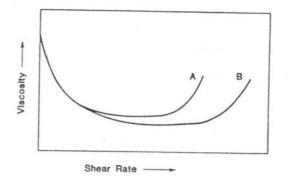
Figure 5.3 : General variation of viscosity with shear rate for two slurries indicating shear thickening behaviour at a high shear rate. The less well-dispersed system A exhibits shear thickening behaviour at a lower shear rate.[27]
