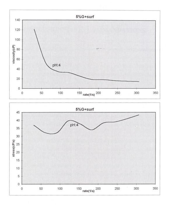
Figure 7.33 : Viscosity vs.rate and rate vs.stress graphs for powder G (5%) having surfactant
