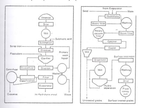
Figure 2.3 : Flow diagram of titania production.[26]
