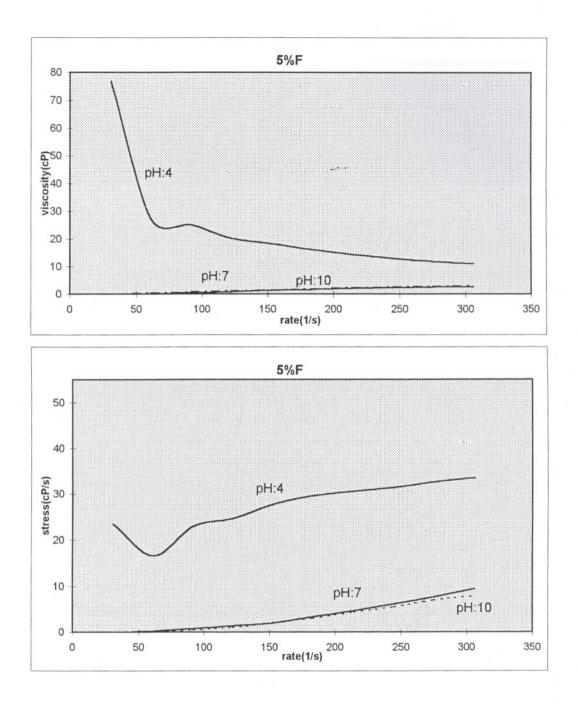
Figure 7.24 : Viscosity vs.rate and rate vs.stress graphs for powder F having 5% solid
