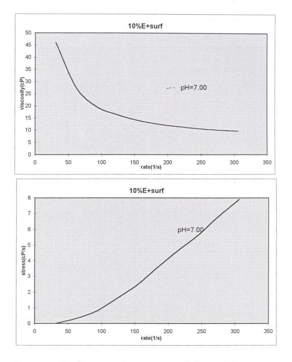
Figure 7.20 : Viscosity vs.rate and rate vs.stress graphs for powder E (10% solid) having surfactant
