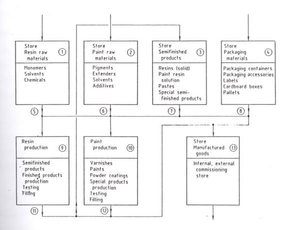
Figure 3.1 : Material Flow in paint production.[31]
