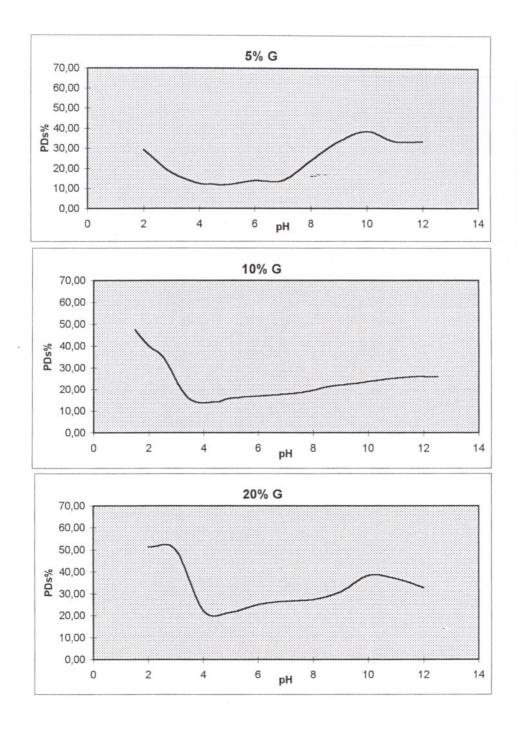
Figure 7.29 : PD% vs.pH at saturation time for powder G without surfactant
