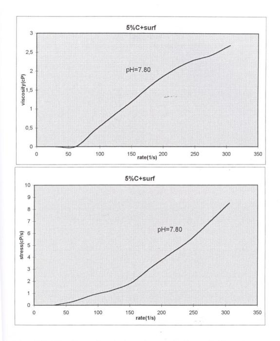
Figure 7.9 : Viscosity vs.rate and rate vs.stress graphs for powder C — having surfactant
