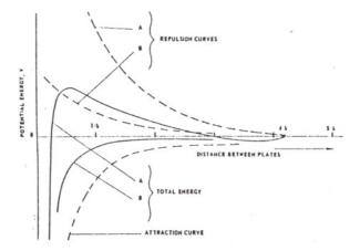
Figure 4.7: Total potential energy curve. Two repulsion curves, A and B, are shown. The solid lines are the resultant curves obtained by adding either A or B to the dotted attraction curve. In one case, a total repulsion curve is obtained, in the other case, the total curve is one of attraction.
