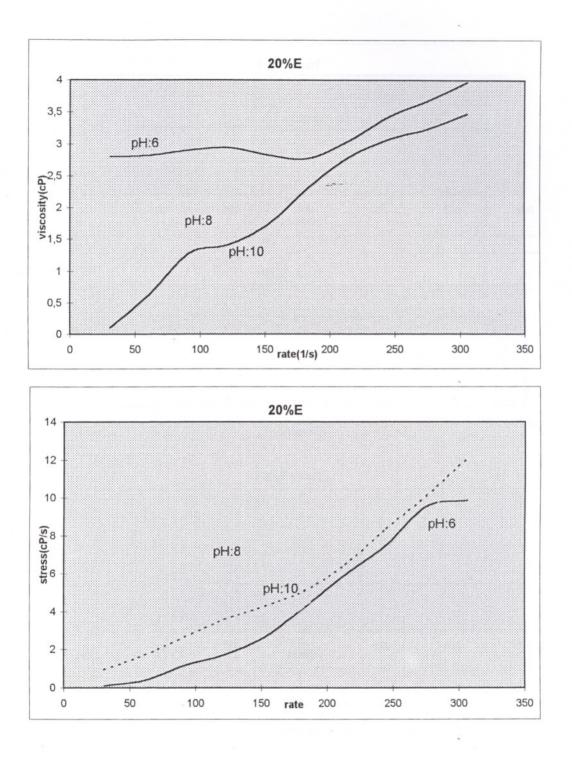
Figure 7.16 : Viscosity vs.rate and rate vs.stress graphs for powder E having 20% solid
