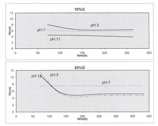
Figure 7.28 : H vs.t at 3 different pH for powder G without surfactant
