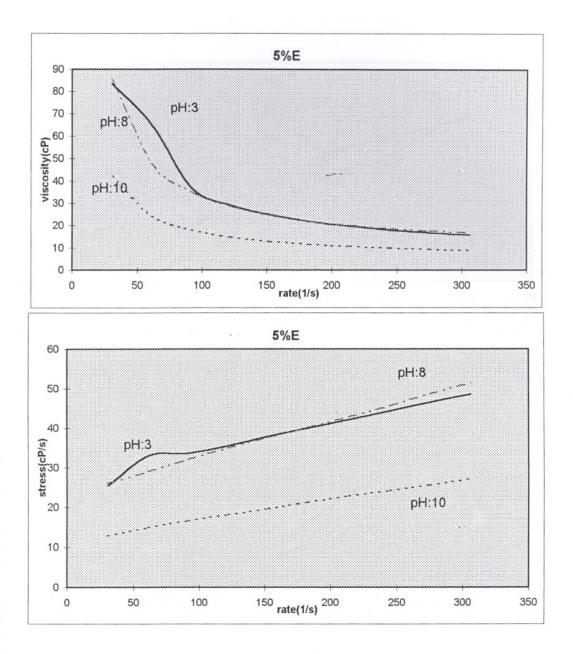
Figure 7.14 : Viscosity vs.rate and rate vs.stress graphs for powder E having 5% solid
