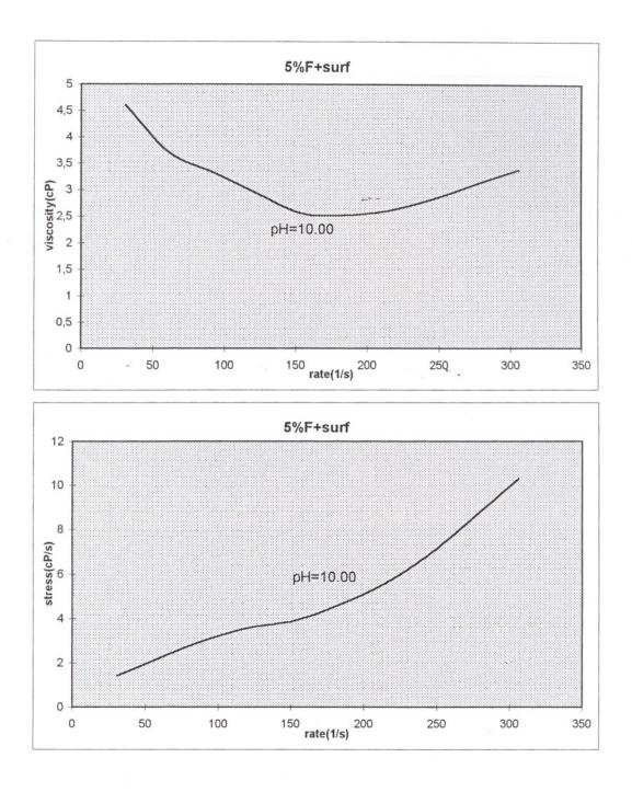
Figure 7.27: Viscosity vs.rate and rate vs.stress graphs for powder F (5%) having surfactant
