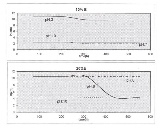
Figure 7.12 : H vs.t at 3 different pH for powder E without surfactant
