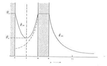
Figure 4.6 : Double layer between two flat plates ,as compared with double layer for a single plate.[4]
