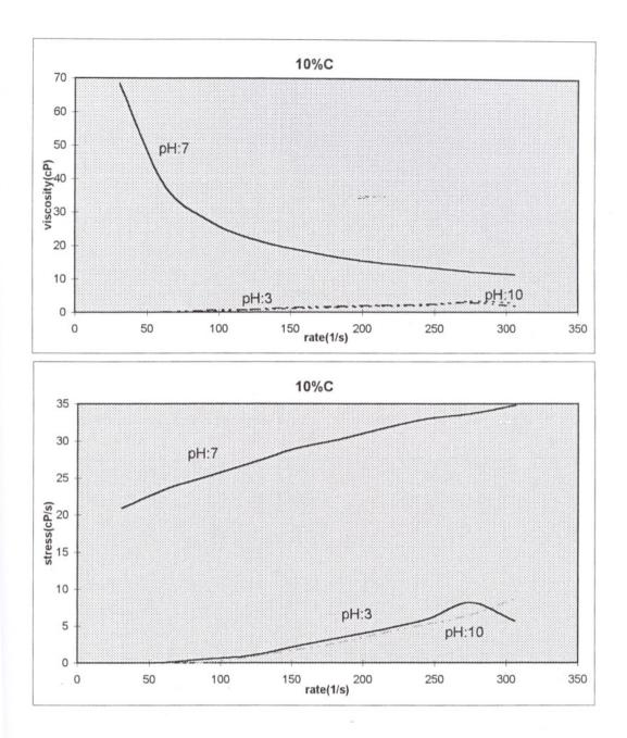
Figure 7.5 : Viscosity vs.rate and rate vs.stress graphs for powder C having 10% solid
