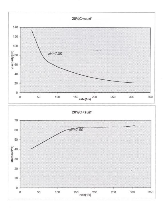
Figure 7.11 : Viscosity vs.rate and rate vs.stress graphs for powder C (20% solid) having surfactant
