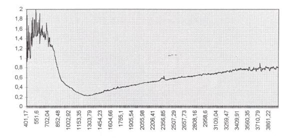
Figure A.4 : FTIR Spectra of anatase powder E
