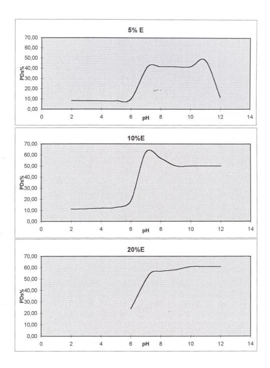
Figure 7.13 : PD% vs.pH at saturation time for powder E without surfactant
