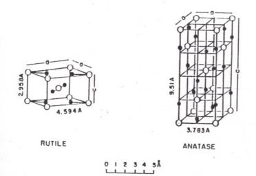
Figure 2.1 : Crystal Unit Cells of Anatase and Rutile.[26]
