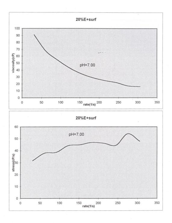
Figure 7.21 : Viscosity vs.rate and rate vs.stress graphs for powder E (20% solid) having surfactant
