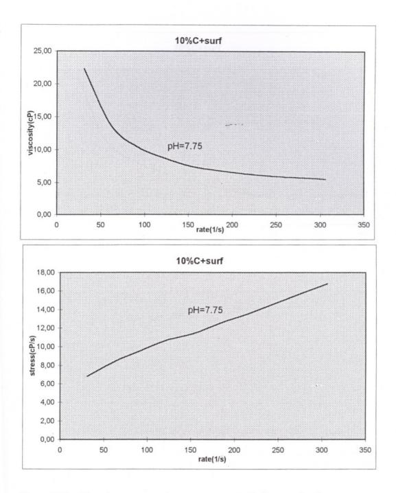
Figure 7.10 : Viscosity vs.rate and rate vs.stress graphs for powder C (10% solid) having surfactant
