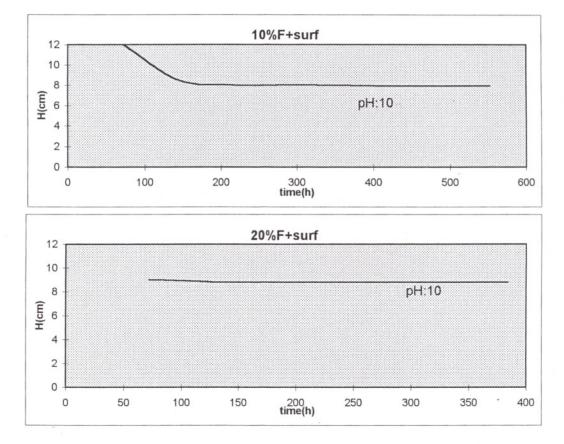
Figure 7.25 : The trend of H vs.t for titania powder F having surfactant
