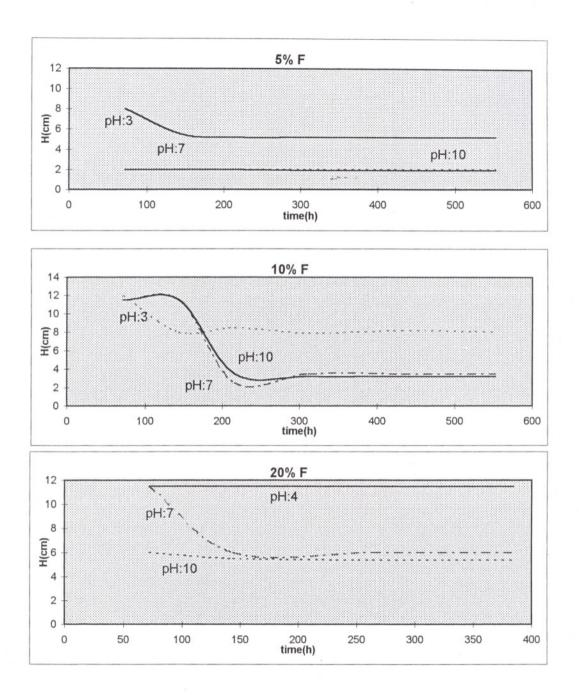
Figure 7.22 : H vs.t at 3 different pH for powder F without surfactant
