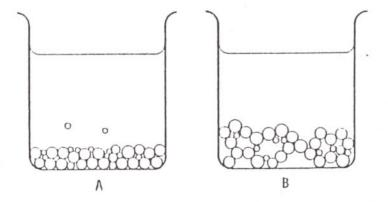
Figure 5.6 : Structure of sediments. A-) compact sediment from stable suspension B-)loose sediment from flocculated suspension.[24]
