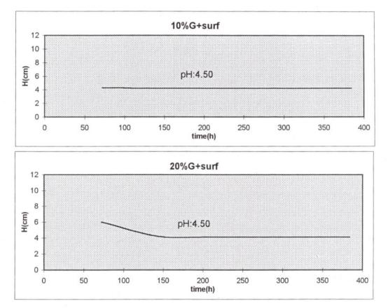
Figure 7.31 : The trend of H vs.t for titania powder G having surfactant
