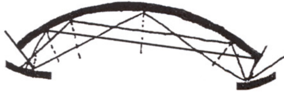
Figure 3- 29 Profile of the original dome with Anthemius' reflectors on the window sills. (Potamianos 1997 p163)
