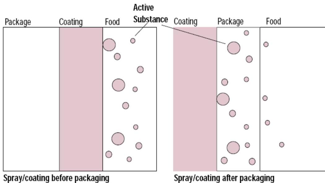
Figure 2.5. Effect of the coating location on the diffusion of antimicrobial agents
