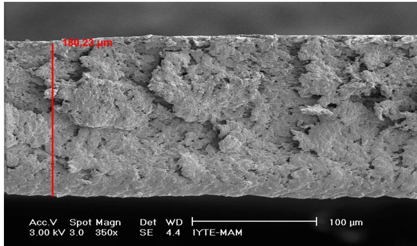
Figure 5.5. The cross-section photograph of zein film obtained by scanning electron microscope (SEM) (magnification x350; content of film produced by stirring method:  $175 \mu\text{g}/\text{cm}^2$  lysozyme )
