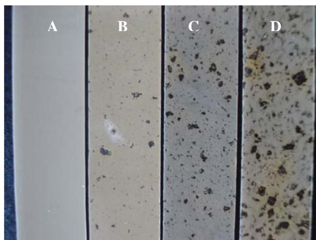
Figure 5.1. Photographs of different zein films produced by stirring method (Film contents: A, control film; B, 175  $\mu\text{g}/\text{cm}^2$  lysozyme; C, 350  $\mu\text{g}/\text{cm}^2$  lysozyme; D, 700  $\mu\text{g}/\text{cm}^2$  lysozyme. The background was black to make the light yellow semi-transparent protein aggregates visible)
