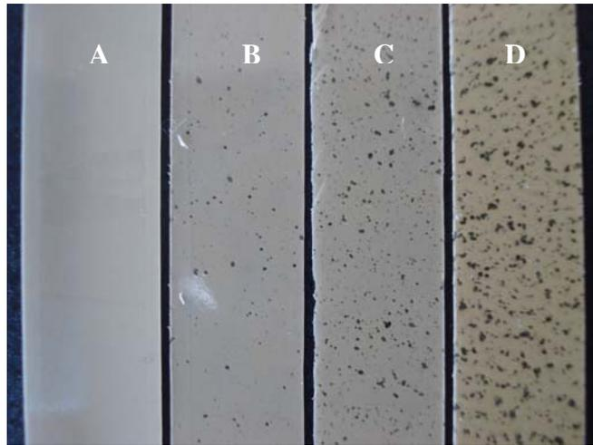
Figure 5.2. Photographs of different zein films produced by homogenization method (Film contents: A, control film; B, 175  $\mu\text{g}/\text{cm}^2$  lysozyme; C, 350  $\mu\text{g}/\text{cm}^2$  lysozyme; 700  $\mu\text{g}/\text{cm}^2$  lysozyme The background was black to make the light yellow semi-transparent protein aggregates visible.)
