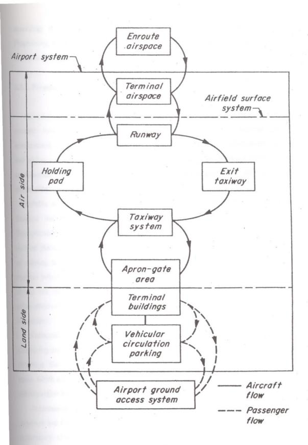
Fig. 3.2 Components of the airport system for a large airport source: Horonjeff and McKelvey (2)
