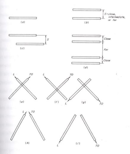
Fig. 4.1 Typical runway configurations a) single runway b) two parallel runways-even threshold c) two parallel runways-staggered threshold d)four parallel runways e) intersecting runways g) intersecting runways h) open-V runways I) open-V runways.
