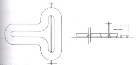
(f) <u>AMOEBA</u> This system is an extension of the race track system. The only difference being that the baggage is manually loaded directly onto the conveyor by an attendant behind a wall and out of view from the passengers.
