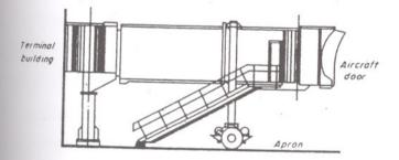
Fig. 4.15 Typical aircraft loading bridges source: Horonjeff and McKelvey (2)
