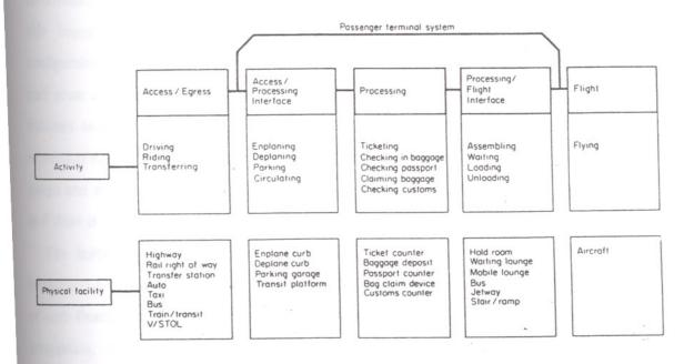
Fig. 4.11 Components of the passenger terminal system
