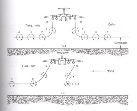
Fig. 4.10 Vortex movement near the ground showing the effect of wind. Source. Horonjeff and Mc Kelvey (2)
