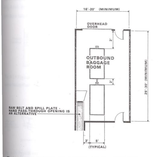
Fig.4.14 Outbound baggage room typical raw belt conveyor installation source: J.de Chiara and J. Callender (9)
