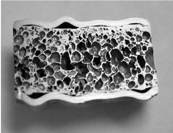
Fig. 3. Section through an F1 Al tube showing tube walls pulling away from foam.
