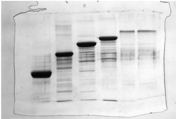
Fig. 2. Molecular weight of AMG (Novo) enzyme (lane 1: egg albumin (45,000 Da); lane 2: BSA (66,000 Da); lane 3: Phosphorylase B (97,400 Da); lane 4: \beta -galactosidase (116,000 Da); lane 5: AMG (Novo, 7.5 \mu l); lane 6: AMG (Novo, 10 \mu l)). 7.5% of SDS-PAGE.
