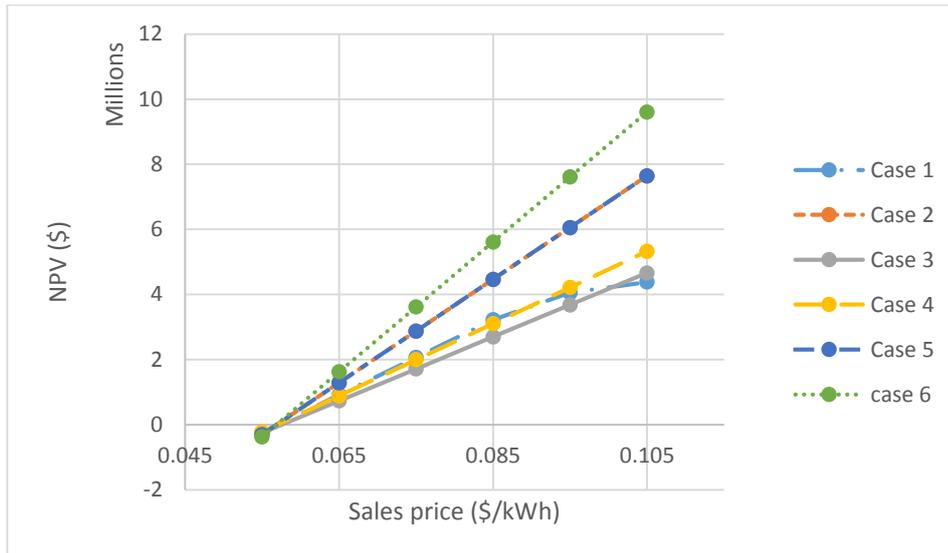
Figure 4.16. NPV of the DHE power generation versus electricity sales price rates.
