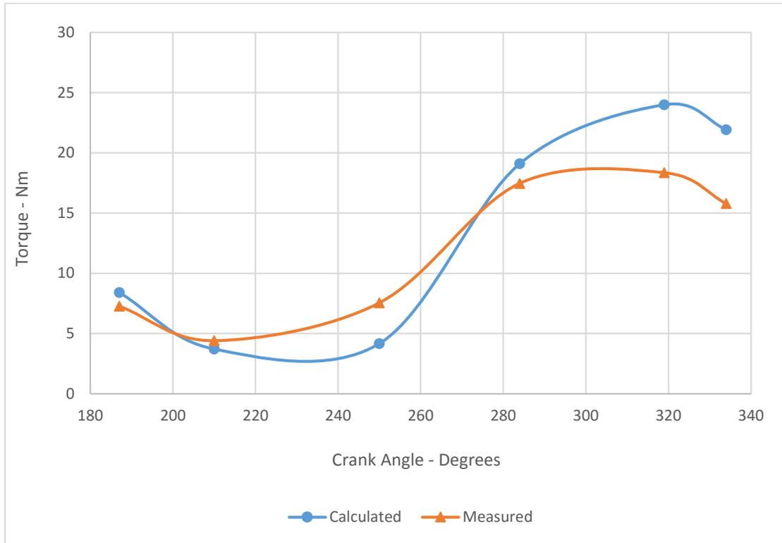
Figure 52. Measured Torque Results Compared to Calculated Torques
