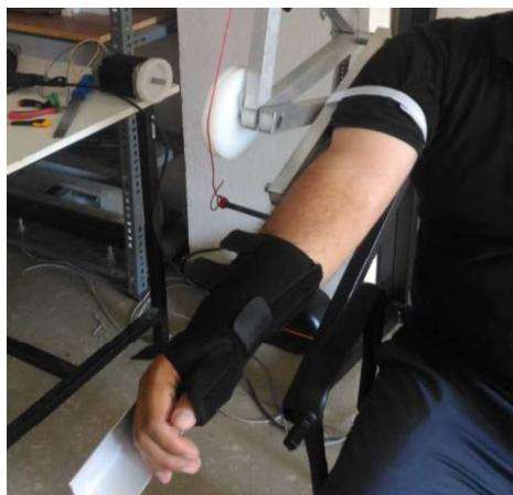
Figure 50. Attachment of the Human Arm to the System
