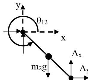
Figure 33. FBD of the Crank Link
