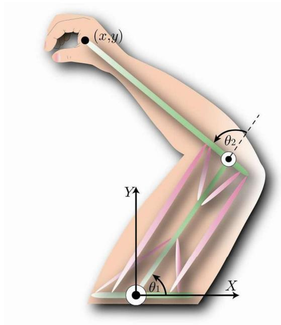
Figure 13. Human Arm as a 2R Serial Planar Kinematic Chain
