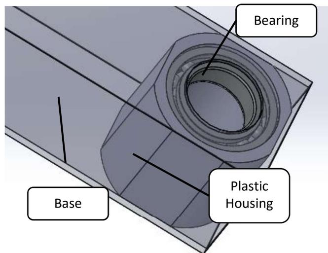
Figure 41. Kinematic Element Design on the Base
