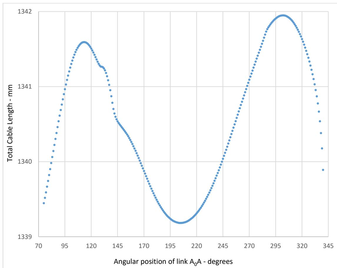
Figure 31. Total Cable Length Variation throughout the Motion
