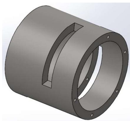
Figure 47. The CAD Model of Motor Pulley Casing
