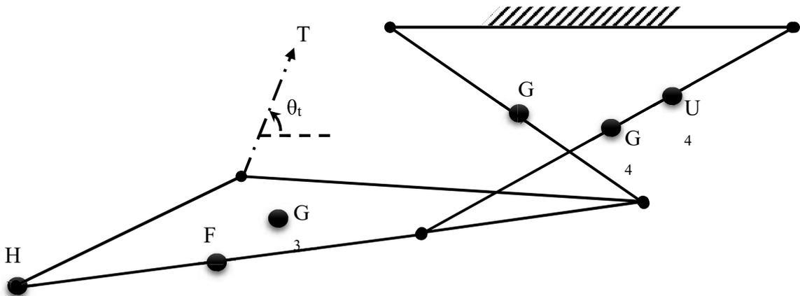
Figure 32. Mass Centers and Location of External Forces
