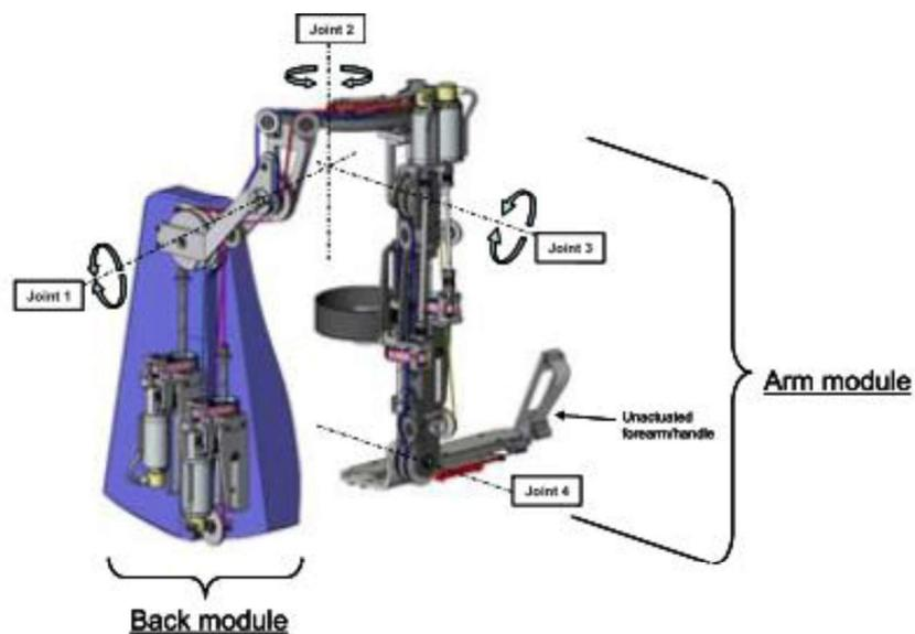
Figure 10. Actuator Mounting and Power Transmission of ABLE
