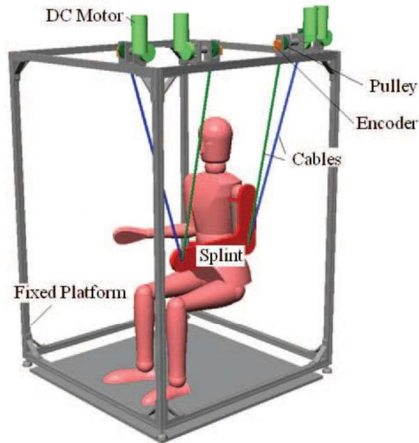
Figure 12. Arm Rehabilitation with a CDPM [14]
