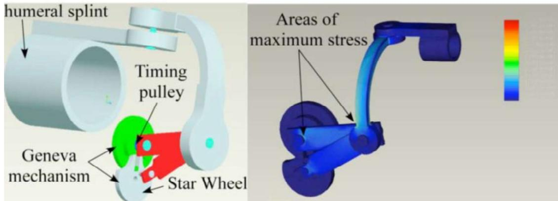
Figure 11. Shoulder Rehabilitation System with Geneva Mechanism [32]
