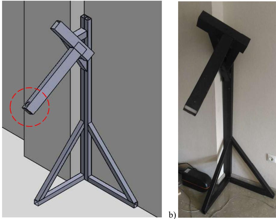
Figure 40. The Base Design: a) the CAD Model and b) the Manufactured Base
