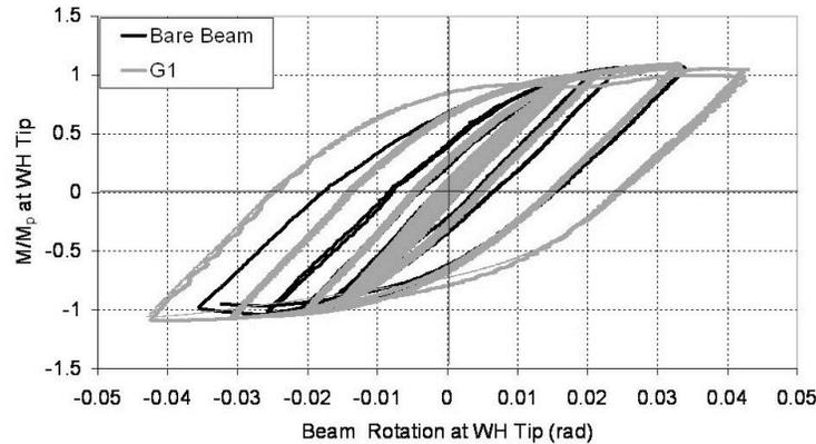
Fig. 10: Comparison of  $M/M_p$ -Beam Tip Rotation plots of Specimens G1 and B
