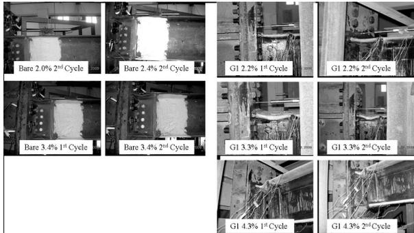
Fig. 8: Photos of Top Flange LB for Spec. B and G1
