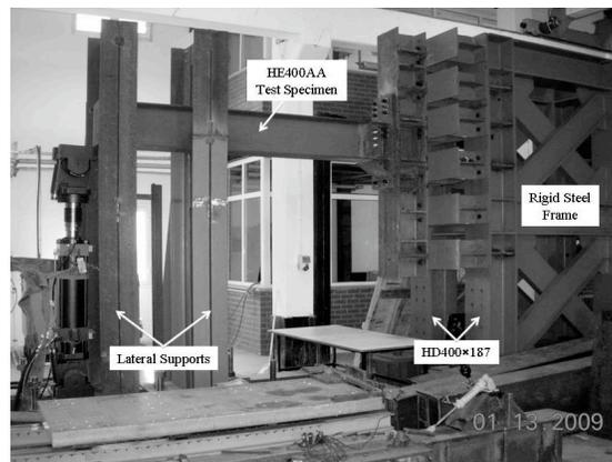
Fig. 2: Photograph of Test Setup and HE400AA Test specimen
