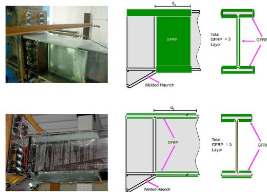
Fig. 5: Specimen G2 (top) and Specimen G3 (bottom)
