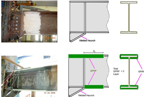
Fig. 4: Specimen Bare (top) and Specimen G1 (Bottom)
