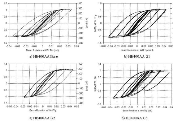
Fig. 7:  $M/M_p$ -Beam Tip Rotation Plots of Specimens
