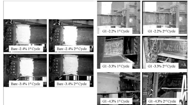
Fig. 9: Photos of Bottom Flange LB for Spec. B and G1
