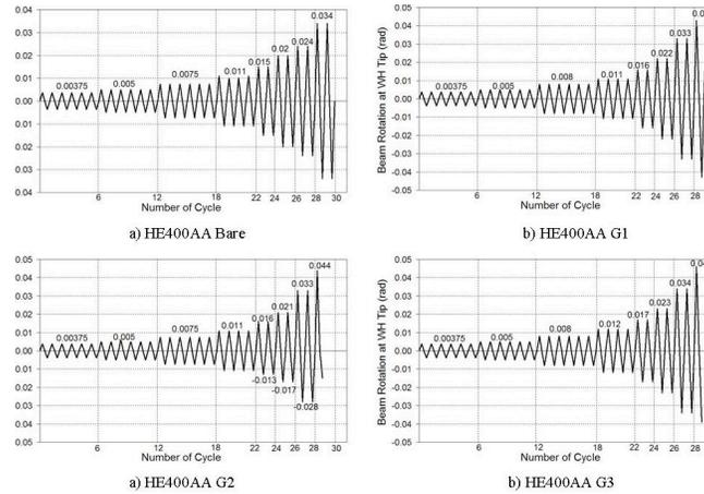
Fig. 6: Loading Sequences followed in the Cyclic Tests
