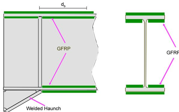
Fig. 1: GFRP Configuration used in the Analytical Study
