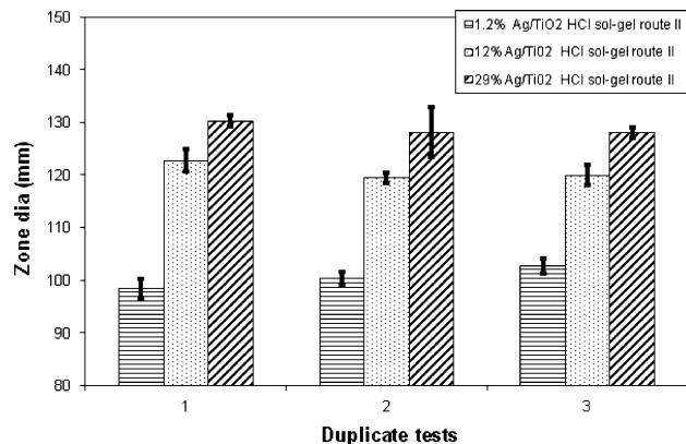
**Fig. 2** Disk diffusion method: Ag loading effect on the bactericidal activity of the xerogels made with HCl sol-gel route II
