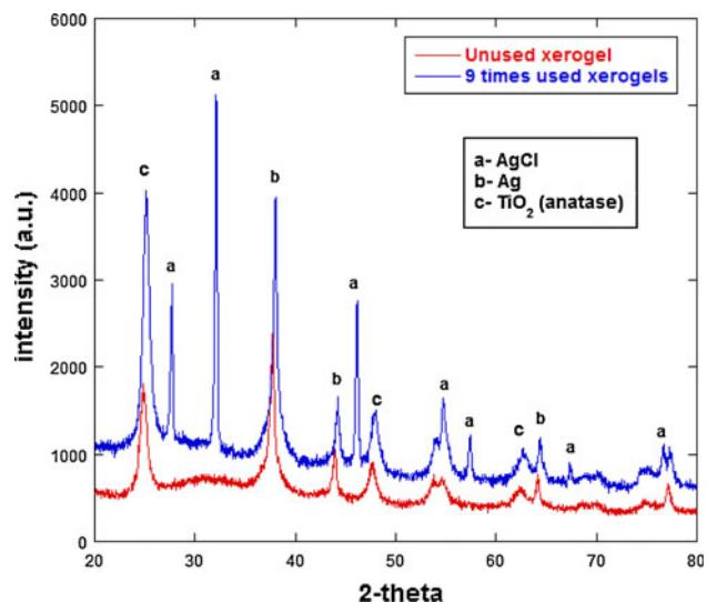
**Fig. 6** XRD patterns of 29%Ag/TiO<sub>2</sub> made with HNO<sub>3</sub> sol-gel route I before and after using 9 times in antibacterial tests
