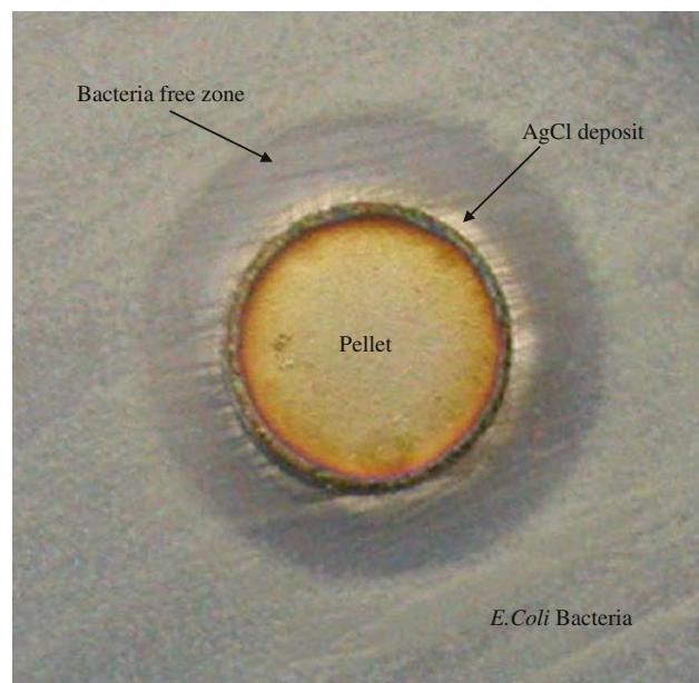
**Fig. 5** Bacteria free zone formation and local AgCl deposition around 29%Ag/TiO<sub>2</sub> made with HNO<sub>3</sub> sol-gel route I
