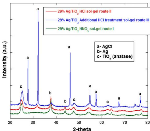
**Fig. 3** XRD patterns of 29% Ag/TiO<sub>2</sub> xerogels prepared with the three preparation routes
