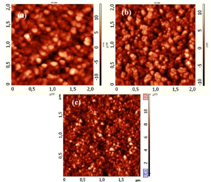
Fig. 2. Surface topography image of bare ITO (a), surface topography image of MPPBA modified ITO (b), and surface topography image of THIBSi modified ITO (c).
