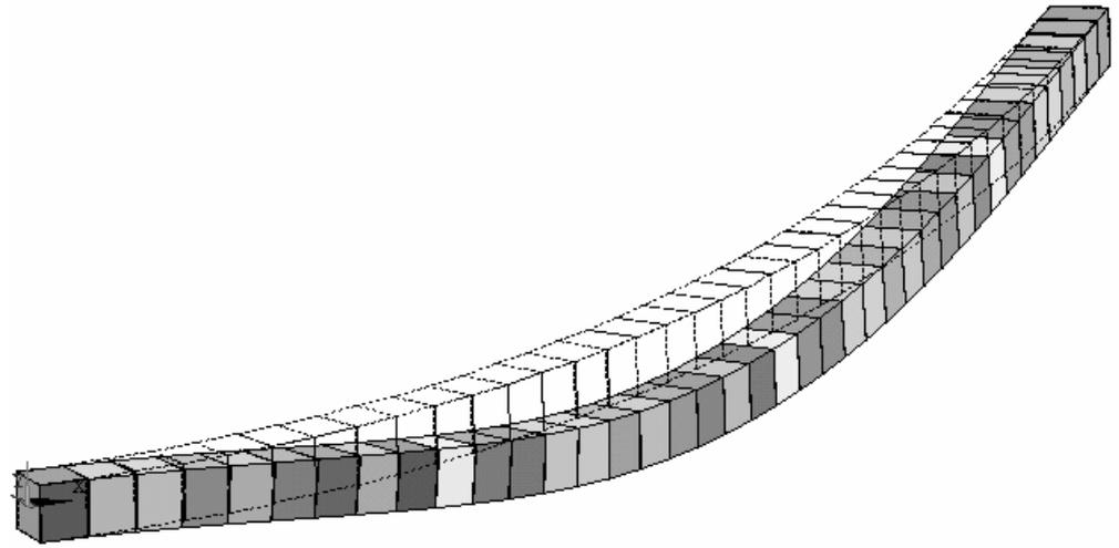
Figure 3.9. Statical displacement of parabolic curved beam due to force at node 16
