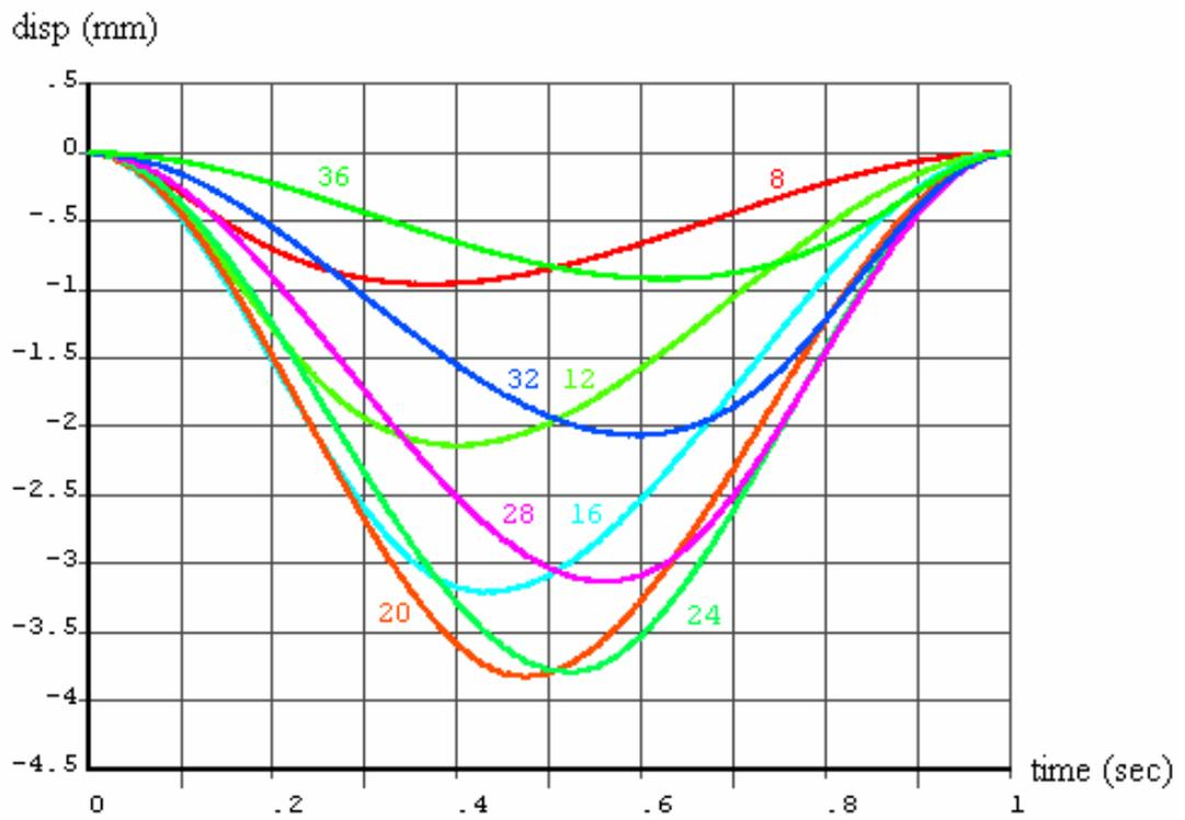
Figure 3.15. Displacements of different nodes for  $v=2080$  mm/s
