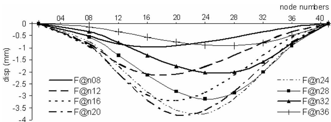
Figure 3.6. Static displacements of parabolic curved beam under several loadings
