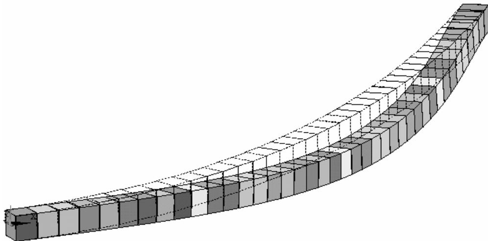
Figure 3.14. Statical displacement of parabolic curved beam due to force at node 36
