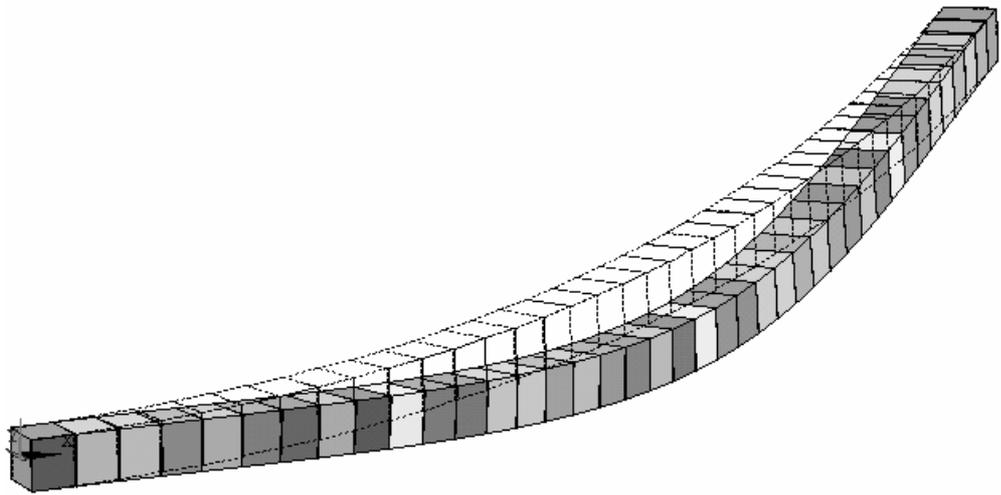
Figure 3.11. Statical displacement of parabolic curved beam due to force at node 24
