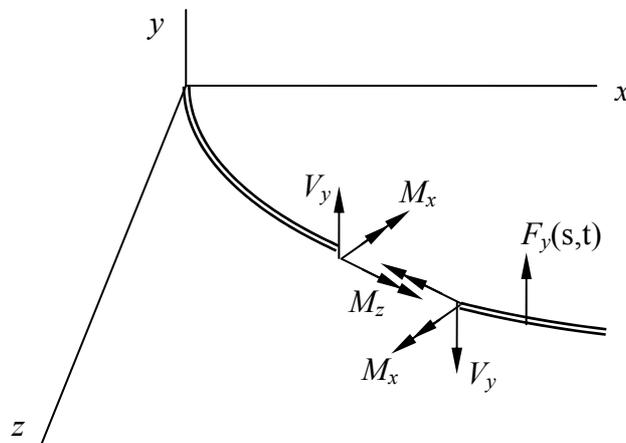
Figure 2.2. Internal reactions and external force of a curved beam
