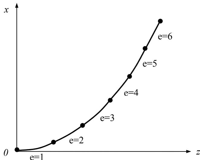
Figure 2.4. Meshing of a curved beam with six finite elements (e≡element).
