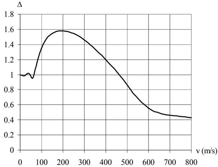
Figure 3.26.  $\Delta$ -v plot for fixed-fixed parabolic curved beam
