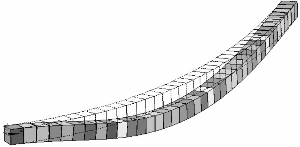
Figure 3.8. Statical displacement of parabolic curved beam due to force at node 12
