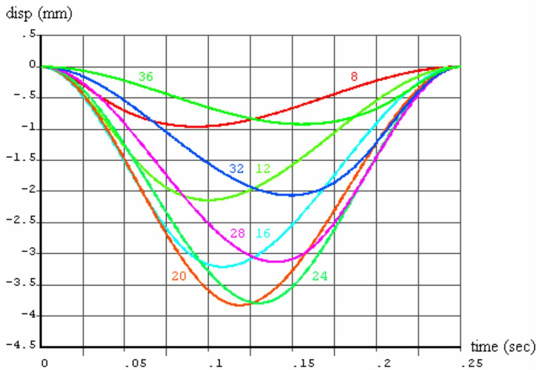
Figure 3.18. Displacements of different nodes for  $v=8320$  mm/s
