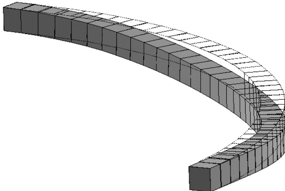
Figure 3.3. First mode shape of a quarter-circular fixed-fixed curved beam
