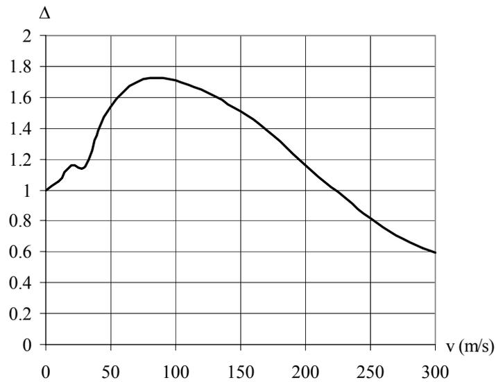
Figure 3.27.  $\Delta$ -v plot for simply supported parabolic curved beam
