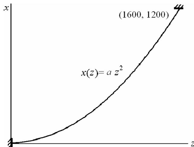
Figure 3.1. Axis of the present non-circular curved beam
