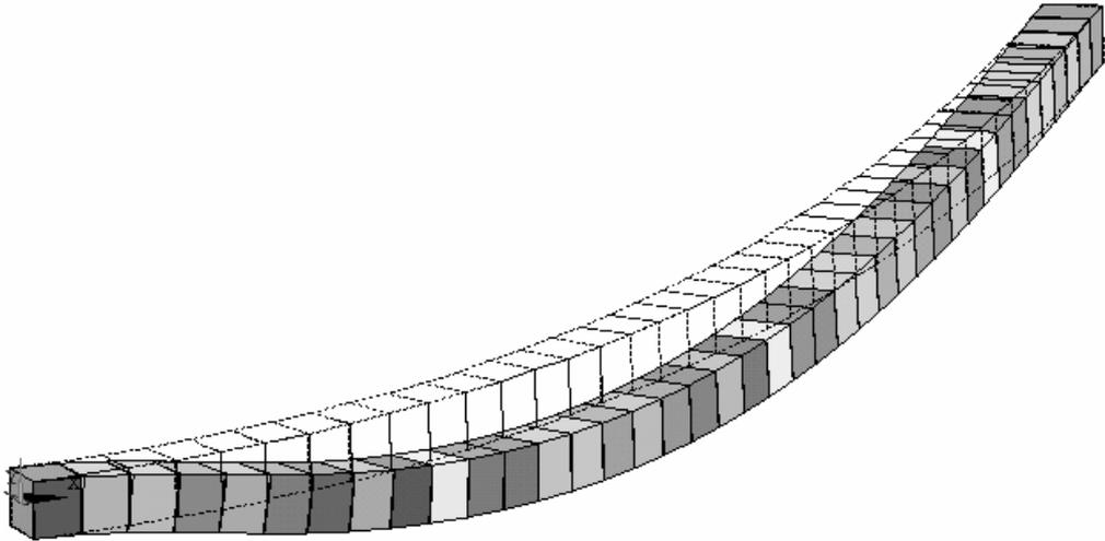
Figure 3.7. Statical displacement of parabolic curved beam due to force at node 8
