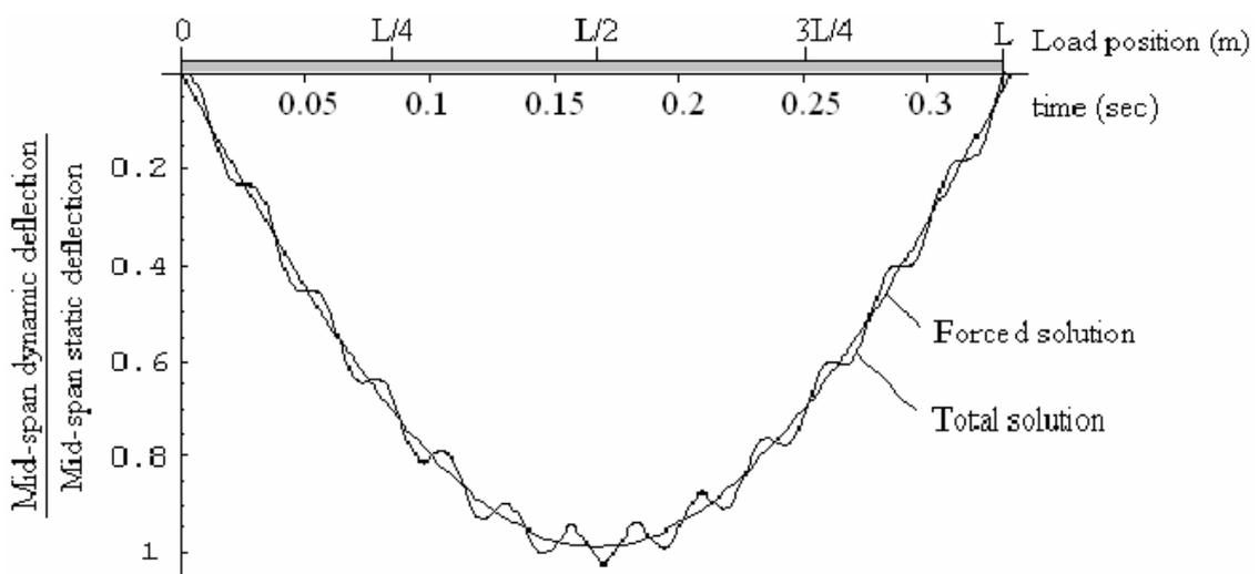
Figure 3.4. Mid-span displacements of simply supported straight beam
