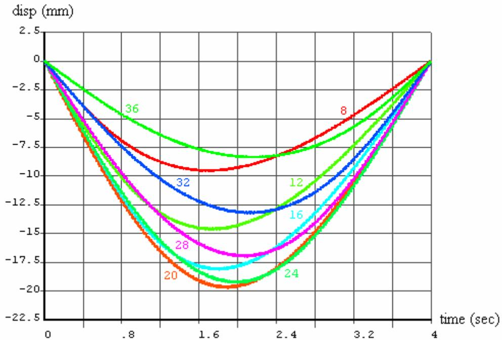
Figure 3.19. Displacements of different nodes for  $v=520$  mm/s
