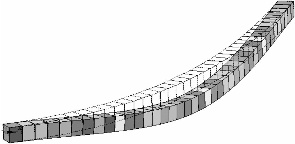
Figure 3.10. Statical displacement of parabolic curved beam due to force at node 20
