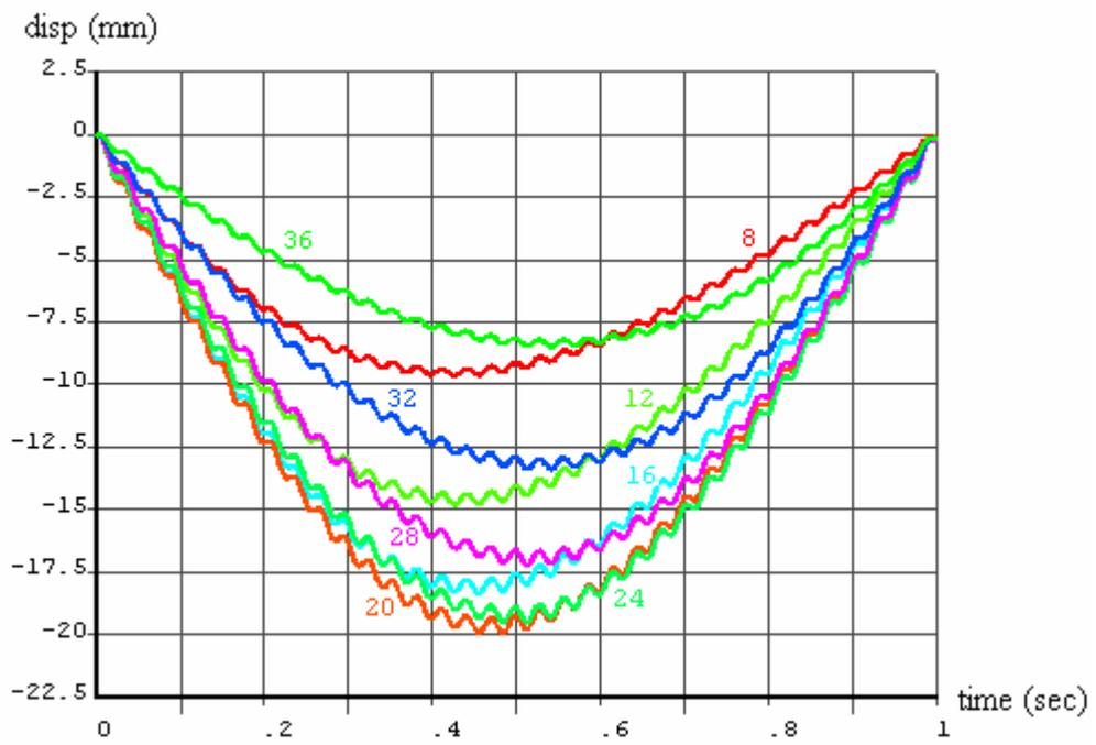
Figure 3.22. Displacements of different nodes for  $v=2080$  mm/s
