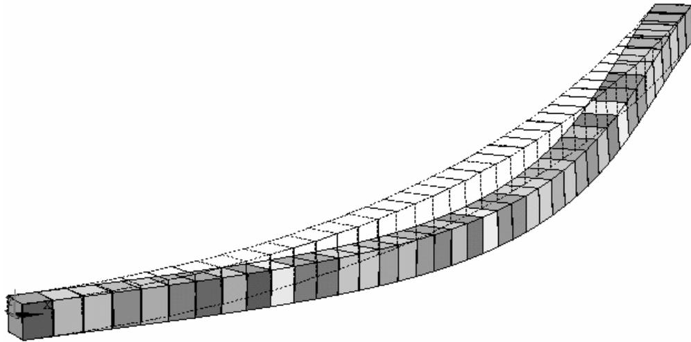
Figure 3.13. Statical displacement of parabolic curved beam due to force at node 32
