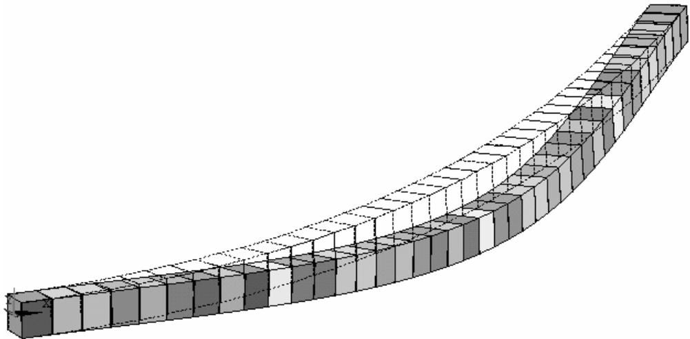
Figure 3.12. Statical displacement of parabolic curved beam due to force at node 28
