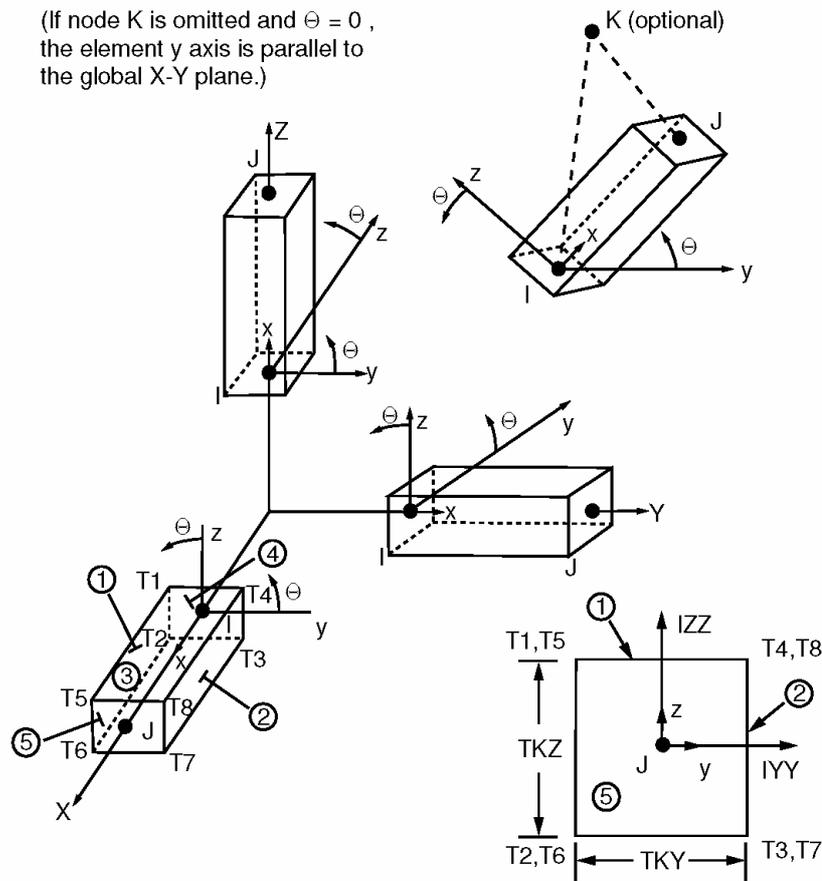
Figure 2.6. Geometry of BEAM4
