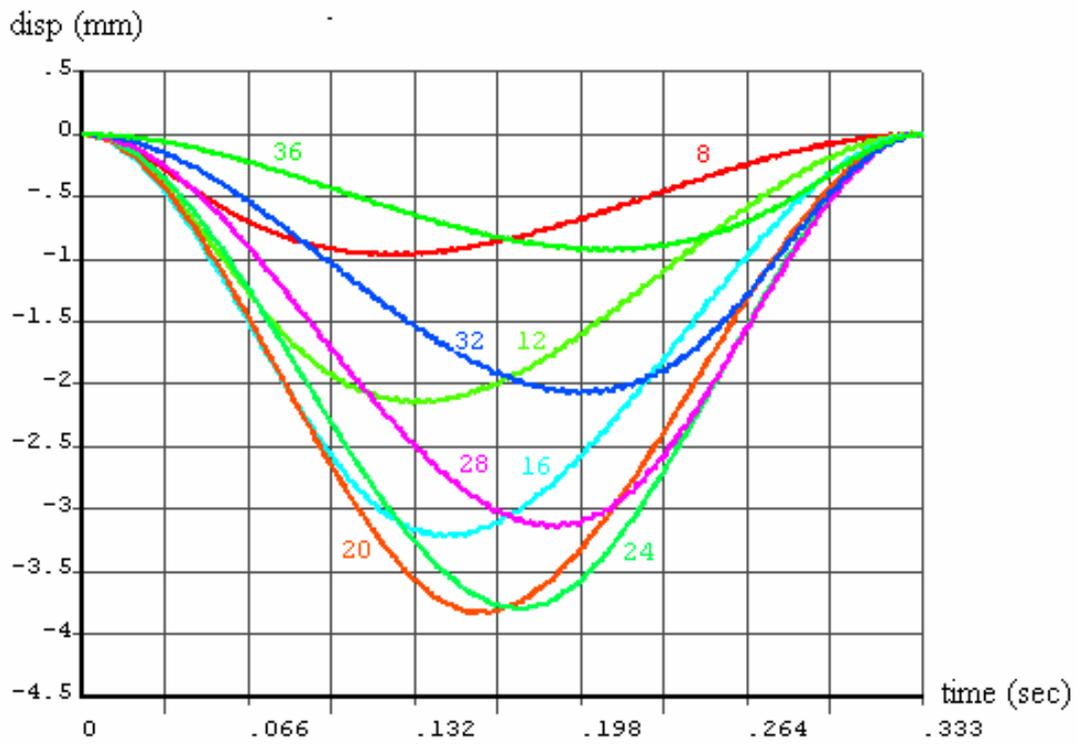
Figure 3.17. Displacements of different nodes for  $v=6240$  mm/s
