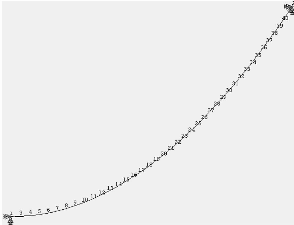
Figure 3.5. Node numbers of parabolic curved beam
