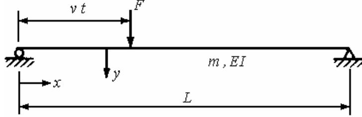
Figure 2.3. A simply supported straight beam under moving load (Source: Biggs, 1964)
