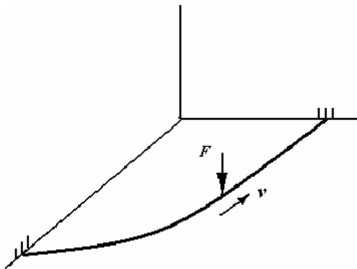
Figure 1.1. A fixed-fixed curved beam under moving load
