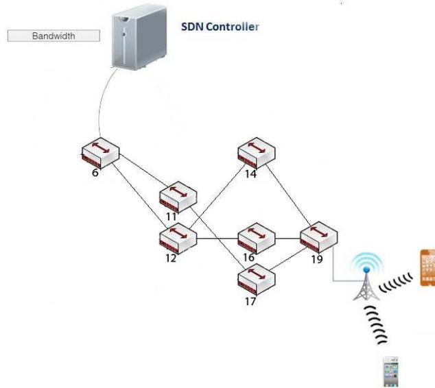
Figure 3.12. Demonstration of the second network with capacity per port of 100 Mbps after proposed routing for 8 flows with throughput requirements of 100 Mbps for the same source and destination nodes.
