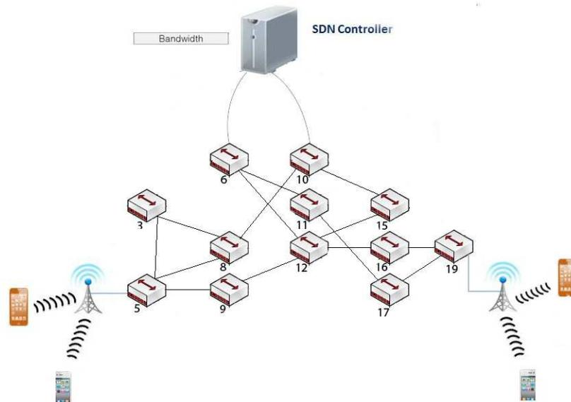
Figure 3.13. Demonstration of the second network with capacity per port of 200 Mbps after proposed routing for 8 flows with throughput requirements of 200 Mbps for the different source and destination nodes.
