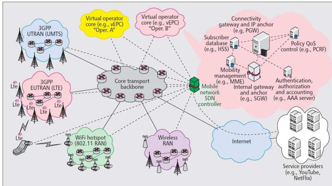
Figure 2.7. SDN-based mobile network architecture [Bernardos2014]
