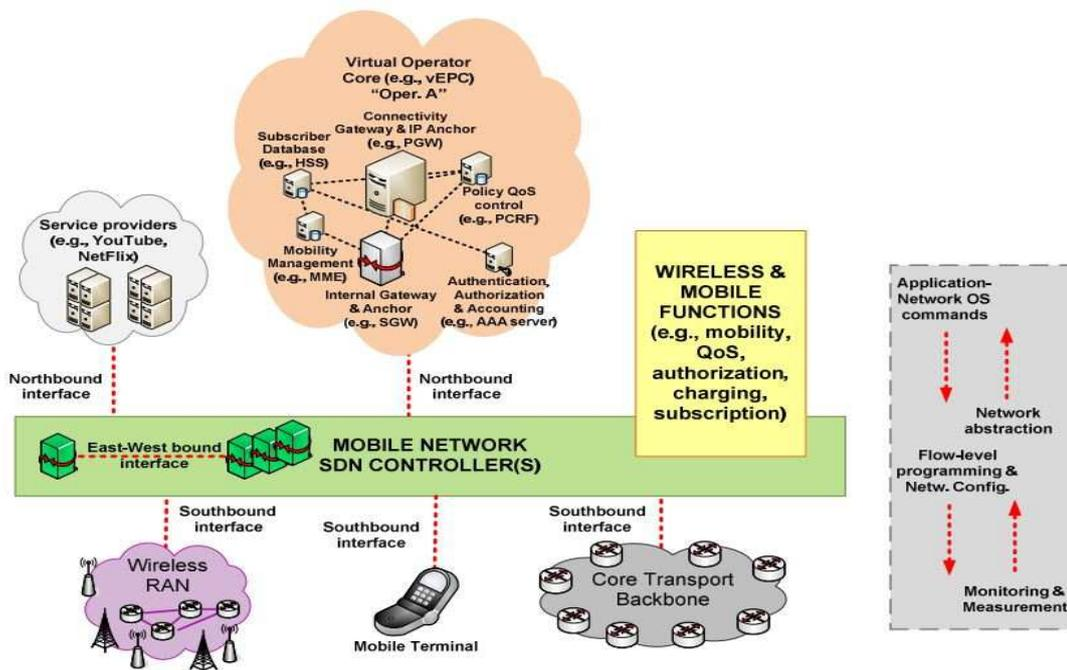
Figure 2.8. SDN-based mobile network interface architecture [Bernardos2014]
