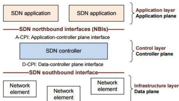
Figure 2.2. SDN components [ONF2014]
