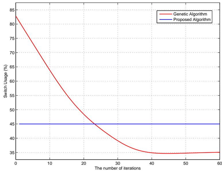
Figure 3.7. Convergence comparison for source node is 1, destination node is 20 and throughput requirement is 100 Mbps
