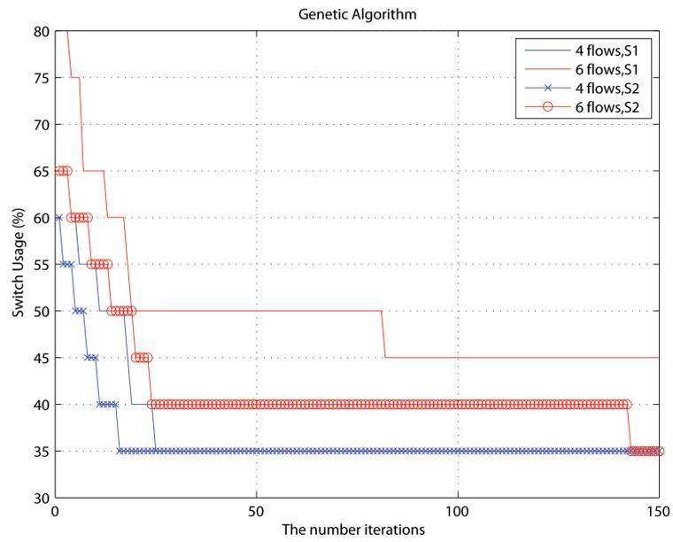
Figure 3.6. The number of required iterations for optimal solution for Scenario 1 and Scenario 2 with throughput requirement of 100 Mbps.
