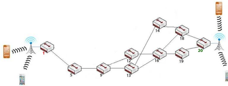
Figure 3.8. Demonstration of network after proposed routing for 8 flows, Scenario 1 with throughput requirement of 100 Mbps.
