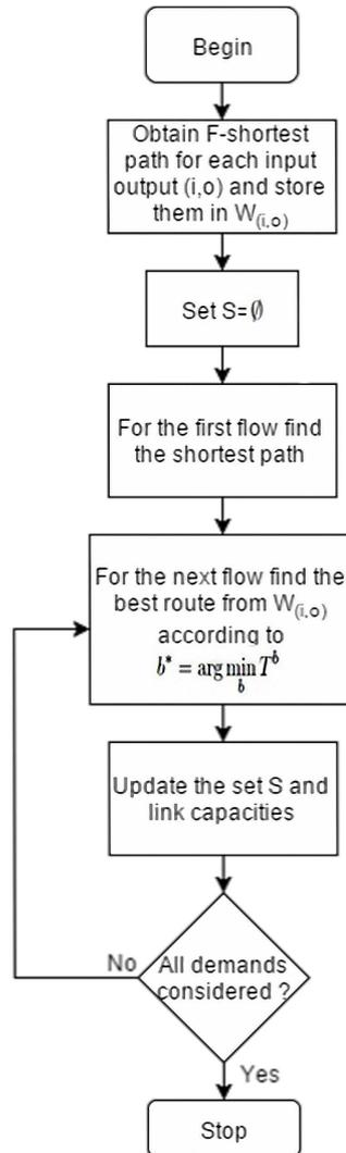
Figure 3.4. The flowchart of proposed routing algorithm
