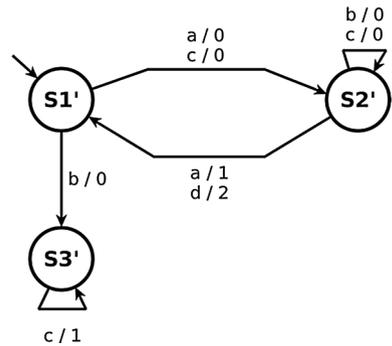
transitions are labeled as *f*-transitions. For the FSM in Fig. 2, a modified FSM with the *f*-transitions is illustrated in Fig. 4.
