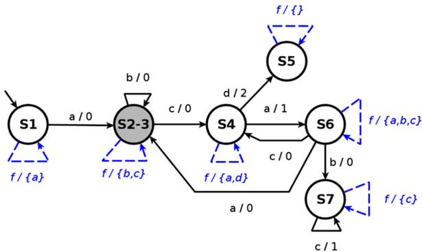
Fig. 5 Reduced FSM with  $f$ -transitions
