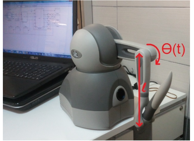
Fig. 2. PHANToM Omni haptic device
