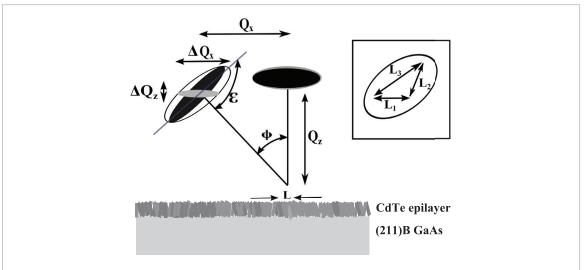
**Figure 4.** Schematics of the lateral coherence length (black ellipse) and domain tilt (grey ellipse). The inset shows  $L_1$ ,  $L_2$  and  $L_3$  vectors according to the general shape of (5 1 1) node of epilayer lattice.
