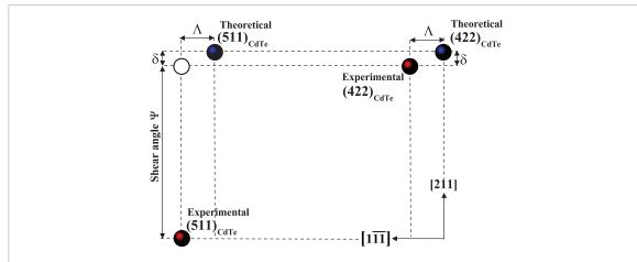
Figure 3.  $\Lambda$  and  $\delta$  parameters due to the lattice tilting, as well as the shear angle  $\Psi$  produced by the low-symmetry surface, are shown in the scaled figure. Open circle was drawn based on the assumption that the tilting trend of the (4 2 2) node is valid for theoretical position of the (5 1 1) node.
