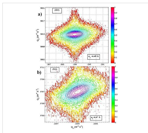
**Figure 1.** (a) The (4 2 2) and (b) the (5 1 1) nodes of CdTe epilayer. Elongation of these RLPs can be indication of the formation of a mosaic layer structure. The calculated lattice parameters ( $a_{\perp}$  and  $a_{\parallel}$ ) are also seen in their insets, with measurements in angstroms (Å).
