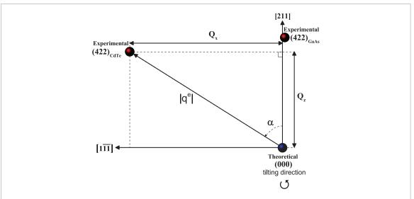
**Figure 2.** The experimental positions (red) of the (4 2 2) RLPs of CdTe epilayer and GaAs substrate without taking widths of the peaks into account. The scattering vector length of the epilayer ( $|\mathbf{q}^e|$ ) and the tilting angle ( $\alpha$ ) according to the theoretical origin (blue) are also illustrated.
