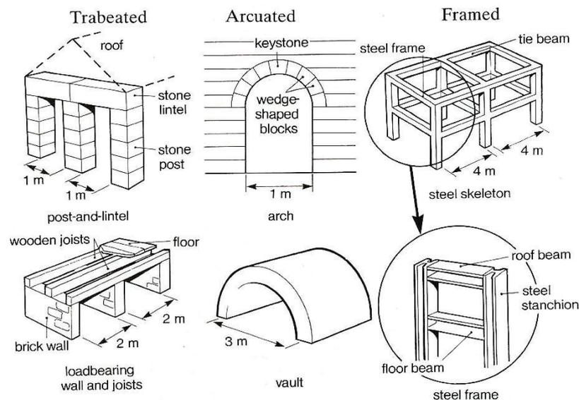
Figure 2.2. Structural system examples
