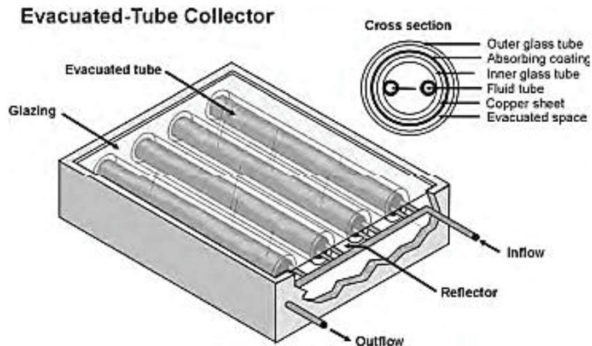
Figure 3.13. Evacuated tube solar collector
