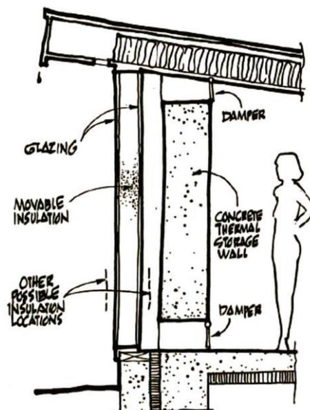
Figure 3.5. Trombe wall system principle
