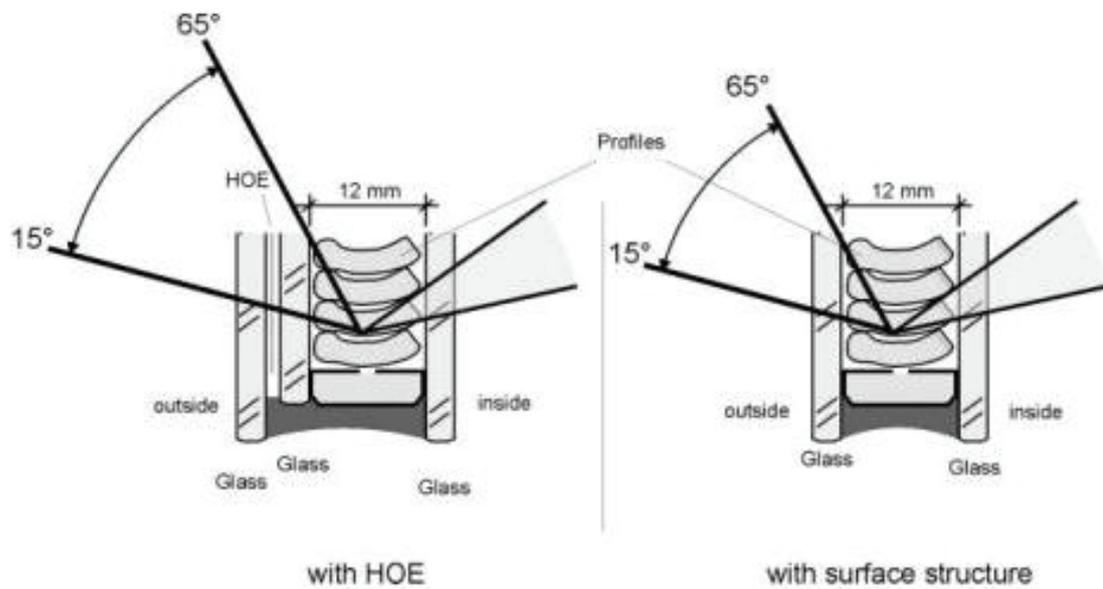
Figure 3.23. Vertical deflection of sun directing glass (HOE: Holographic optical elements) (IEA, 2000; Koster, 2004; Reinhart, 2014)
