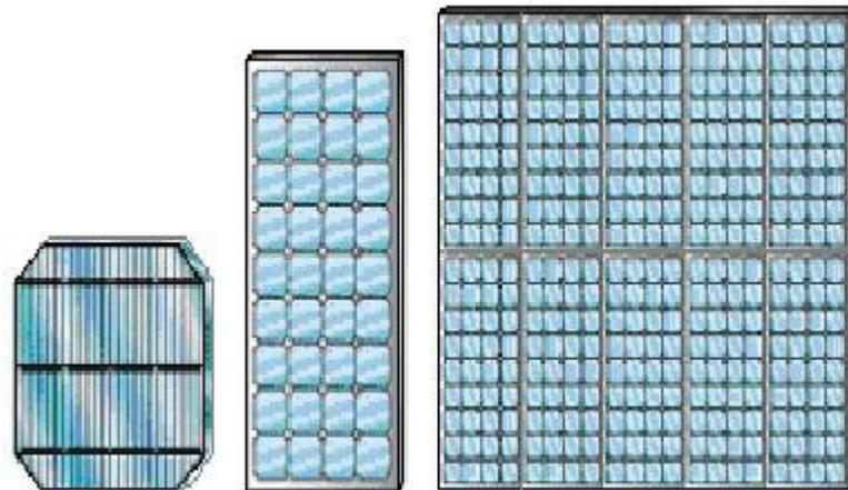
Figure 3.19. A photovoltaic cell, photovoltaic module and photovoltaic panel
