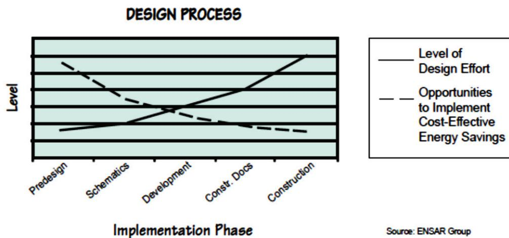
Figure 3.1. Relation between design process and integration (Smith, 2010)
