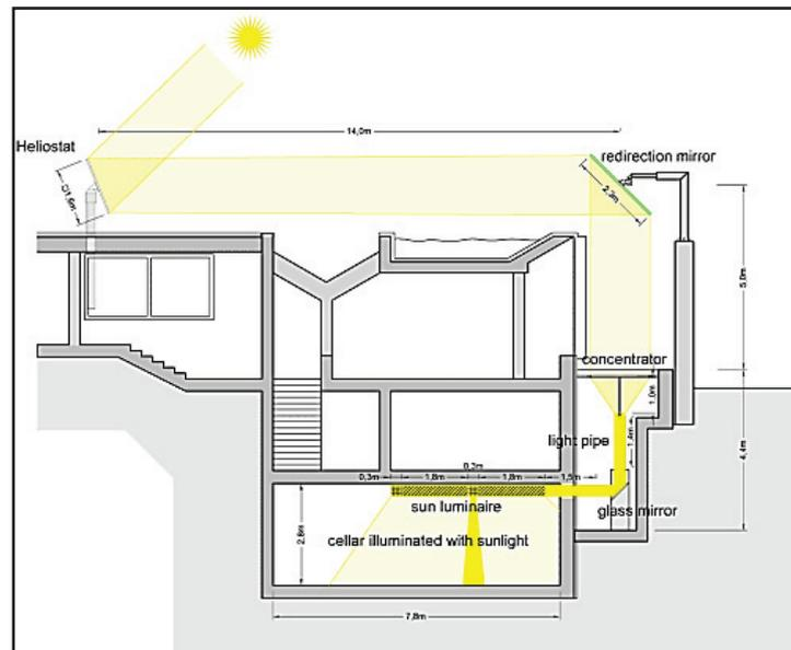
Figure 3.28. Scheme of heliostat daylighting system
