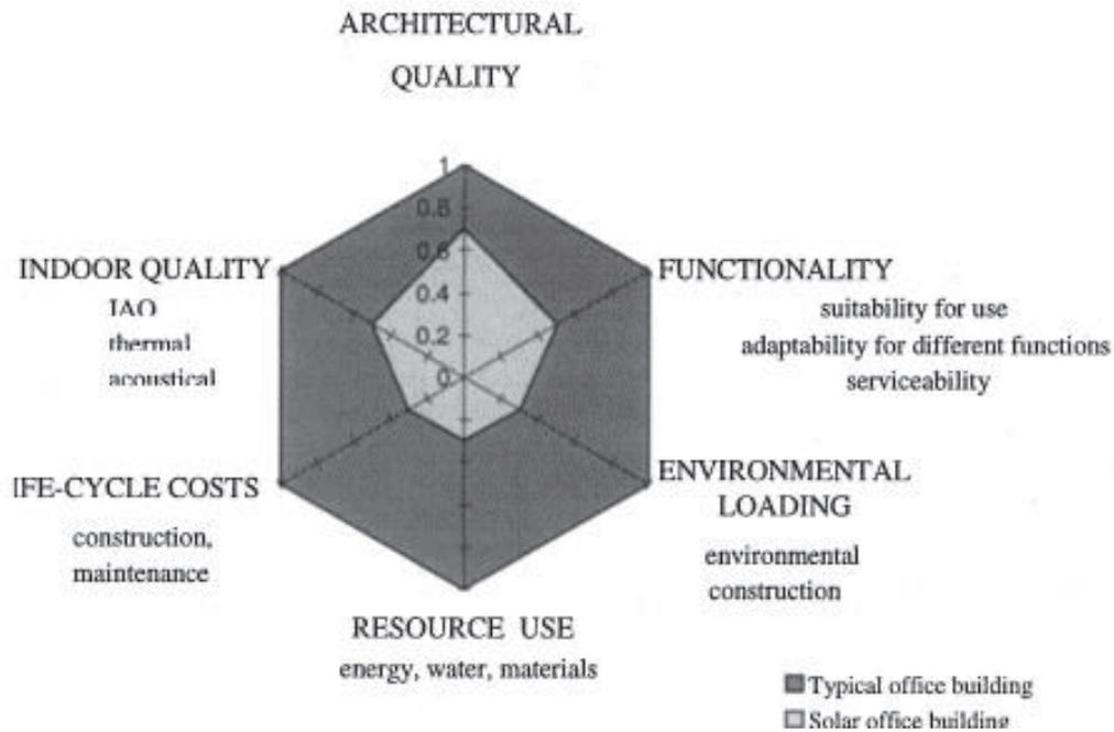
Figure 3.3. An example of a footprint of a solar office building and typical office building (Hestnes, 1999)
