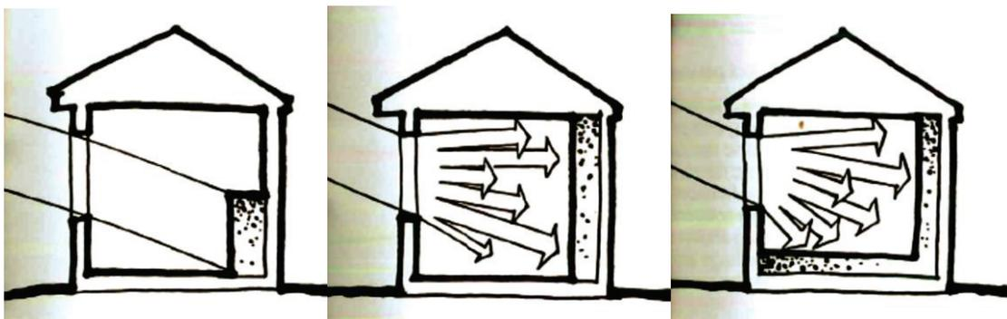
Figure 3.4. Solar heat gain from solar windows
