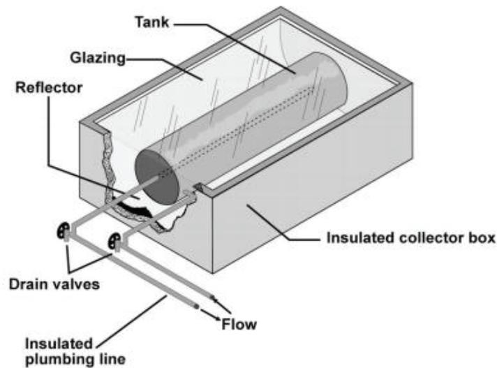
Figure 3.14. Batch solar collector
