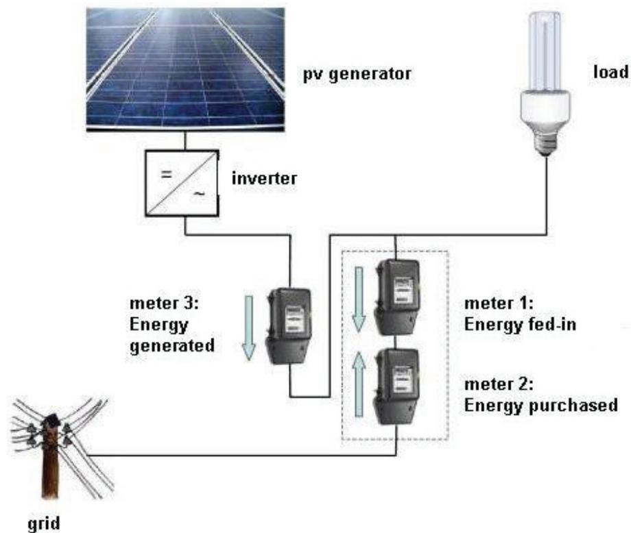
Figure 5.8. Diagram of a grid-connected PV system
