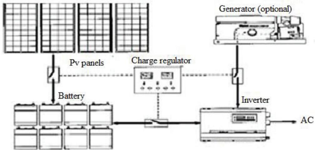
Figure 3.18. PV systems working principle
