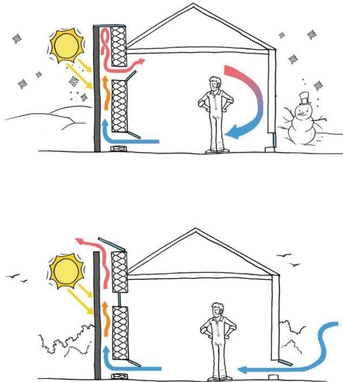
Figure 3.11. Solar chimney system principal for heating and cooling
