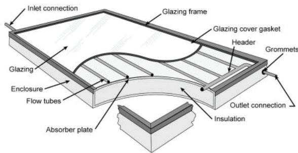
Figure 3.12. Flat plate solar collector
