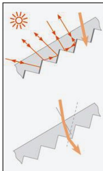
Figure 4.2. Static prismatic systems
