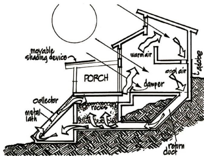
Figure 3.10. Thermosyphon system
