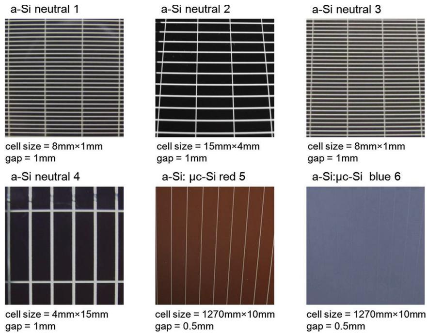
Figure 5.6. PV modules in various types
