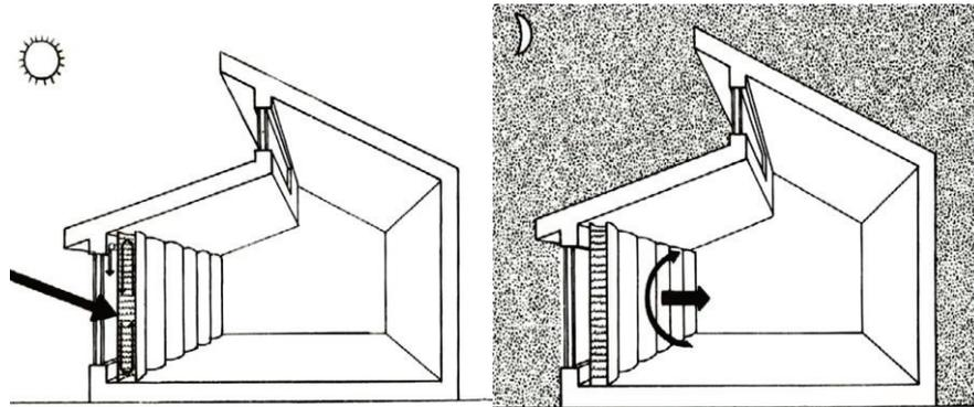
Figure 3.6. Water wall system principal, daytime and nighttime
