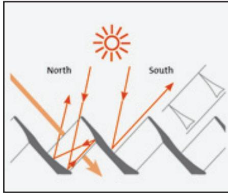
Figure 4.3. Micro-sun shielding louvers
