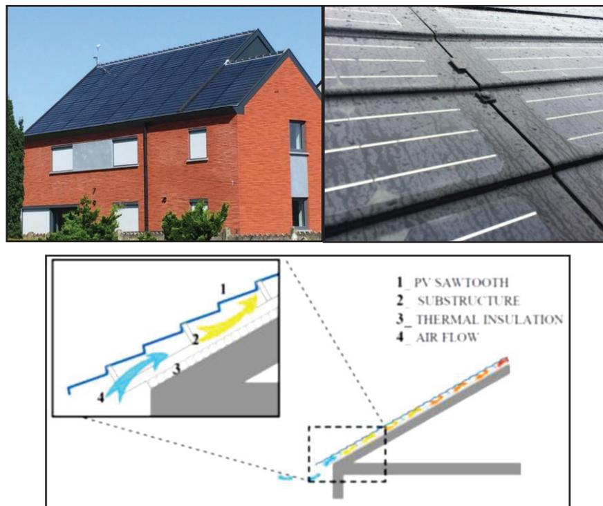
Figure 5.1. The roof structure indicating the way of the air flow behind the PV panels(Agathokleous, Kalogirou, & Karellas, 2017).
