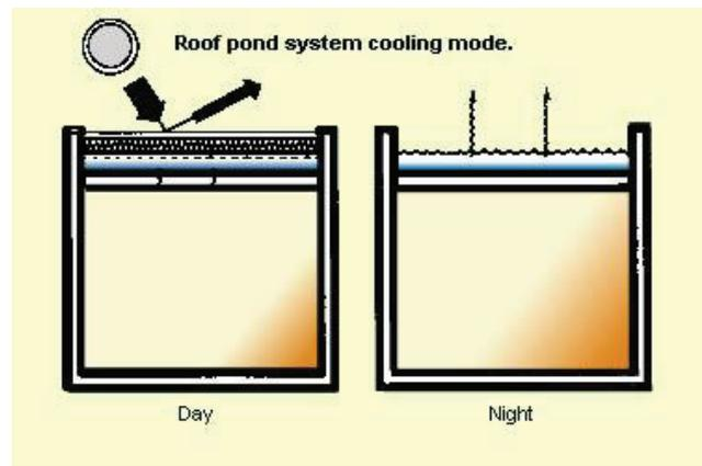
Figure 3.8. Roof pond system principal in summer (Al-Jamal et al., 1988)
