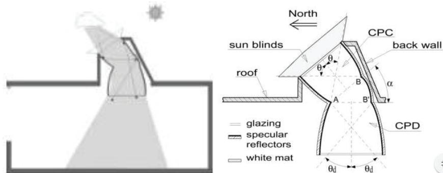
Figure 3.27. Anidolic zenith openings scheme and cross-section
