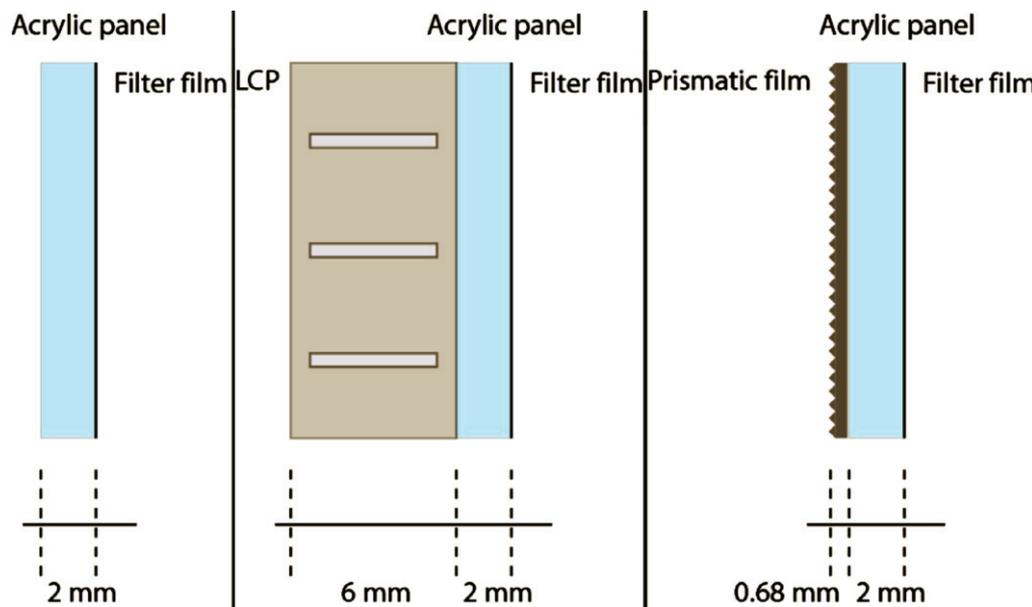
Figure 5.5. Attachment types of CFS and their appearance on the fenestration (Thanachareonkit & Scartezzini, 2010)
