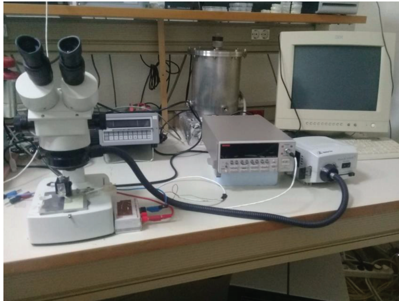
Figure 4.12. I-V experimental setup interfaced with a computer.
