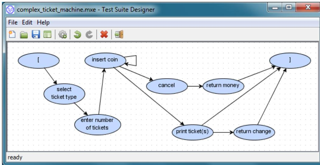
Figure 22. ESG for complex ticket machine [96]
