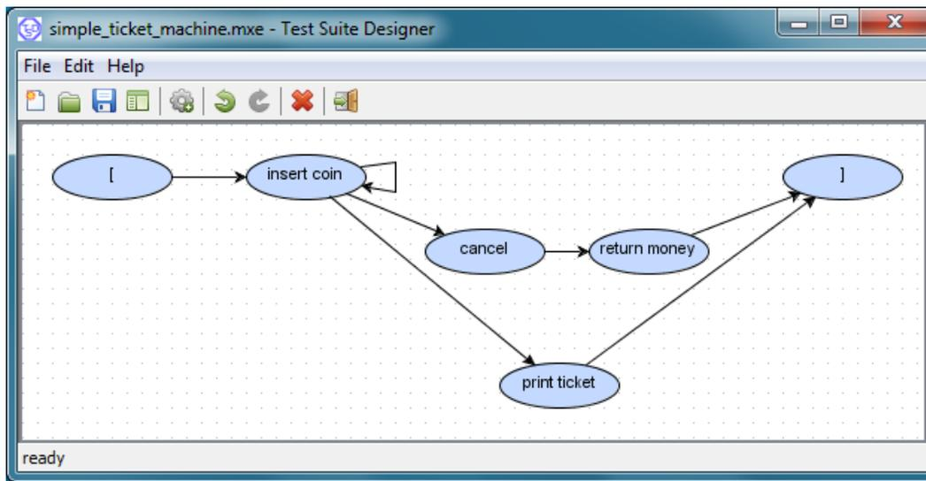
Figure 20. ESG for simple ticket machine in ESG-TSD [96]
