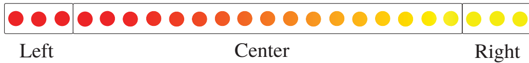
Figure 1.4. An example of a partitioned one-dimensional model for heat transport under a temperature gradient. The temperature gradient is shown by a color gradient from hot reservoir (Left region) to cold reservoir (Right region) through the device (Center region)
