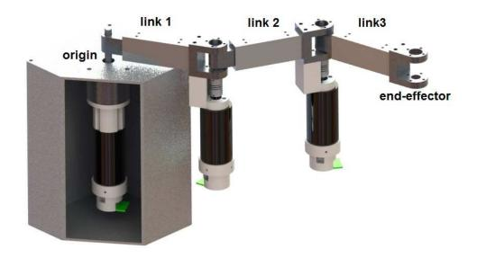
Figure 2.8. The 3 degree of freedom planar robot manipulator
