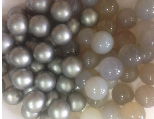
Figure 3.6. Agate milling balls covered by Al powder and cleaned with NaOH solution.
