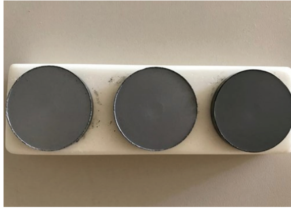
Figure 3.11. The pressed samples with a diameter of 30 mm.
