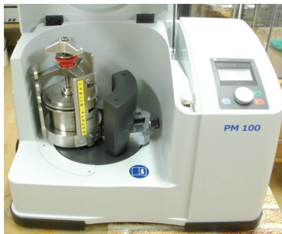
Figure 3.7. The planetary ball mill utilized in the study.
