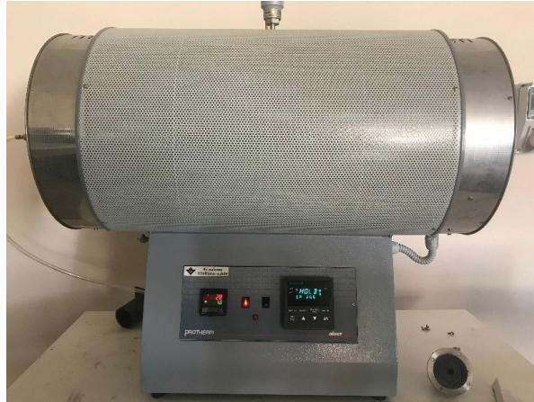
Figure 3.12. Tube sintering furnace used in the sintering process.
