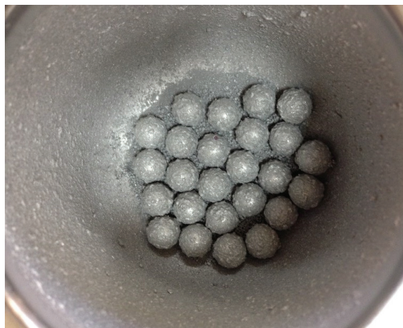
Figure 3.5. Contamination of milling tools by the cold-welded Al particles during milling in the absence of any PCA.
