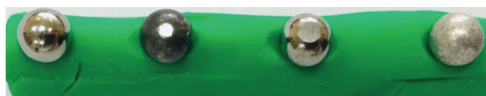
Figure 4.31. Hardened steel balls used for ball-on disc dry sliding wear test.
