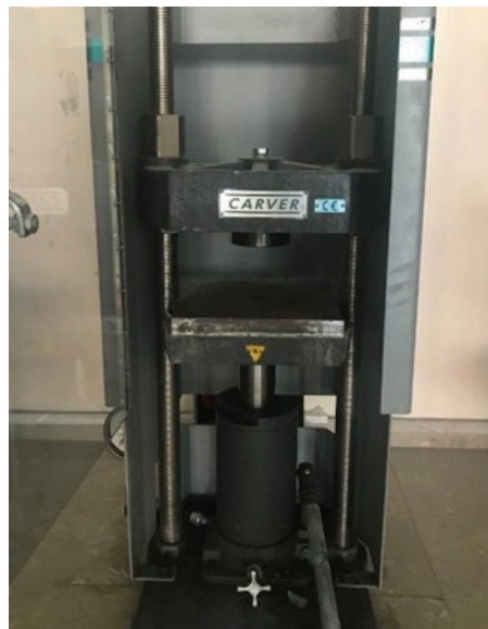
Figure 3.10. Carver hydraulic unit model uniaxial press.
