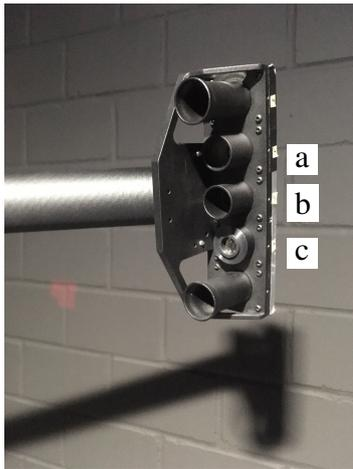
Figure 2.8: Si (a), Si photometric (b), and InGaAs (c) detectors employed in this research. The outer two positions are unused and available for future extensions.
