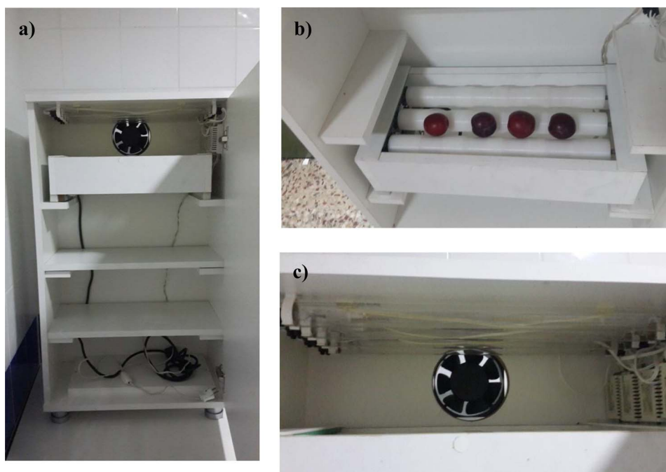
Fig. 1. Bench top UV-C system a) Tray system b) Rotating roller bearing c) UV lamps and a cooling fan.
