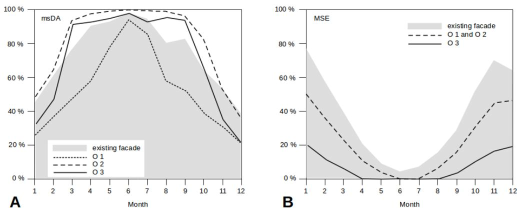
FIG. 6 Monthly daylight metrics msDA (A) and MSE (B) for the optimization variants compared to the existing facade.
