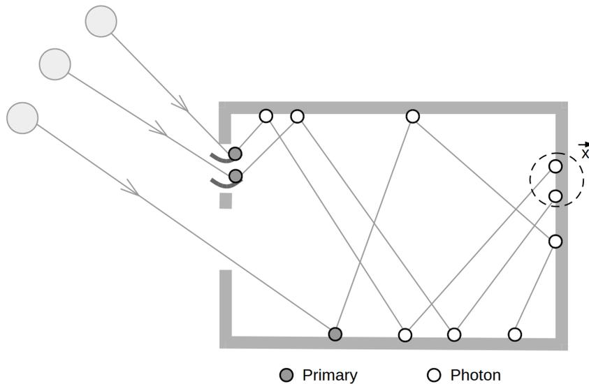
FIG. 3 Contribution Photon Mapping: Photons emitted from the light sources are deposited as primary photons upon their first hit in the scene and referenced by each spawned photon. During gathering at point  $\vec{x}$ , this reference is used to sort the photons according to the emitting light source.
