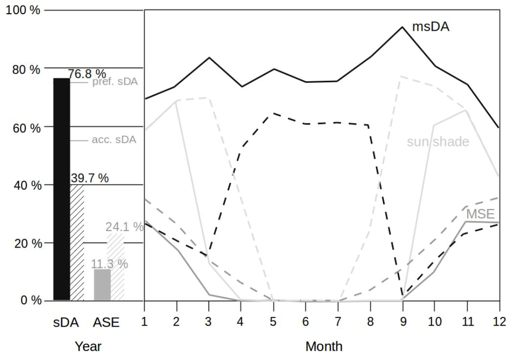
FIG. 8 Daylight metrics for the classroom scene with DRC (filled bars /solid lines) and the reference room without DRC (hatched bars /dashed lines)
