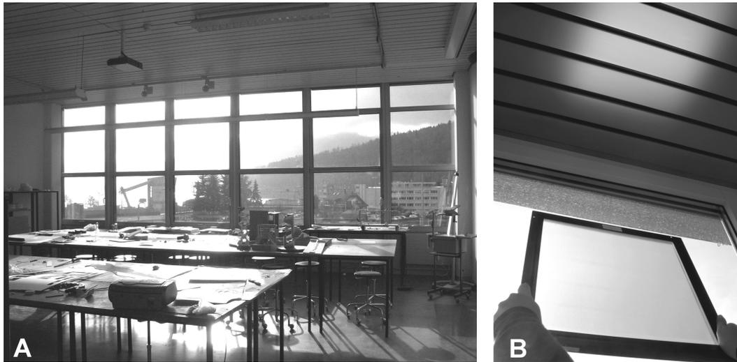
FIG. 4 Room with south facing facade (A) and DRC sample made from light redirecting prismatic film (B)
