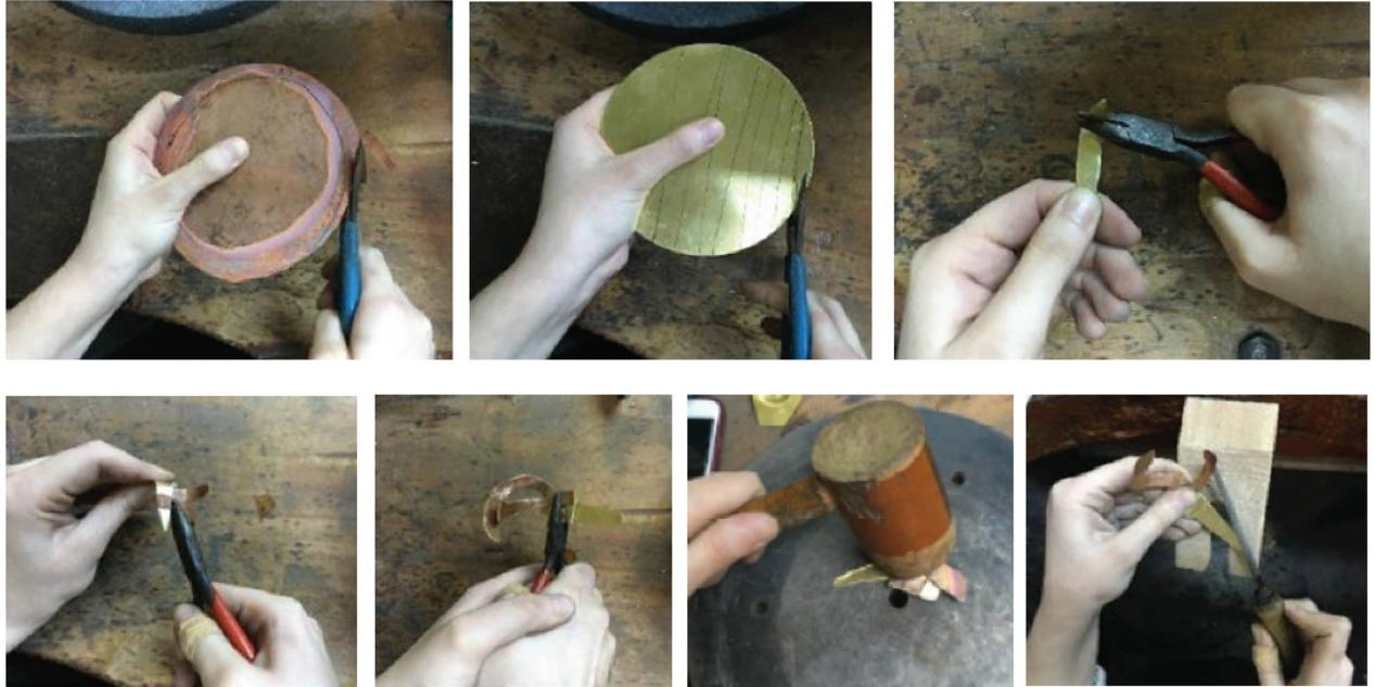
Figure 6: Production process of Anomali by Alara Altmören: 1st row: cutting brass and copper 2nd row: bending, hammering, wrapping and rasping brass and copper. From the Apprenticeship in Product Design: Kapalıçarşı design course archive. © Alara Altmören.
