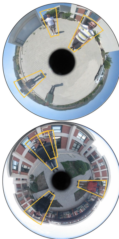
Fig. 10 Example instances where our RICF method fails. Top: false negative example. Bottom: false positive example
