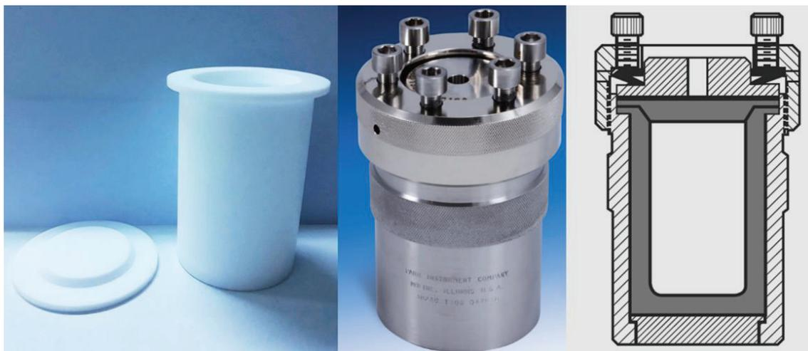
Figure 3.1. The photographs of the used PTFE Teflon, the photograph and schematics of the autoclave<sup>93</sup> from left to the right respectively.
