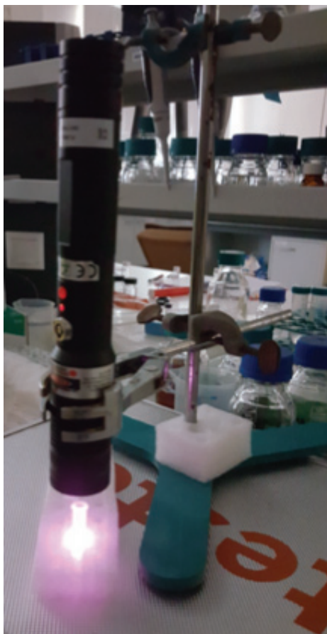
Figure 3.2. Experimental setup for photothermal effect measurements of nanostructures.
