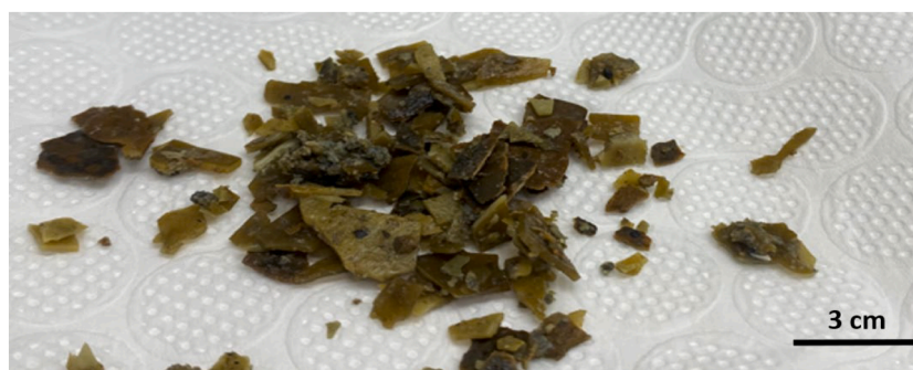
Fig. 12. Precipitation materials collected from inside of 6 5/8-inch casing.
